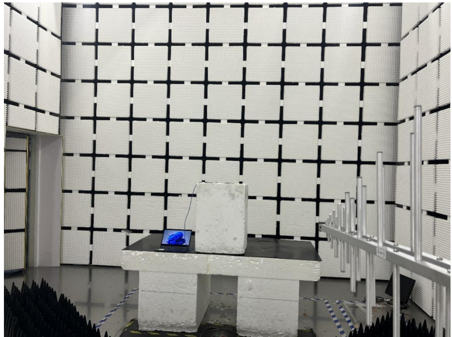
Radiation Emission Test Setup (30MHz to 1GHz)
