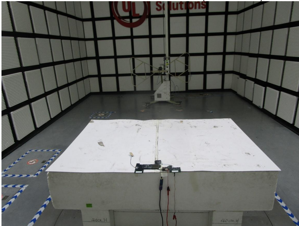
RADIATED RF MEASUREMENT SETUP (Below 30MHz)
