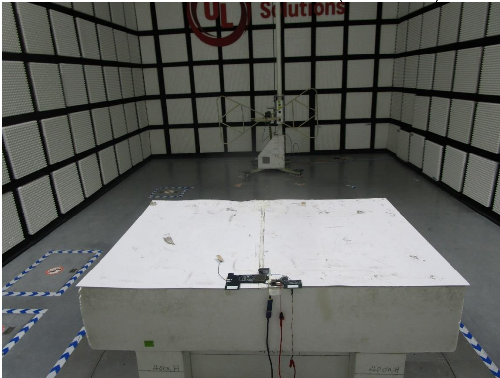
RADIATED RF MEASUREMENT SETUP (Below 30MHz)
