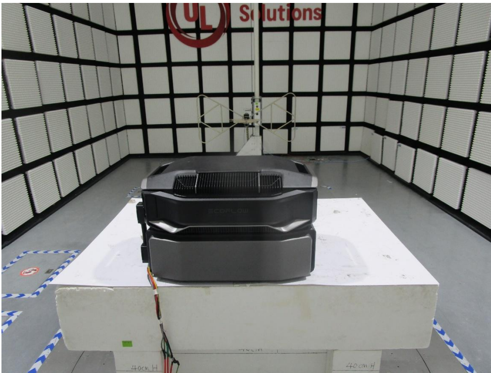
RADIATED RF MEASUREMENT SETUP (30MHz~1GHz)
