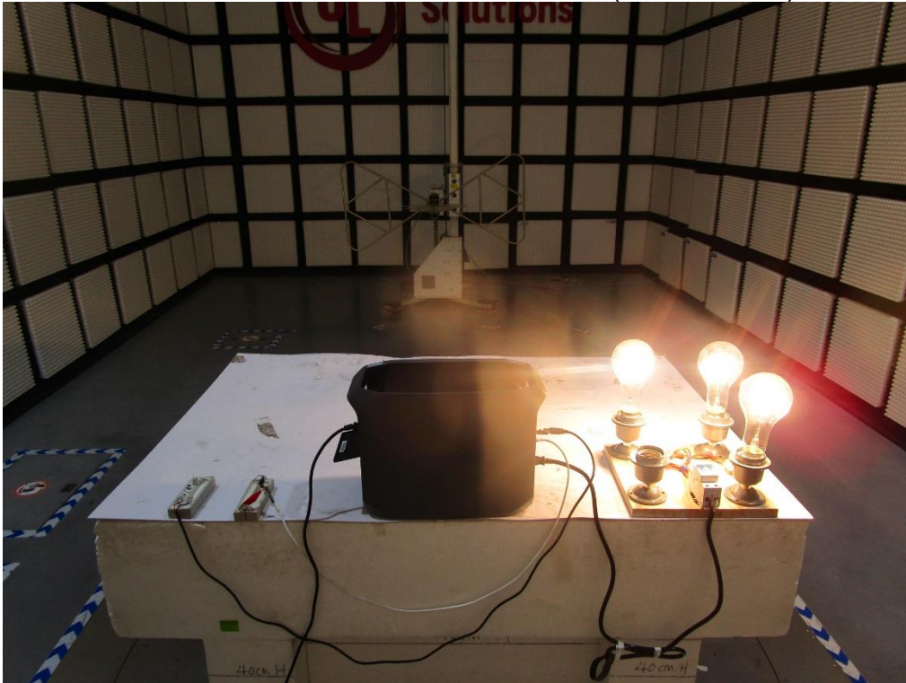
RADIATED RF MEASUREMENT SETUP (Below 30MHz)
