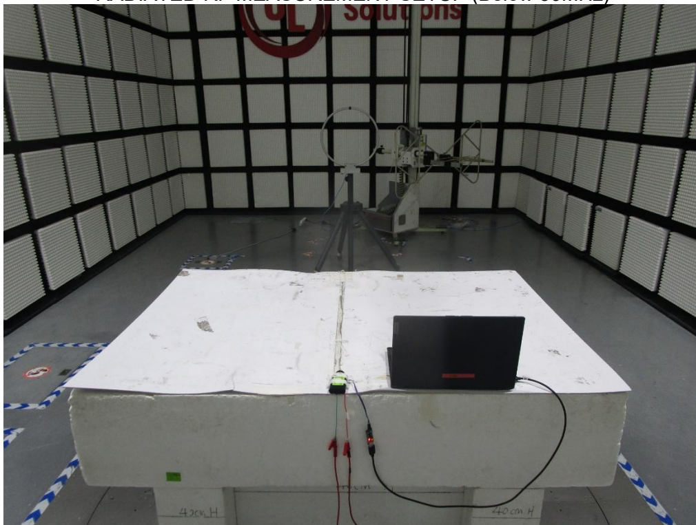
RADIATED RF MEASUREMENT SETUP (Below 30MHz)
