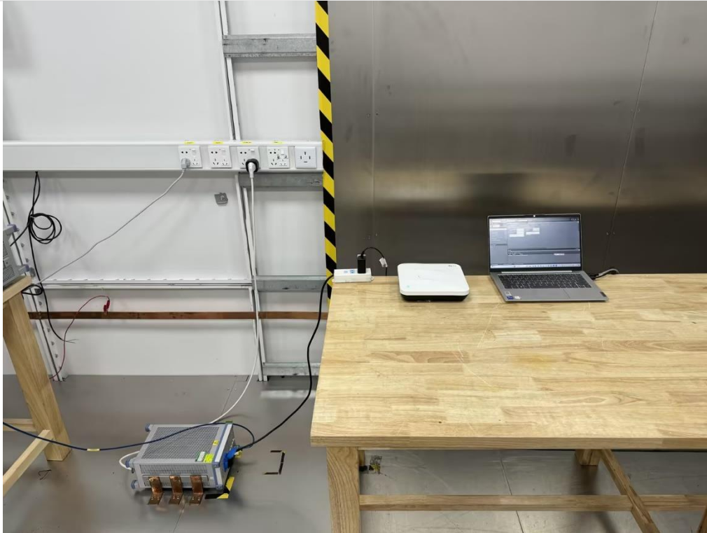
AC Power Line Conducted Emission
