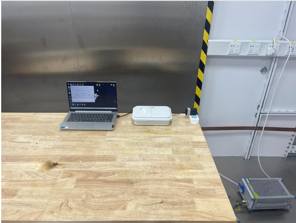
AC Power Line Conducted Emission
