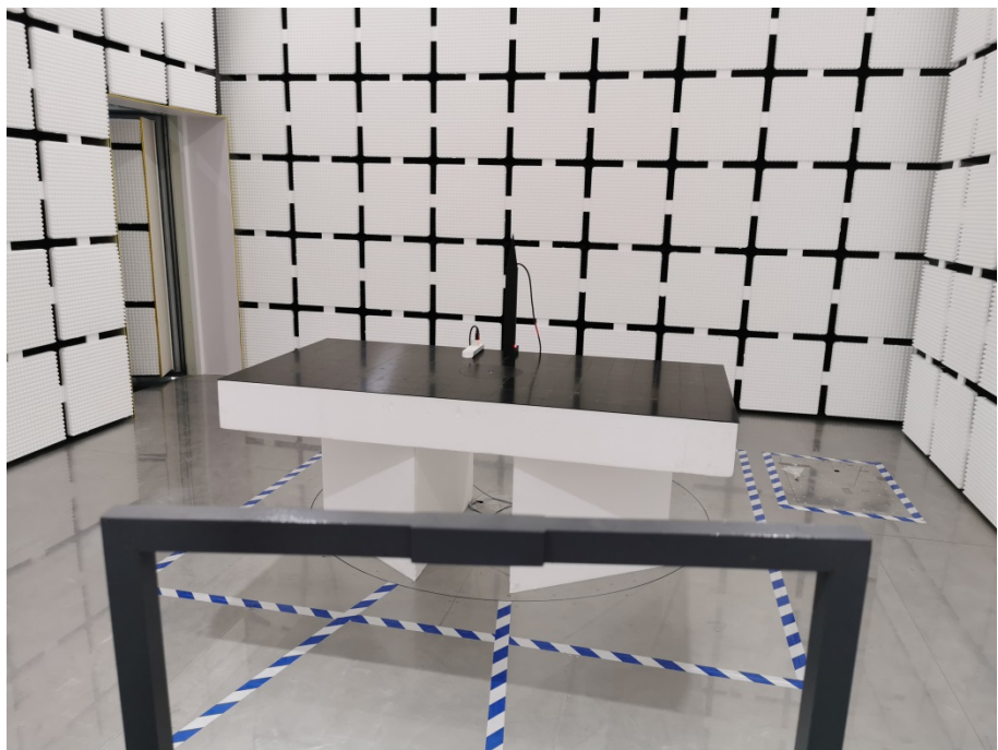
Radiation Emission Test Setup (Below 30MHz)
