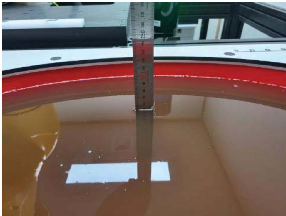
600 MHz ~ 10 GHz Head Broad band Tissue Simulating Liquid, Depth: 150 mm
