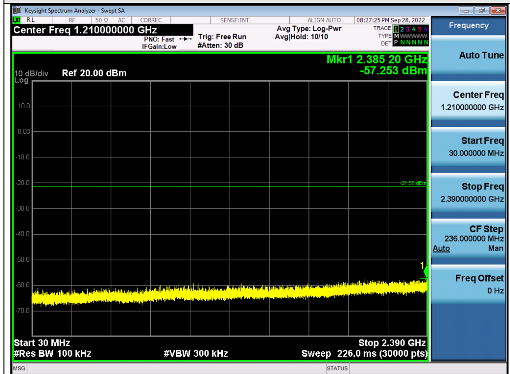
Test_Graph_EDR_ANT1_2402_3Mbps_Lower Band Emissions
