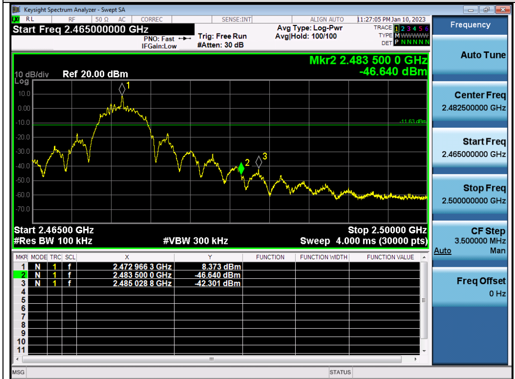
Test_Graph_2.4G_ANT1_2473_4Mbps_Higher Band Edge Emissions
