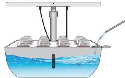
8. Add fresh water into the water tank to the water level of 6.5L, keep the water level gently touching the bottom of planting cotton, and do not add excessive water.
