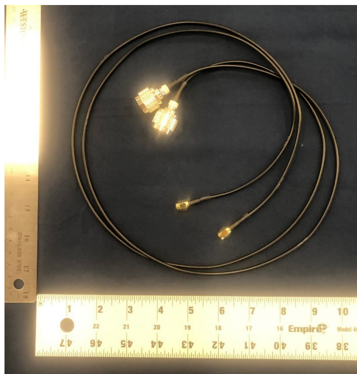
5 GHz Flat Panel Antenna Cables
