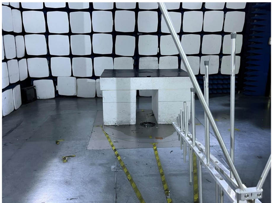
Radiation Emission Test Setup (30MHz to 1GHz)
