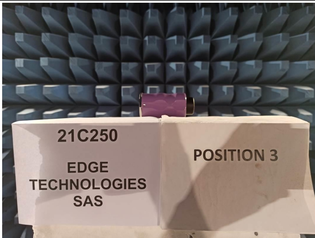
TEST SETUP PHOTO(S) - EQUIVALENT ISOTROPIC RADIATED POWER / POSITION 3
