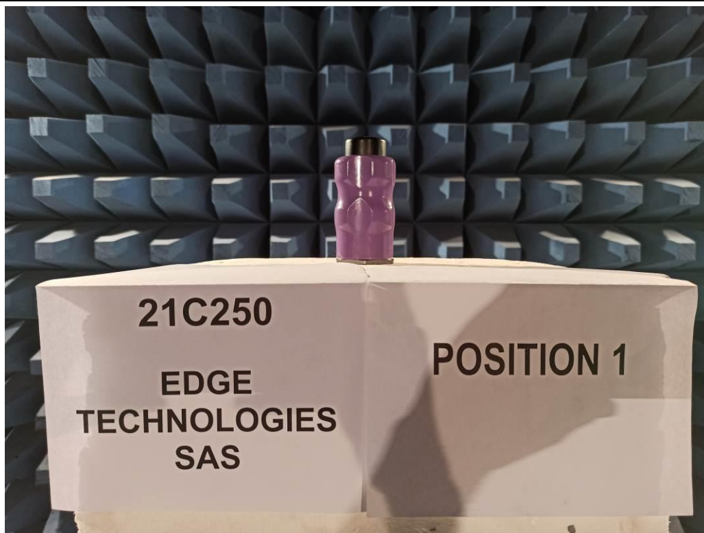
TEST SETUP PHOTO(S) - EQUIVALENT ISOTROPIC RADIATED POWER / POSITION 1
