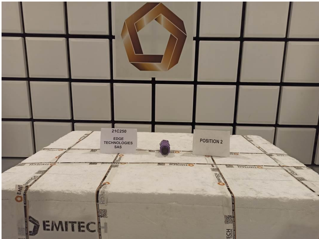
TEST SETUP PHOTO(S) – RADIATED EMISSION LIMITS – POSITION 2
