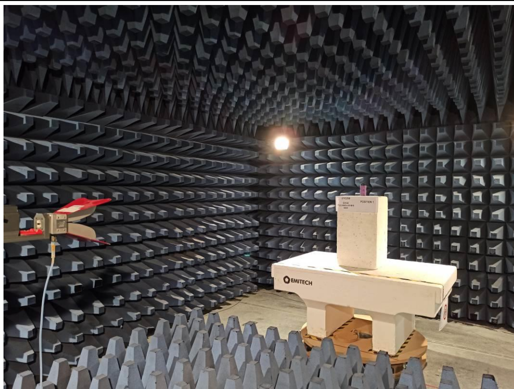
TEST SETUP PHOTO(S) - EQUIVALENT ISOTROPIC RADIATED POWER
