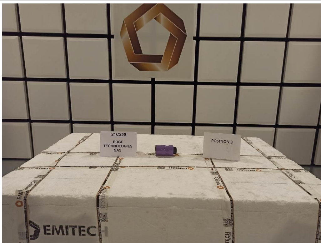
TEST SETUP PHOTO(S) – RADIATED EMISSION LIMITS – POSITION 3
