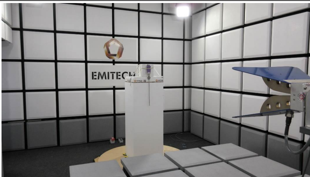
TEST SETUP PHOTO(S) - RADIATED MEASUREMENT / 1 GHz TO 18 GHz
