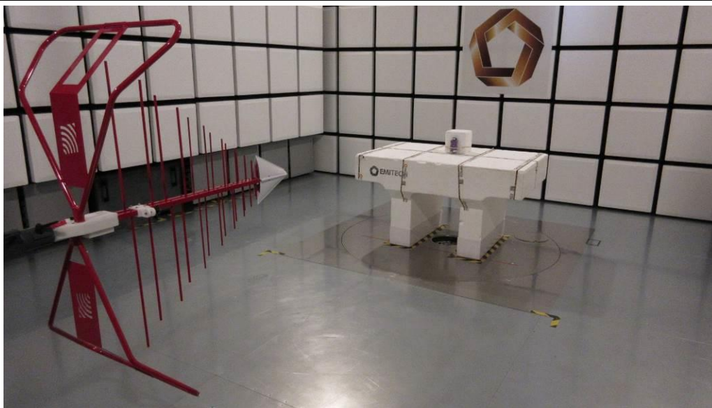
TEST SETUP PHOTO(S) - RADIATED MEASUREMENT / 30 MHz TO 1 GHz
