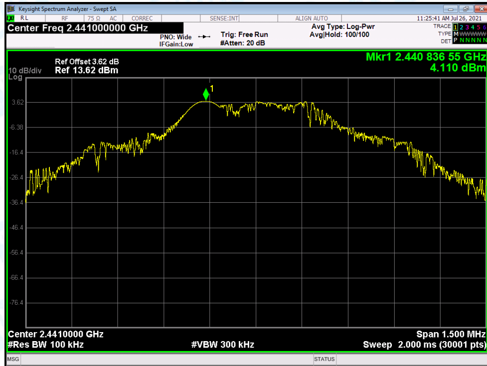
Tx. Spurious NVNT 1-DH1 2441MHz Ant1 Emission
