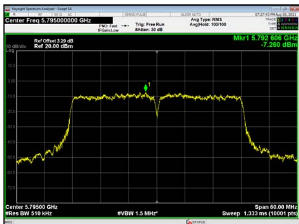
(802.11n40) PSD plot on channel 159
