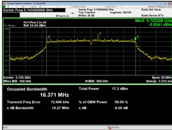
(802.11a) 99%Bandwidth plot on channel 149
