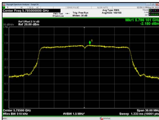
(802.11n20) PSD plot on channel 165
