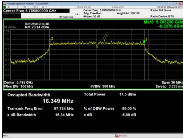
(802.11a) 99%Bandwidth plot on channel 157
