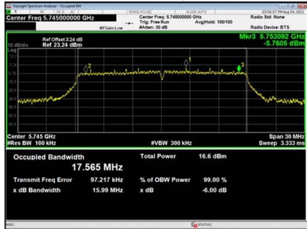
(802.11 n20) 99%Bandwidth plot on channel 149
