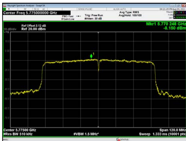
(802.11ac80) PSD plot on channel 155
