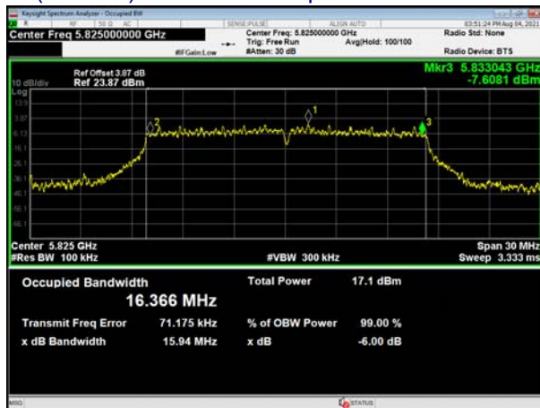
(802.11a) 99%Bandwidth plot on channel 165
