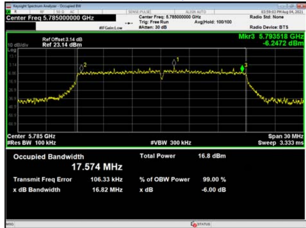
(802.11 n20) 99%Bandwidth plot on channel 157
