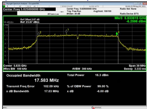
(802.11 n20) 99%Bandwidth plot on channel 165
