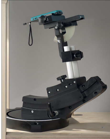
F-2. Device Holder for Transmitters
