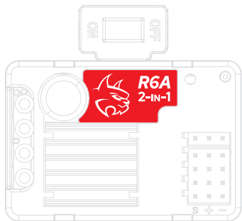
B-TRCRR6AESC-01 RCR-R6A-ESC正面贴 0.175磨砂PC+3M9448A胶 18.30*9.78mm
