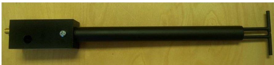
Figure 1 – MVG COMOSAR Validation Dipole
