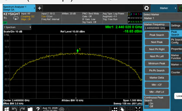
GFSK (BLE 1Mbps) MIDDLE CHANNEL
