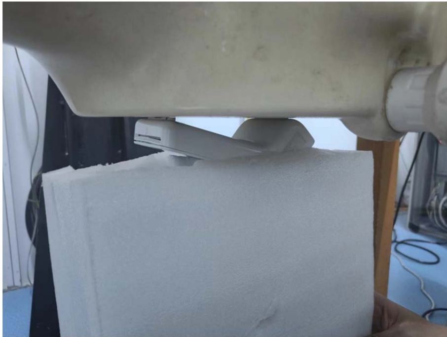
Sensor On Body Back Setup Without device holder Photo (0mm)
