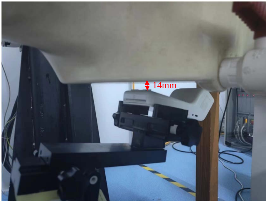
Sensor Off Body Back Setup Photo (14mm)
