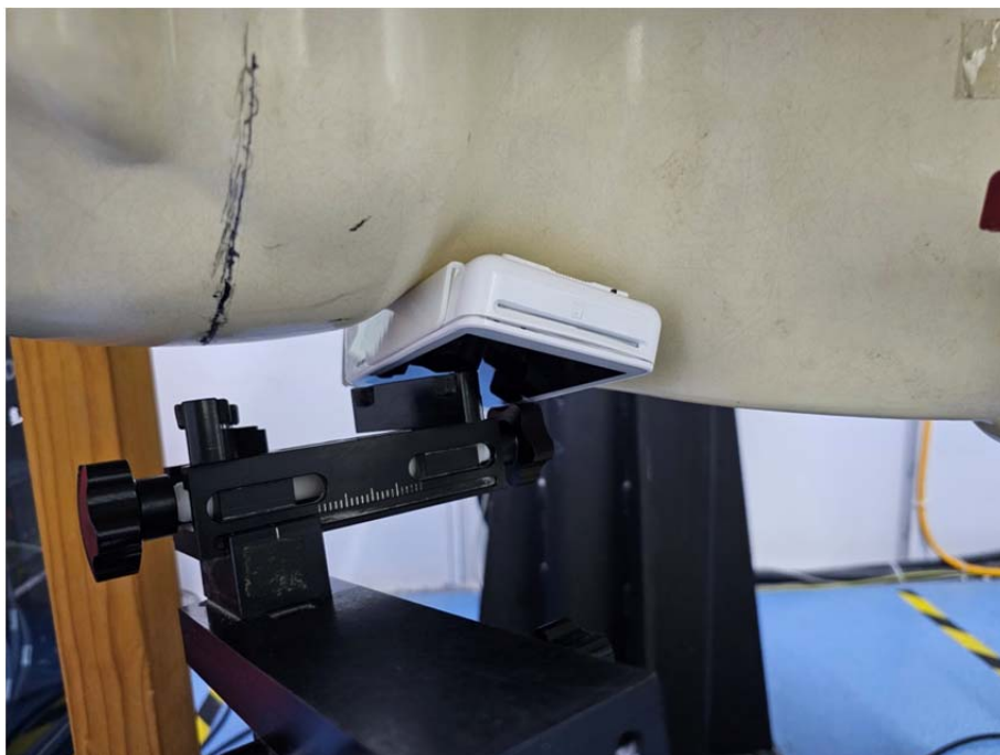
Handheld Back Setup Photo For WiFi/BT (0mm)
