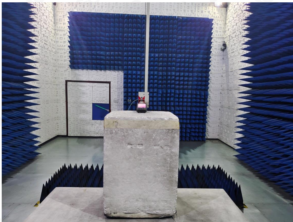
FCC RADIATED EMISSION TEST SETUP ABOVE 1GHZ
