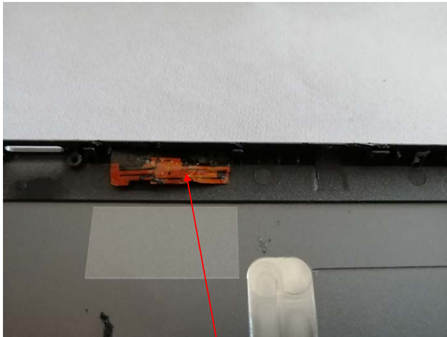
BT antenna / wifi antenna
