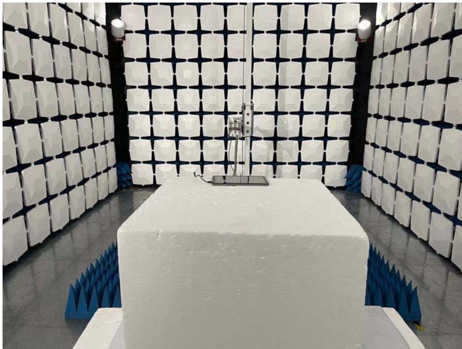
Above 1GHz for radiated emission test setup
