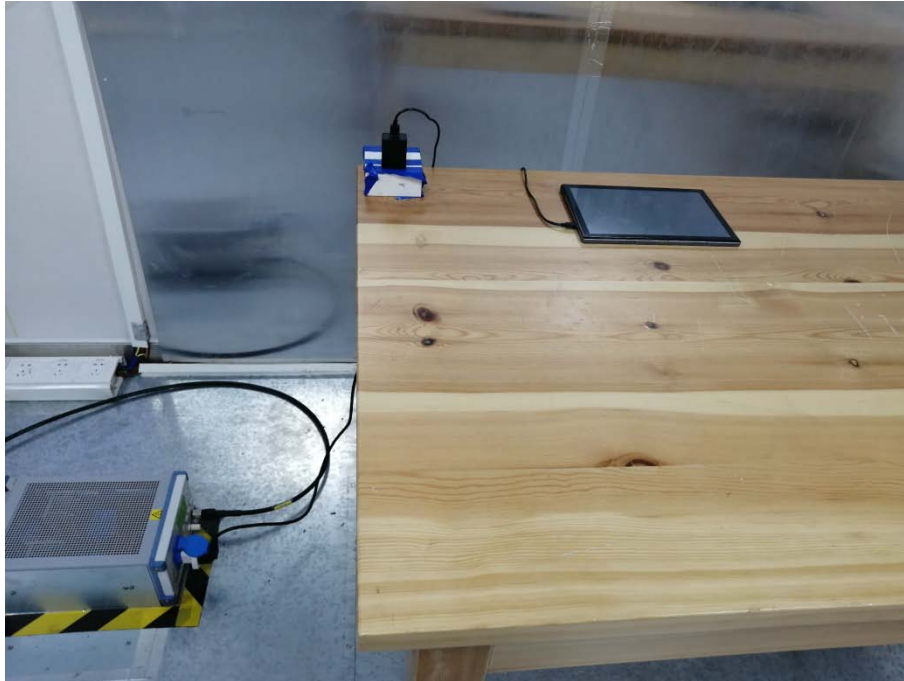
Conducted emission test setup
