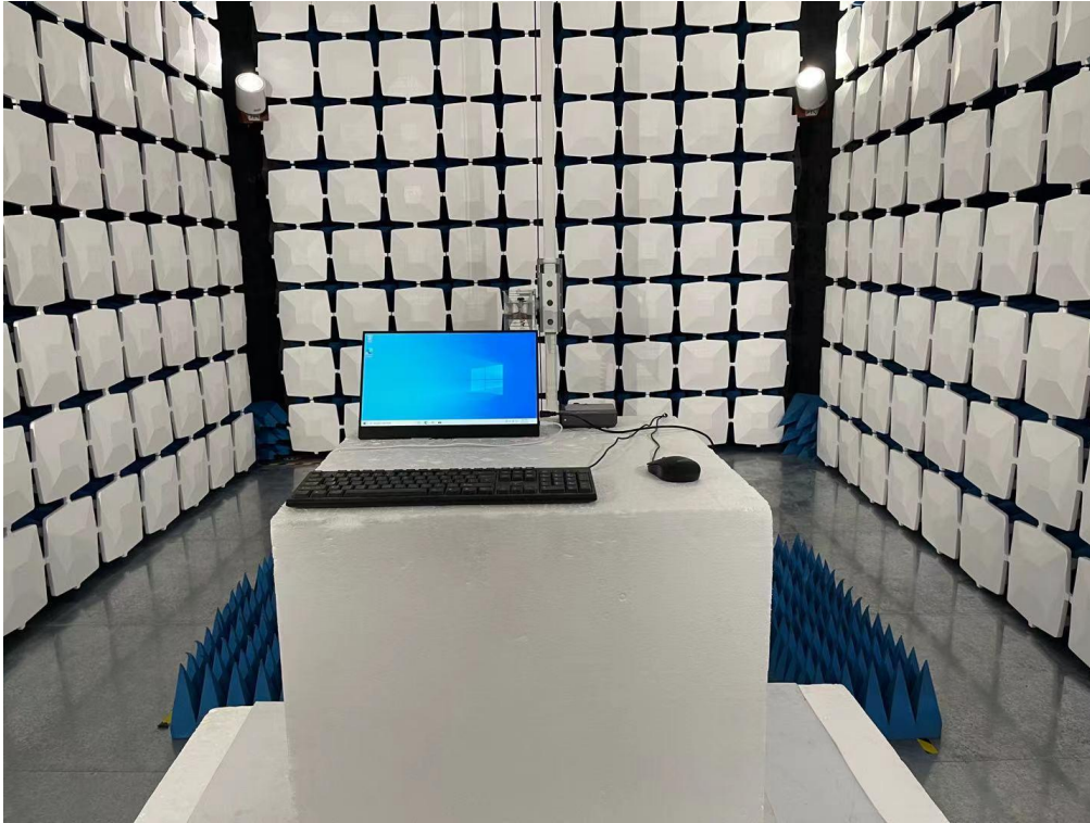
Above 1GHz for radiated emission test setup
