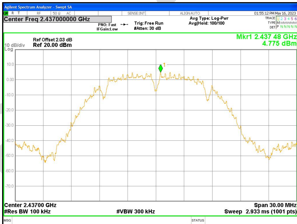
Tx. Spurious NVNT b 2437MHz Ant1 Emission
