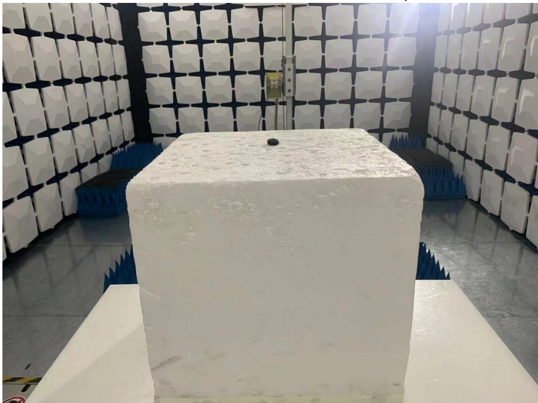
Above 1GHz for radiated emission test setup
