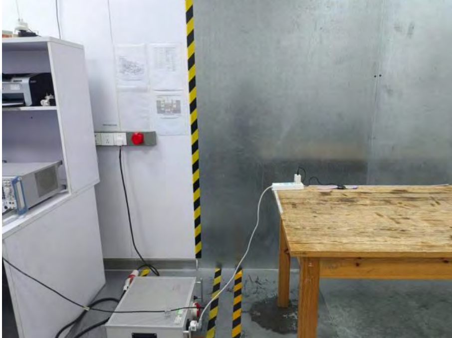
Conducted Emission at AC power line
