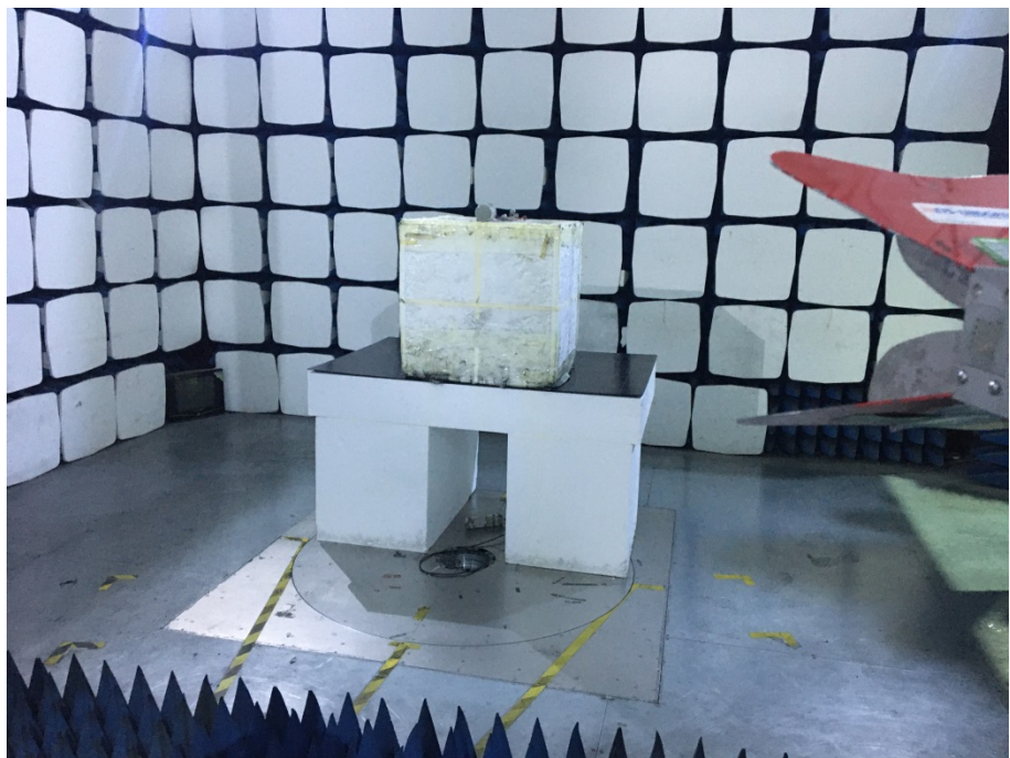
Radiation Emission Test Setup (1GHz to 18GHz)
