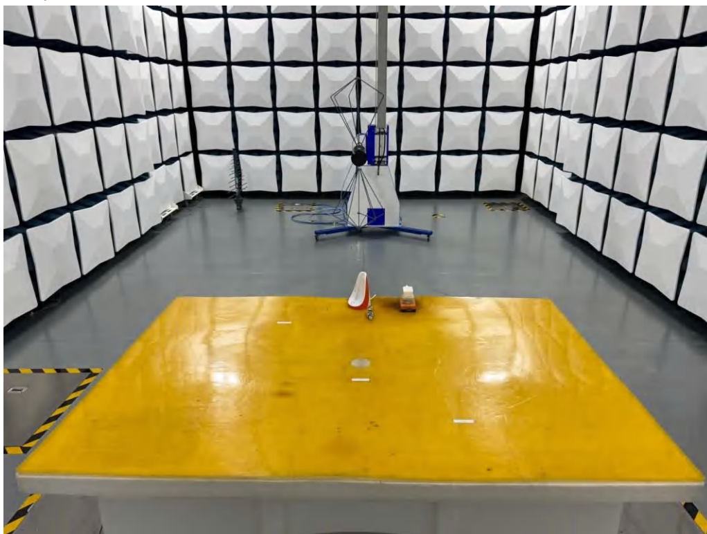
Set-up for Radiated Emission (30MHz-200MHz)
