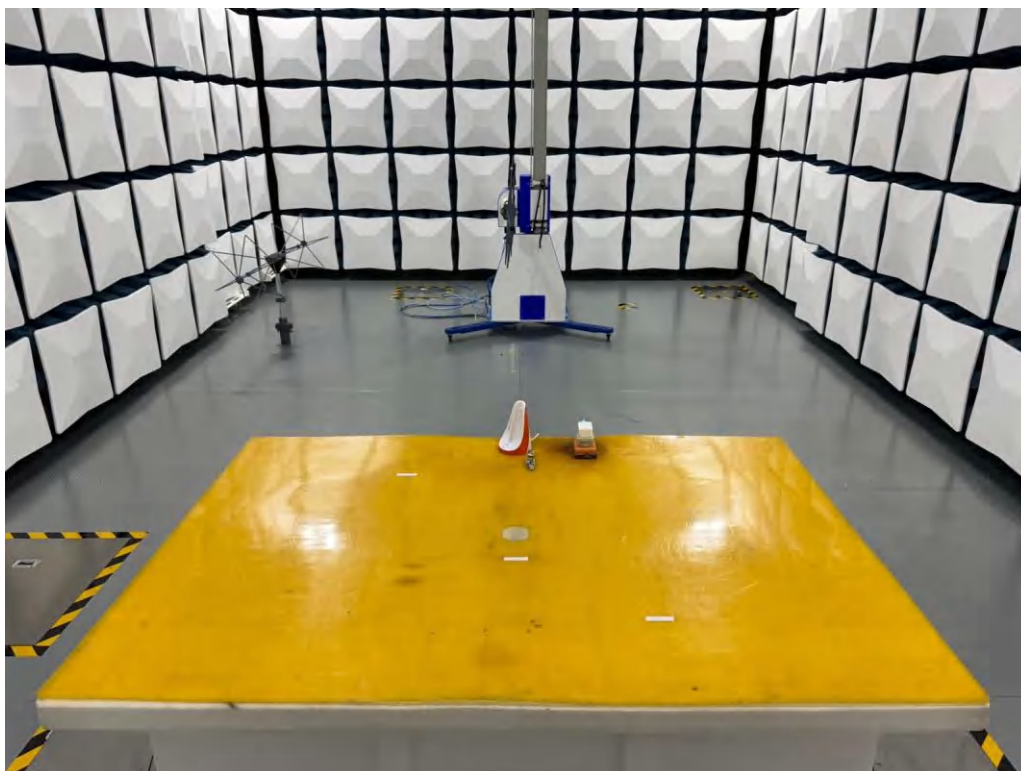
Set-up for Radiated Emission (200MHz-1000MHz)
