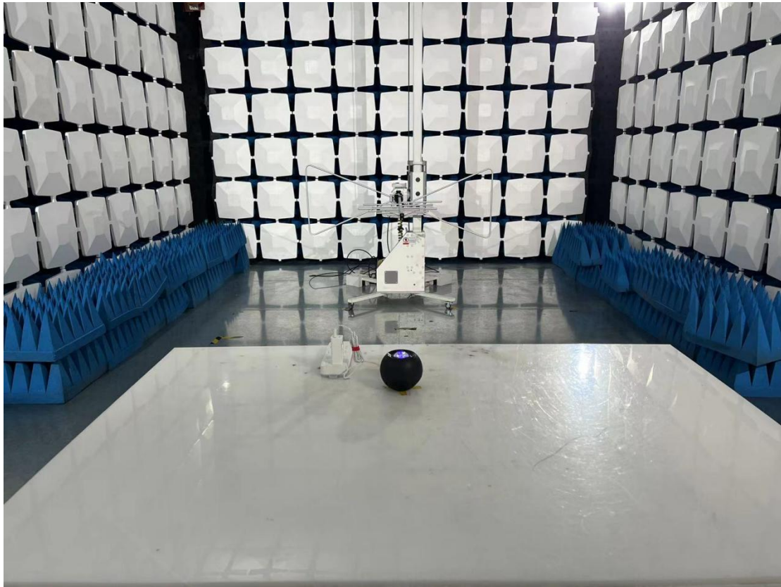
Below 1GHz for radiated emission test setup
