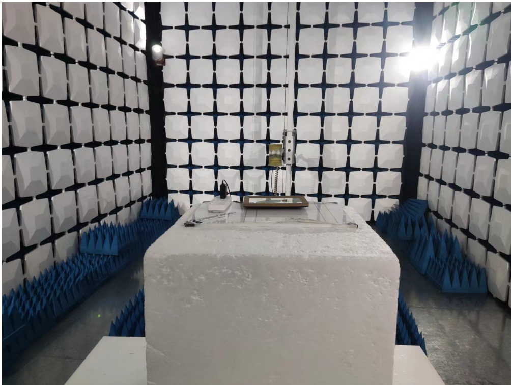
Above 1GHz for radiated emission test setup
