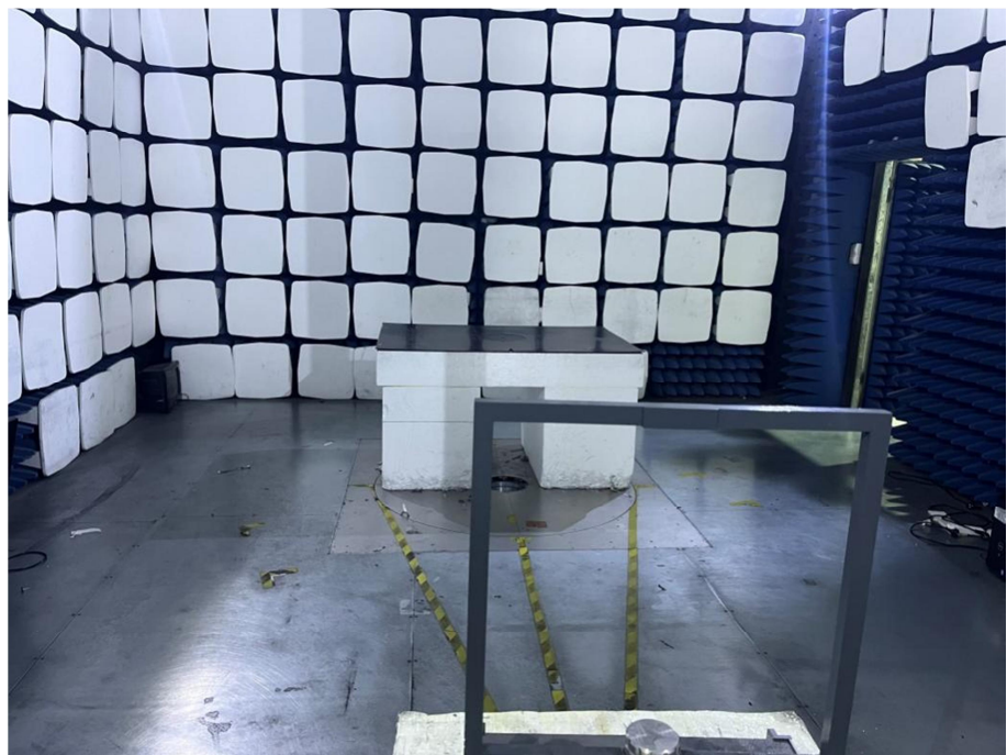
Radiation Emission Test Setup (Below 30MHz)
