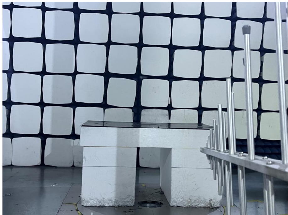
Radiation Emission Test Setup (30MHz to 1GHz)
