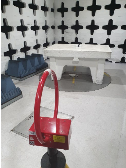
6kHz-30MHz test setup.
