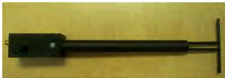
Figure 1 – MVG COMOSAR Validation Dipole
