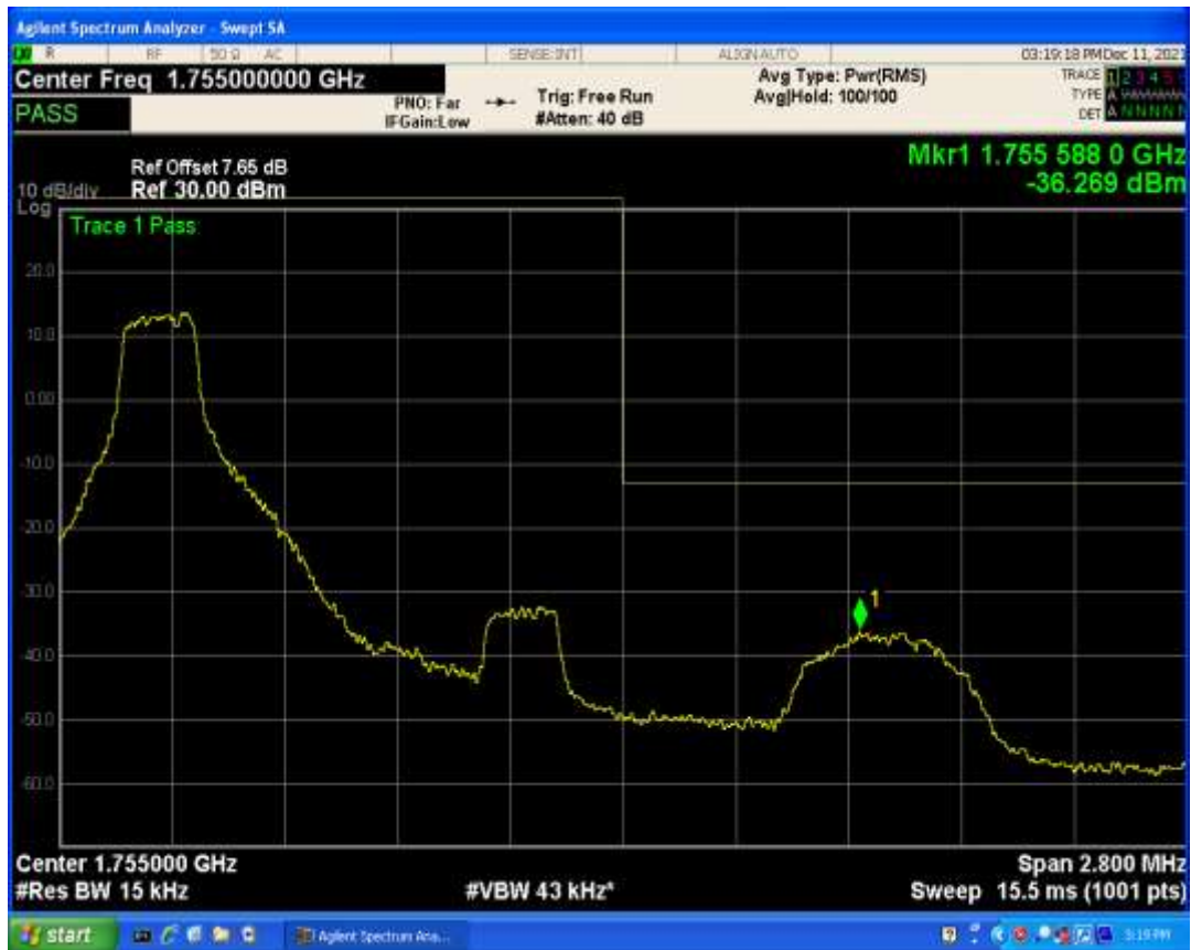
Band4 QAM16 BW=1.4MHz Channel=20393 RB Size=1 Position=#Max
