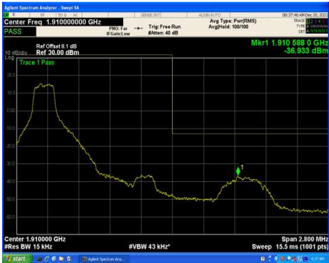
Band2 QAM16 BW=1.4MHz Channel=18607 RB Size=6 Position=#0
