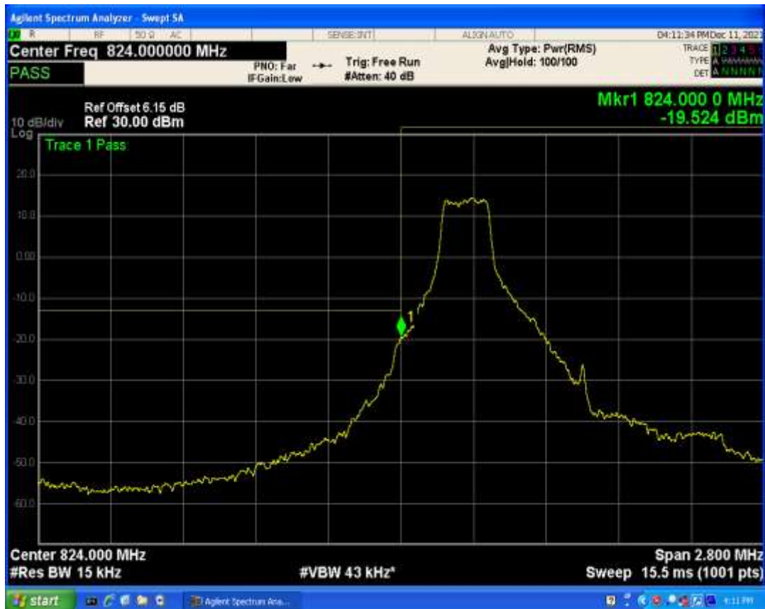
Band5 QPSK BW=1.4MHz Channel=20407 RB Size=6 Position=#0
