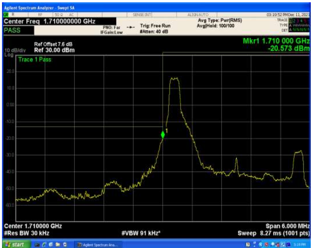
Band4 QAM16 BW=3MHz Channel=19965 RB Size=1 Position=#Max
