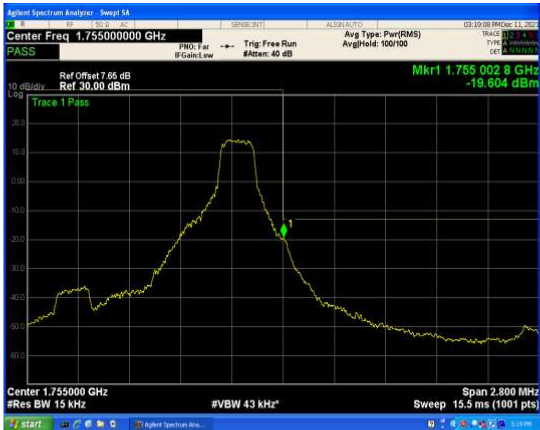
Band4 QPSK BW=1.4MHz Channel=20393 RB Size=6 Position=#0
