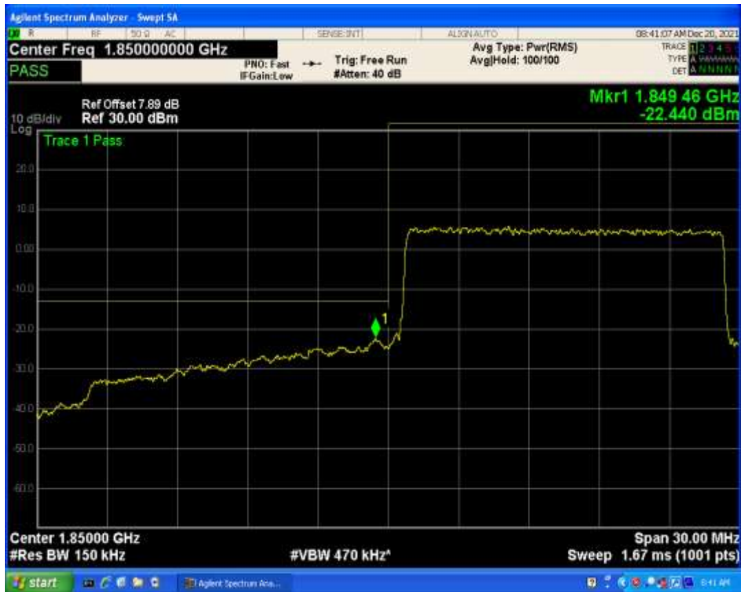
Band2 QAM16 BW=15MHz Channel=18675 RB Size=1 Position=#Max
