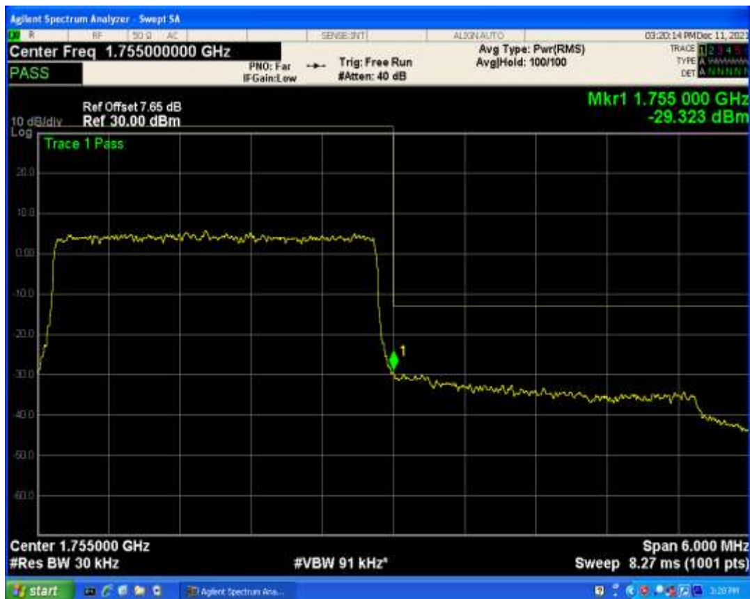
Band4 QAM16 BW=3MHz Channel=20385 RB Size=1 Position=#0
