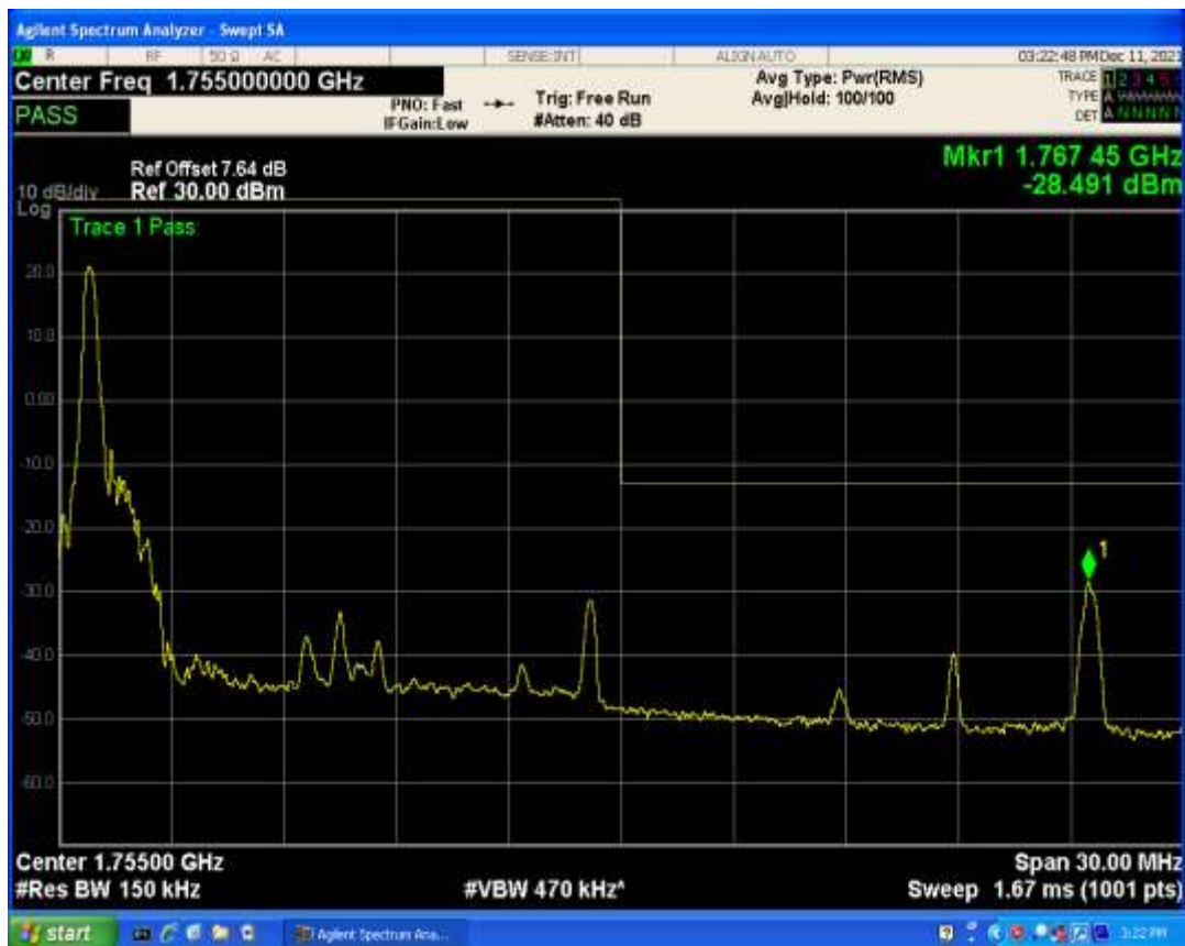
Band4 QAM16 BW=15MHz Channel=20325 RB Size=75 Position=#0
