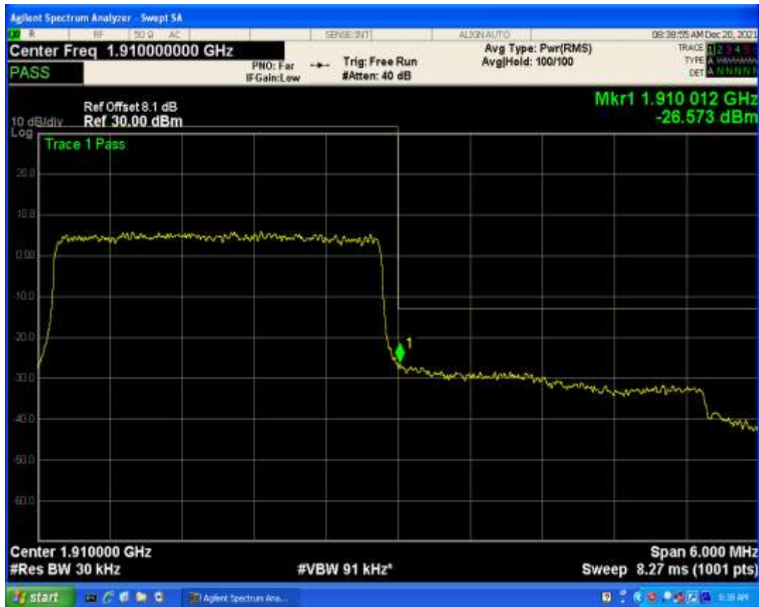
Band2 QAM16 BW=3MHz Channel=19185 RB Size=1 Position=#Max
