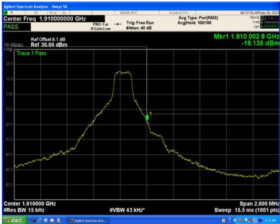
Band2 QPSK BW=1.4MHz Channel=19193 RB Size=6 Position=#0
