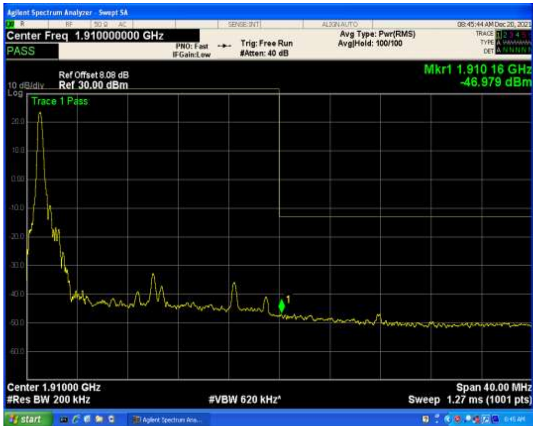
Band2 QAM16 BW=20MHz Channel=18700 RB Size=100 Position=#0
