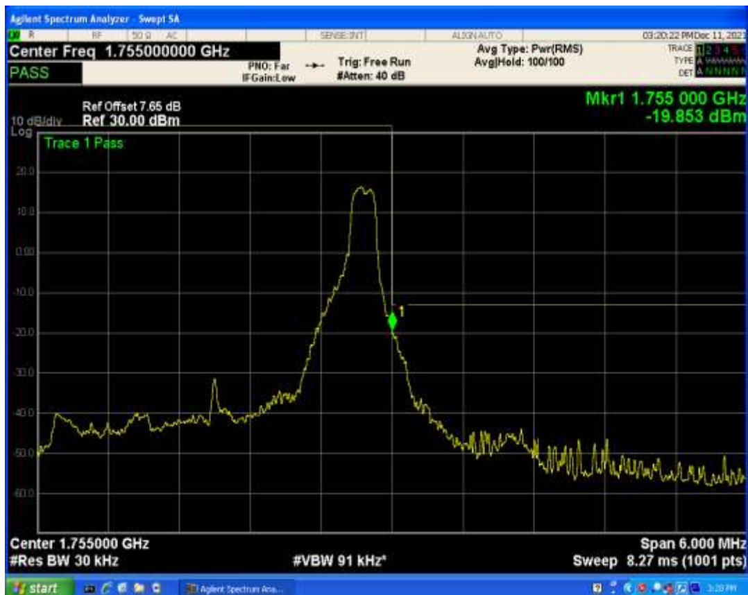
Band4 QAM16 BW=3MHz Channel=20385 RB Size=15 Position=#0
