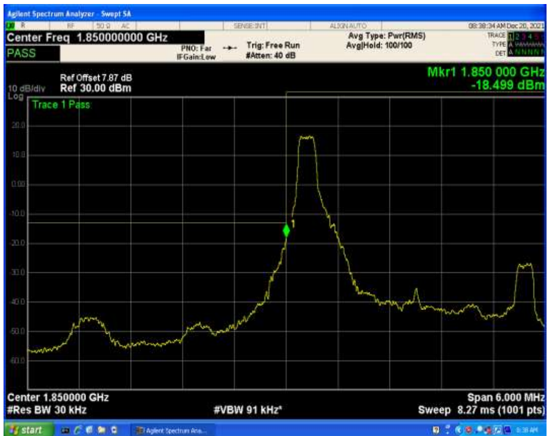
Band2 QPSK BW=3MHz Channel=18615 RB Size=15 Position=#0
