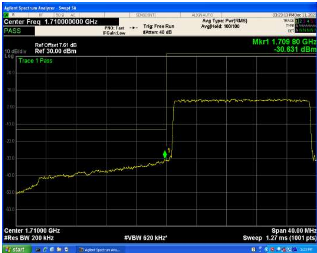
Band4 QAM16 BW=20MHz Channel=20050 RB Size=1 Position=#Max
