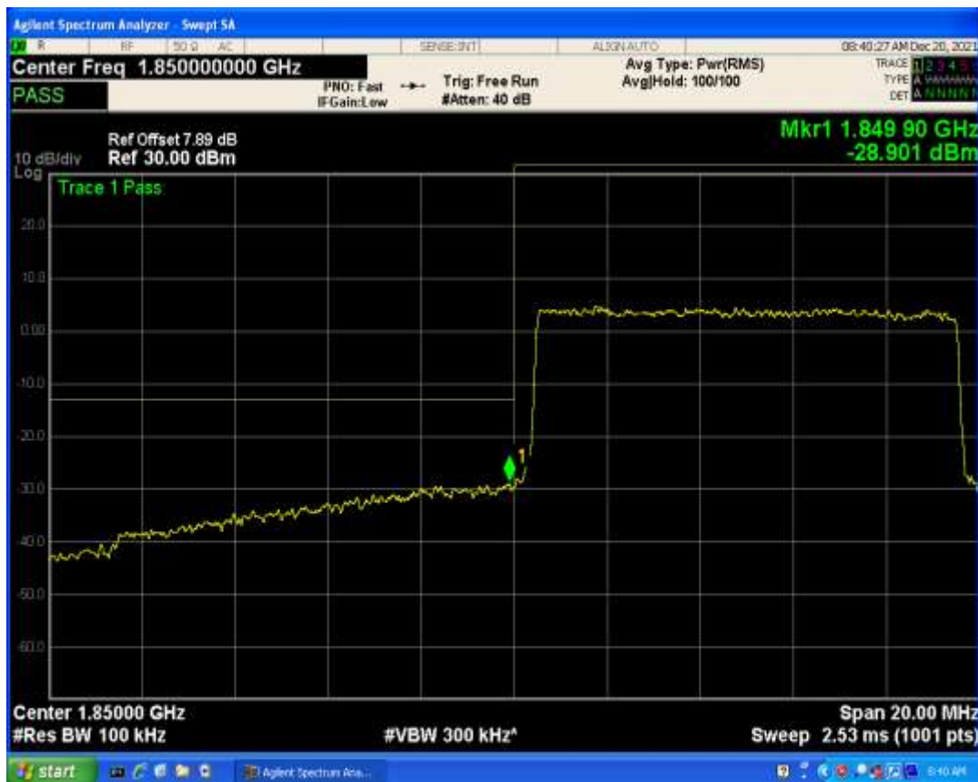
Band2 QPSK BW=10MHz Channel=19150 RB Size=1 Position=#Max
