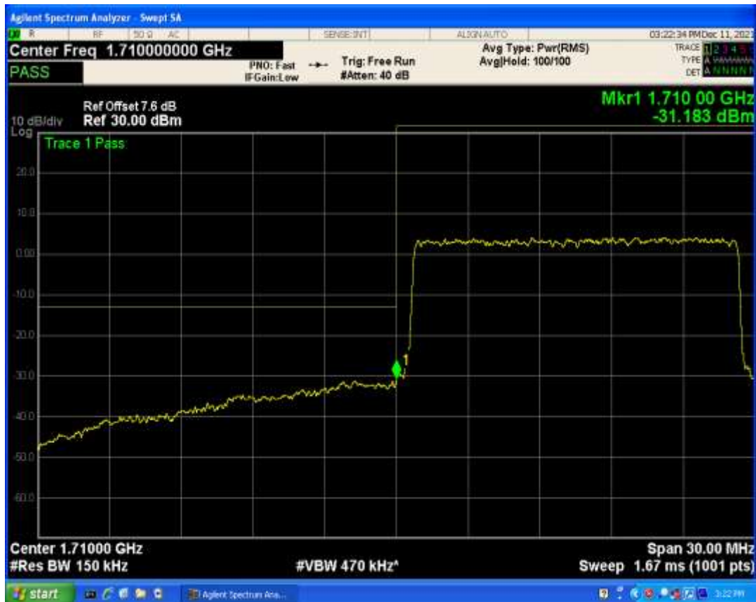
Band4 QPSK BW=15MHz Channel=20325 RB Size=1 Position=#0
