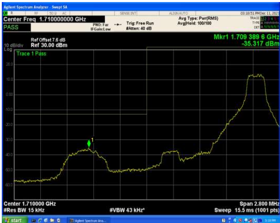
Band4 QAM16 BW=1.4MHz Channel=19957 RB Size=6 Position=#0
