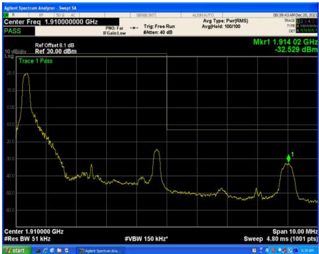
Band2 QPSK BW=5MHz Channel=19175 RB Size=1 Position=#Max
