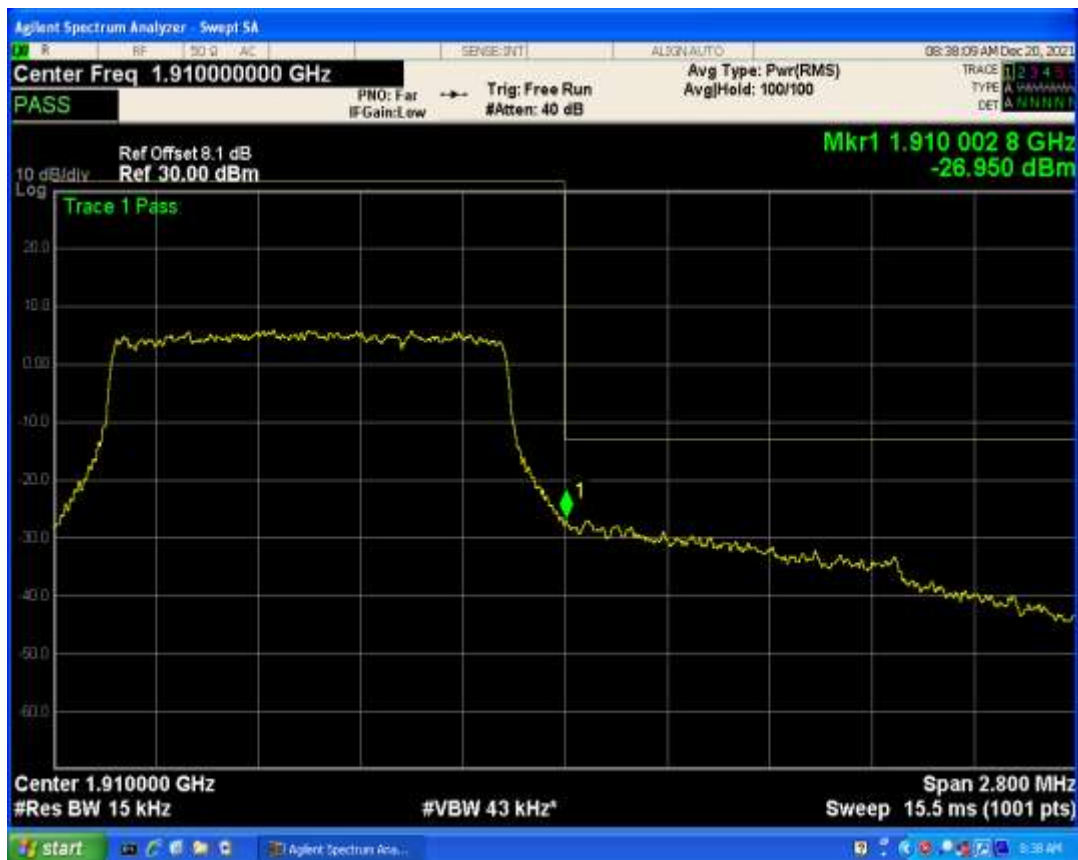
Band2 QPSK BW=3MHz Channel=18615 RB Size=1 Position=#Max
