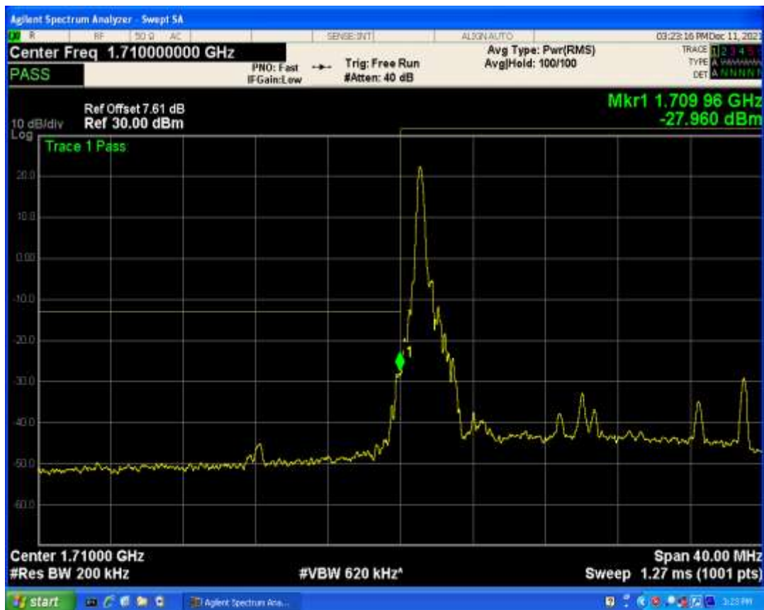
Band4 QAM16 BW=20MHz Channel=20050 RB Size=100 Position=#0
