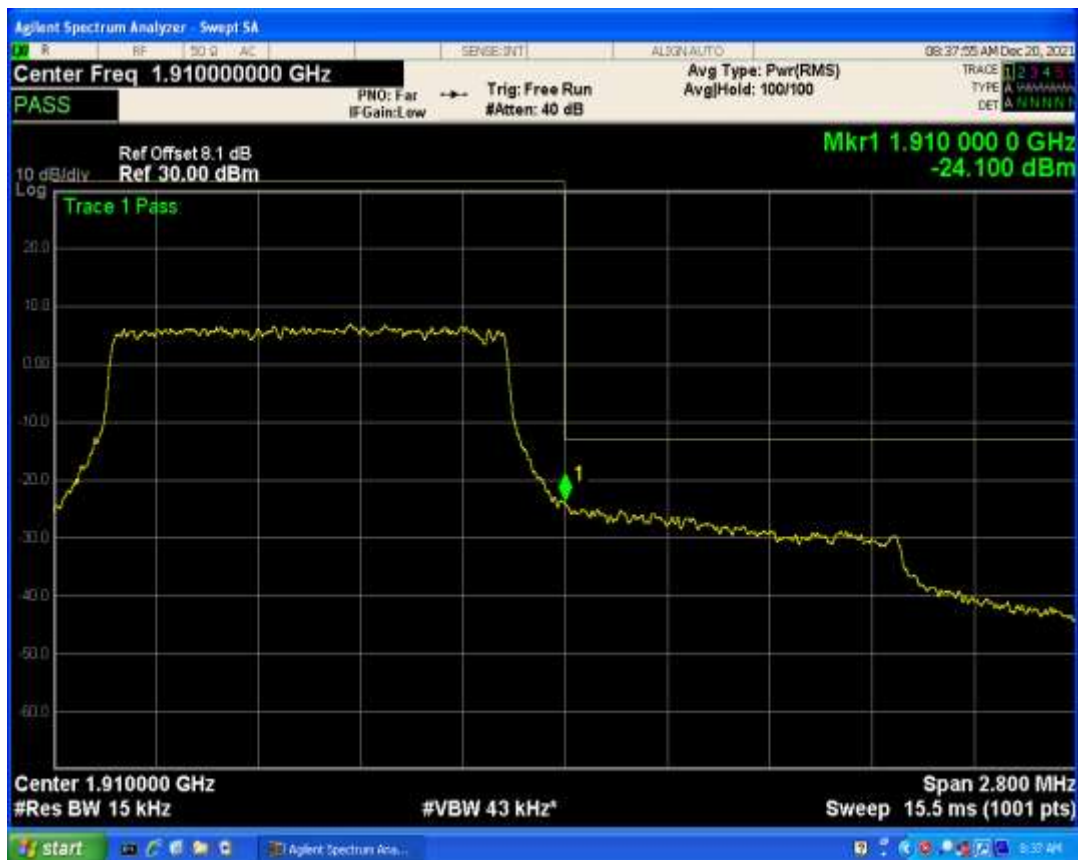
Band2 QAM16 BW=1.4MHz Channel=19193 RB Size=1 Position=#0
