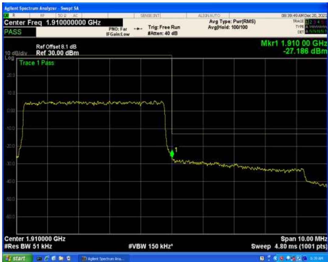
Band2 QAM16 BW=5MHz Channel=19175 RB Size=1 Position=#0
