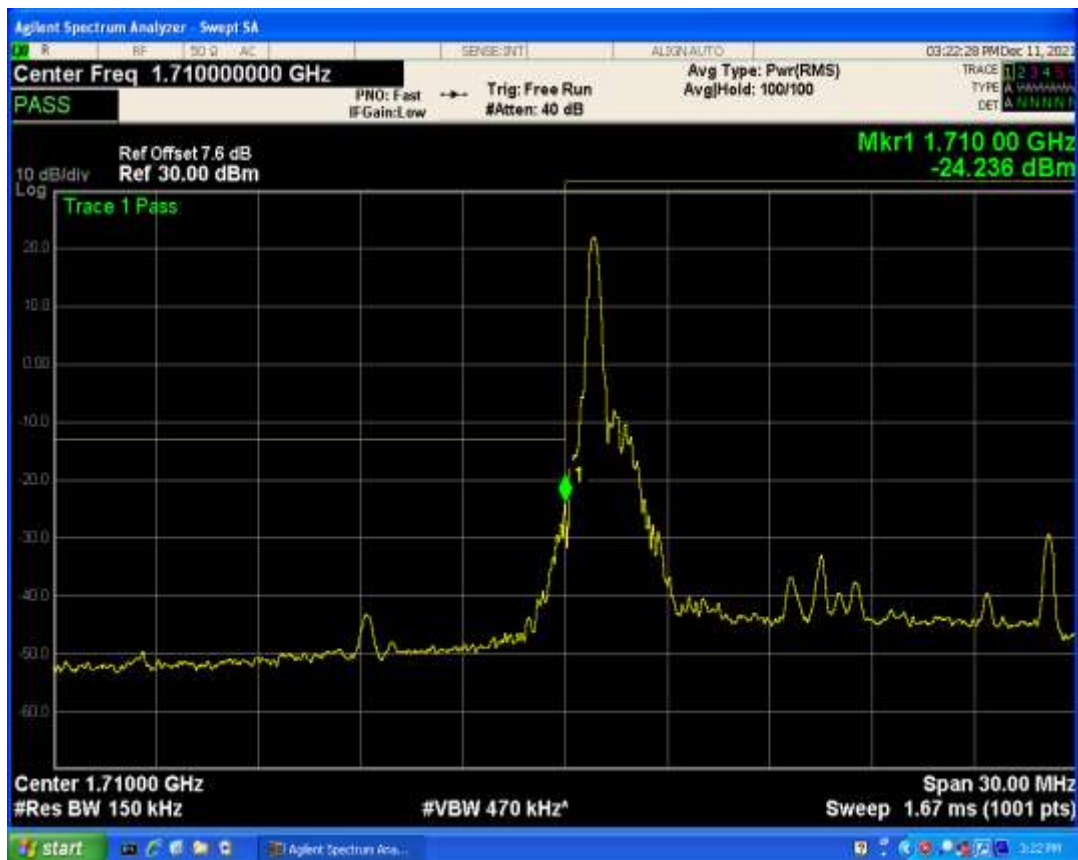
Band4 QAM16 BW=15MHz Channel=20025 RB Size=75 Position=#0
