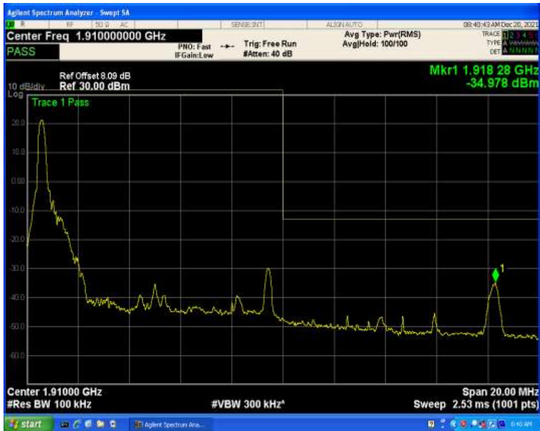
Band2 QAM16 BW=10MHz Channel=19150 RB Size=1 Position=#Max
