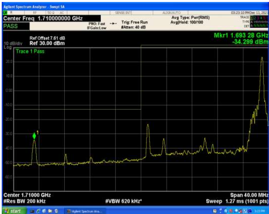
Band4 QPSK BW=20MHz Channel=20050 RB Size=1 Position=#0
