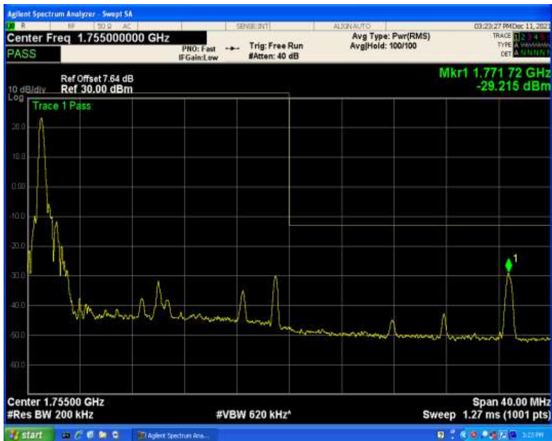
Band4 QPSK BW=20MHz Channel=20300 RB Size=1 Position=#Max
