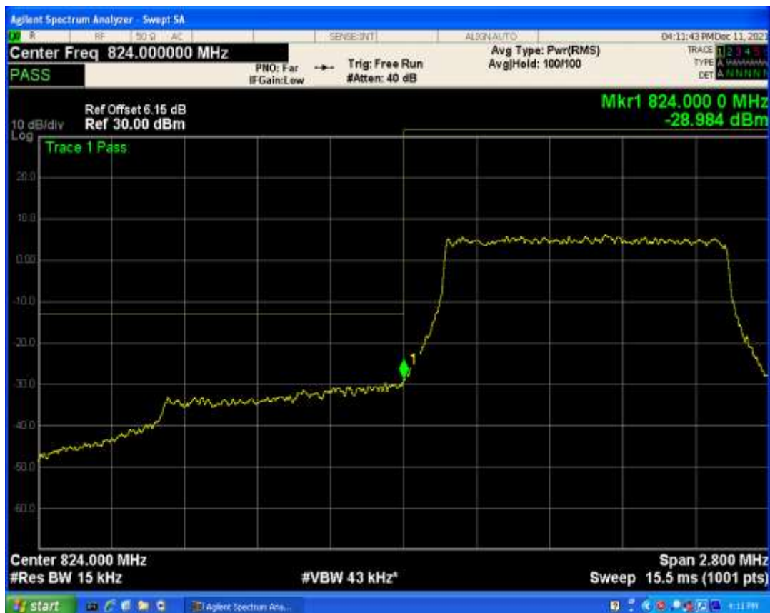
Band5 QAM16 BW=1.4MHz Channel=20407 RB Size=1 Position=#0
