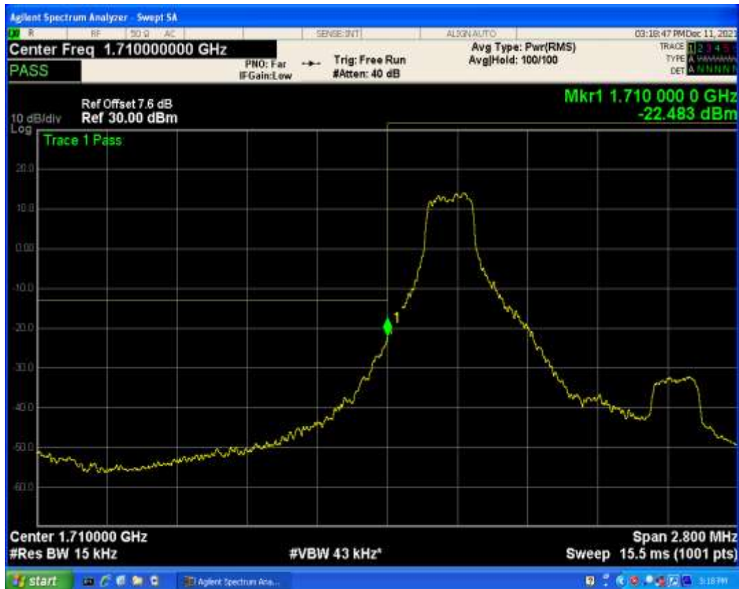
Band4 QAM16 BW=1.4MHz Channel=19957 RB Size=1 Position=#Max
