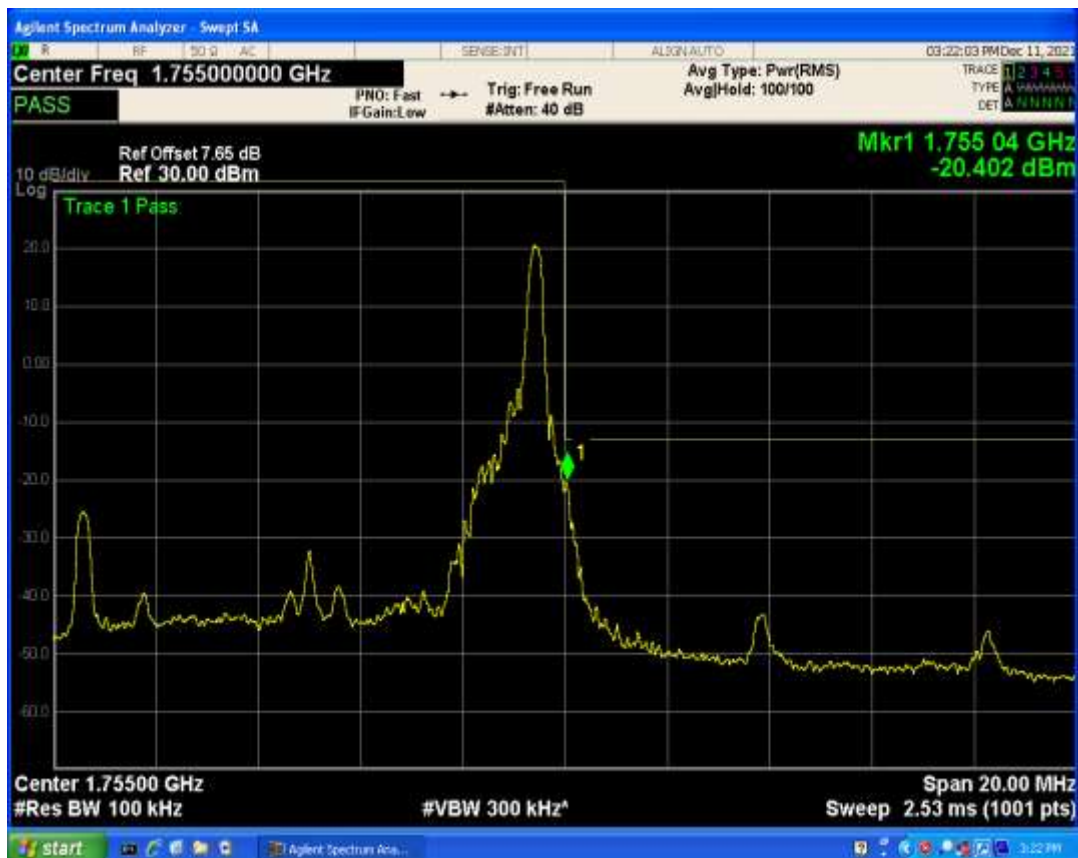
Band4 QAM16 BW=10MHz Channel=20350 RB Size=50 Position=#0
