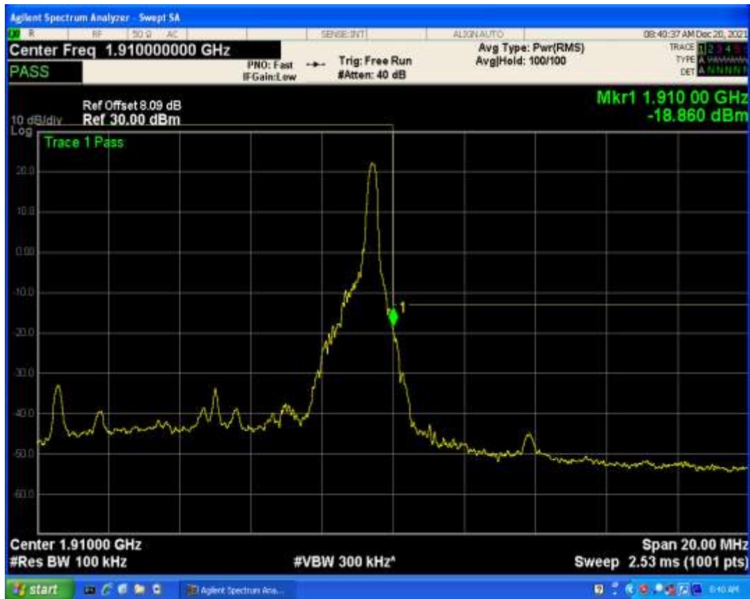
Band2 QPSK BW=10MHz Channel=19150 RB Size=50 Position=#0
