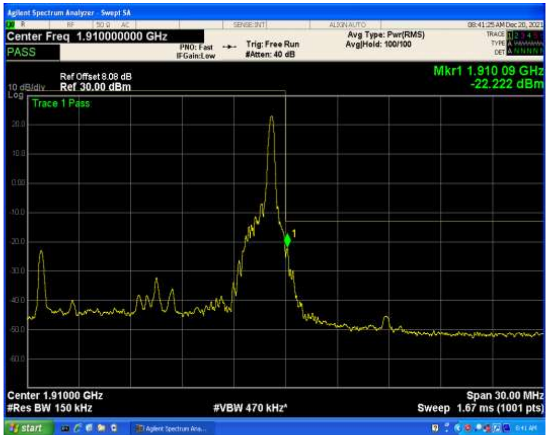
Band2 QAM16 BW=15MHz Channel=19125 RB Size=1 Position=#0
