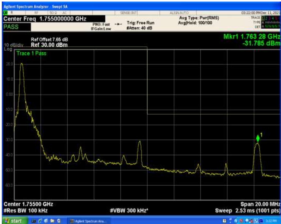
Band4 QAM16 BW=10MHz Channel=20350 RB Size=1 Position=#Max
