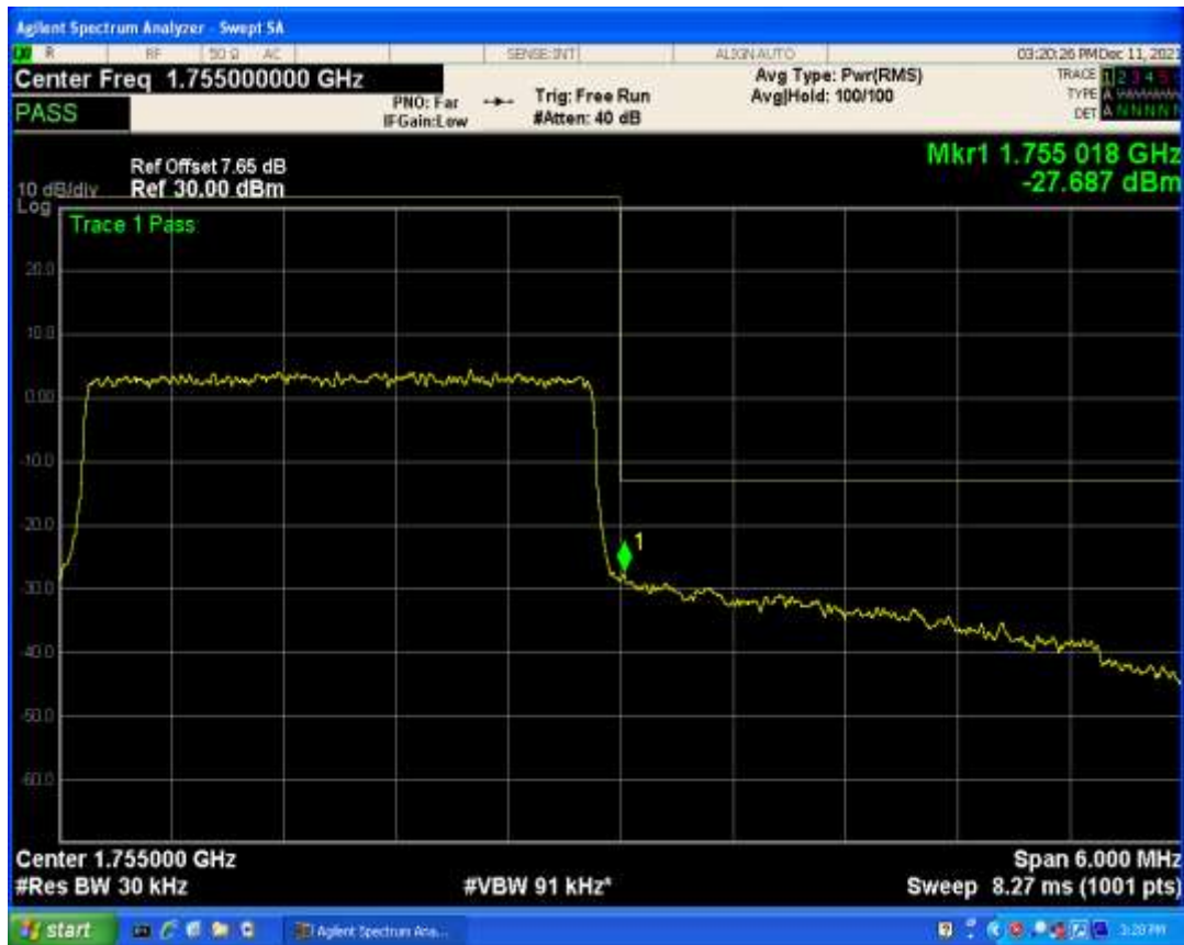
Band4 QPSK BW=5MHz Channel=19975 RB Size=1 Position=#Max
