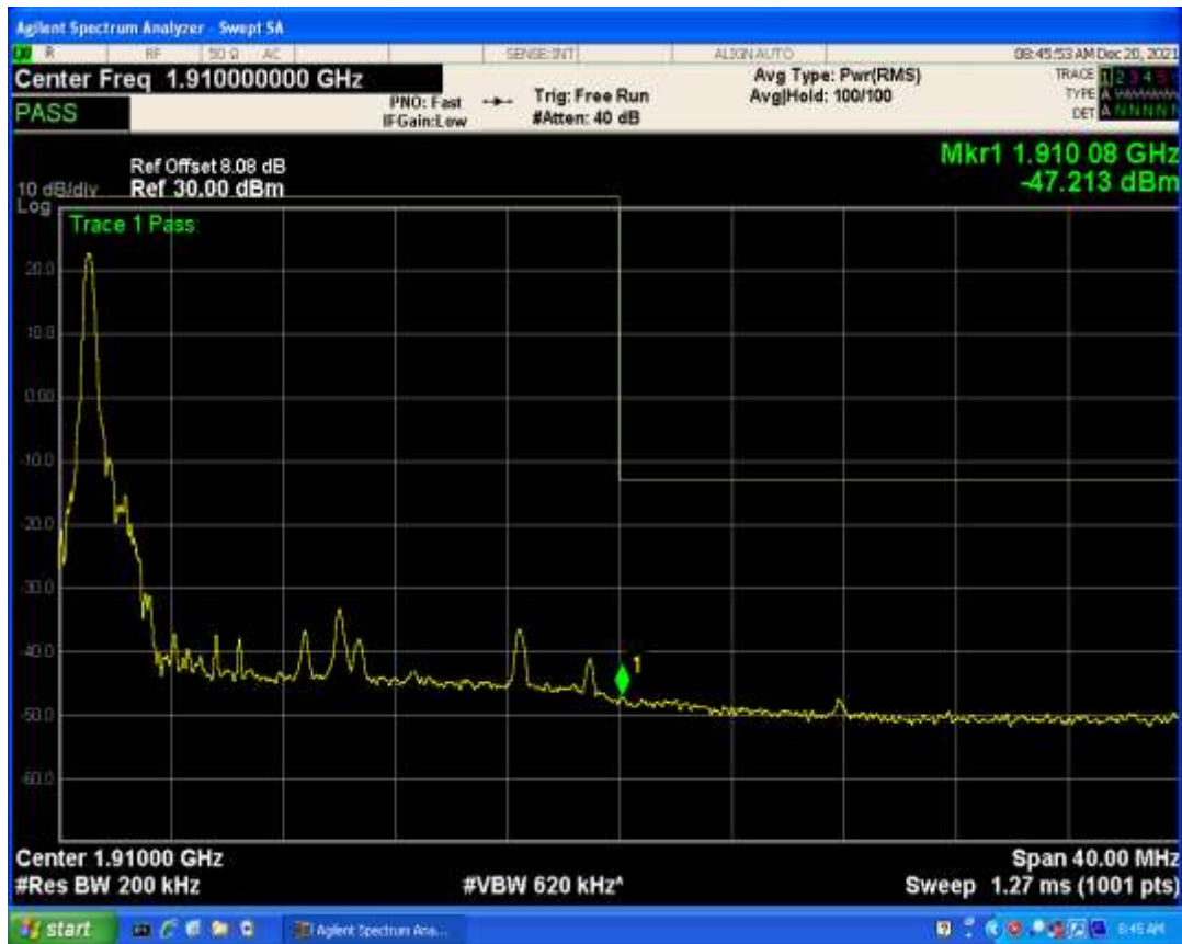
Band2 QAM16 BW=20MHz Channel=19100 RB Size=1 Position=#Max
