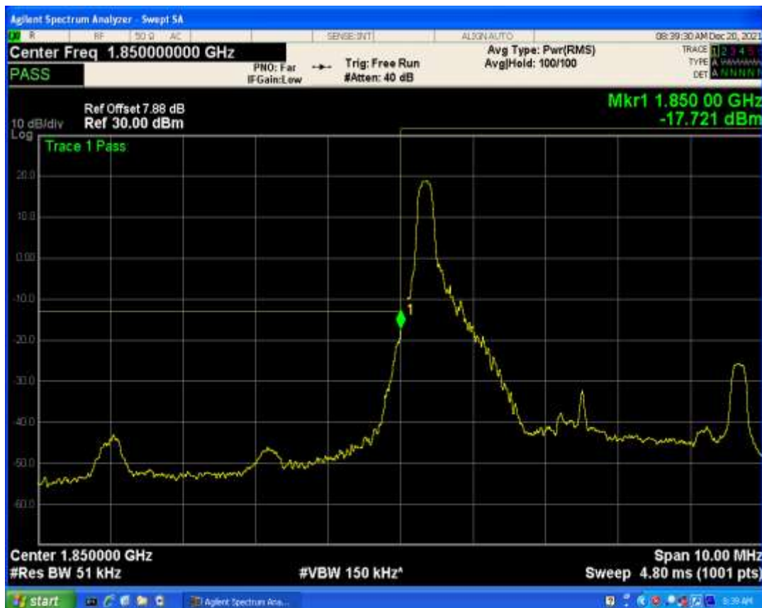
Band2 QPSK BW=5MHz Channel=18625 RB Size=25 Position=#0
