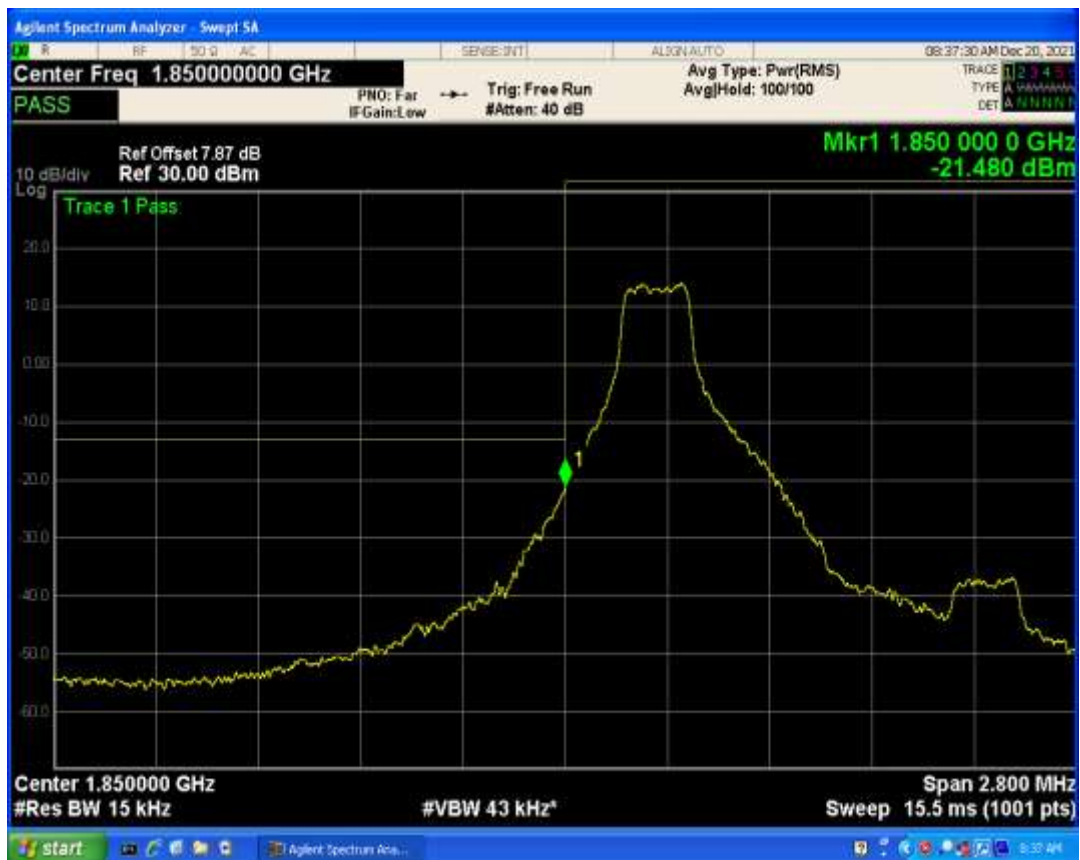
Band2 QPSK BW=1.4MHz Channel=18607 RB Size=6 Position=#0
