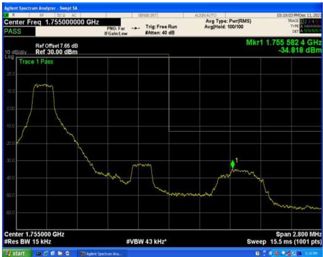
Band4 QPSK BW=1.4MHz Channel=20393 RB Size=1 Position=#Max
