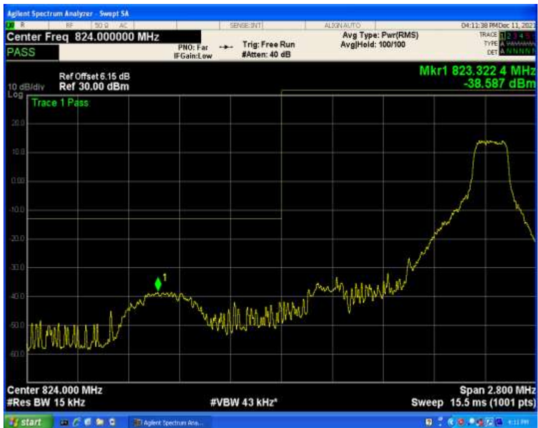
Band5 QPSK BW=1.4MHz Channel=20407 RB Size=1 Position=#0
