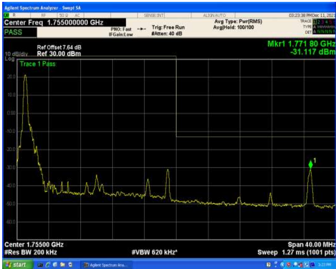
Band4 QAM16 BW=20MHz Channel=20300 RB Size=1 Position=#Max
