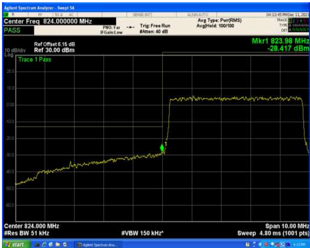
Band5 QAM16 BW=5MHz Channel=20425 RB Size=1 Position=#0
