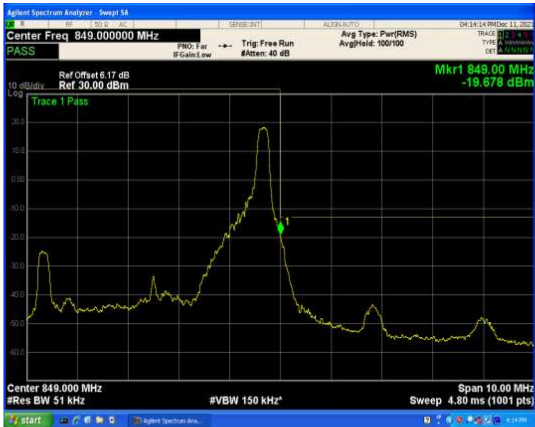
Band5 QAM16 BW=5MHz Channel=20625 RB Size=1 Position=#0
