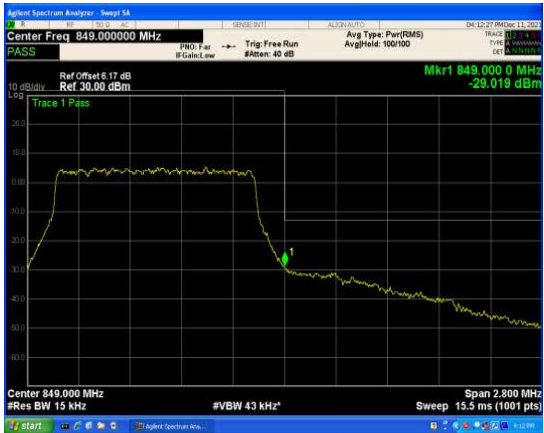
Band5 QPSK BW=3MHz Channel=20415 RB Size=1 Position=#0
