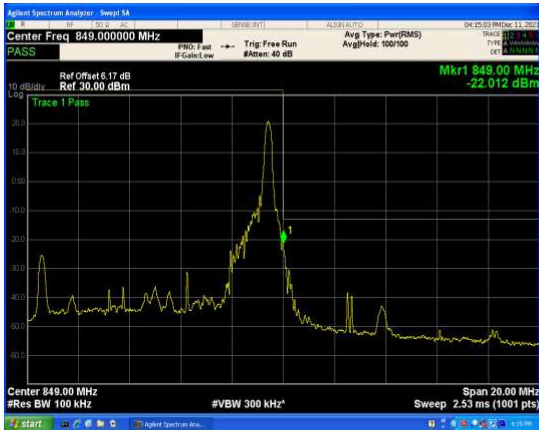
Band5 QAM16 BW=10MHz Channel=20600 RB Size=1 Position=#0
