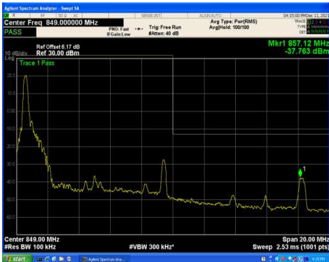
Band5 QAM16 BW=10MHz Channel=20600 RB Size=50 Position=#0
