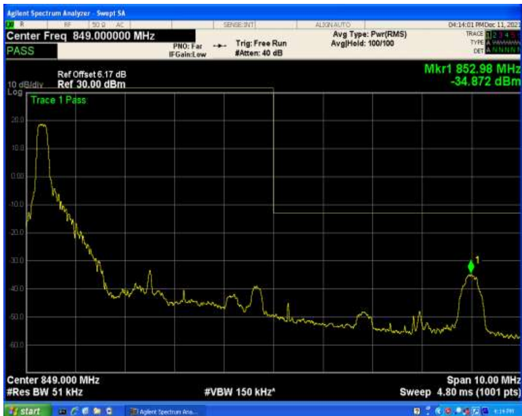
Band5 QPSK BW=5MHz Channel=20625 RB Size=1 Position=#Max
