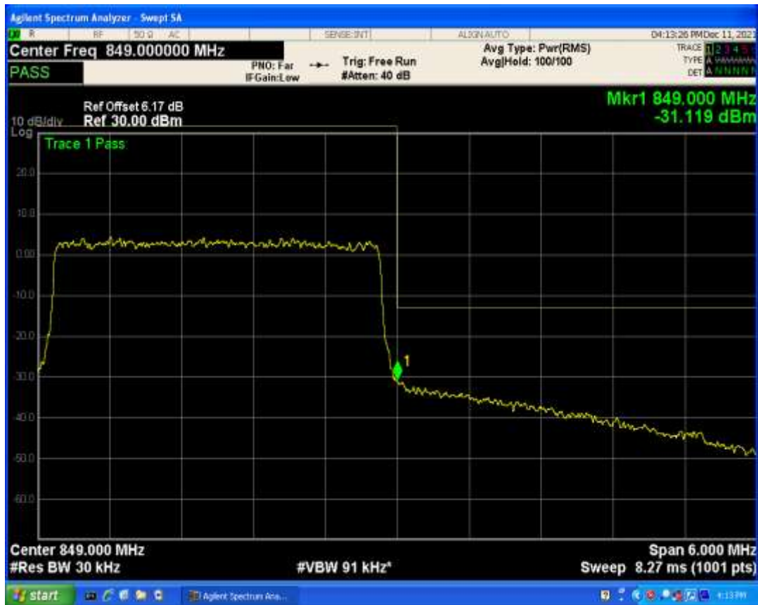
Band5 QPSK BW=5MHz Channel=20425 RB Size=1 Position=#0
