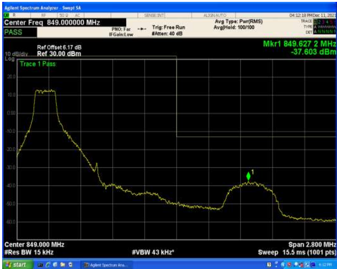
Band5 QAM16 BW=1.4MHz Channel=20643 RB Size=1 Position=#Max
