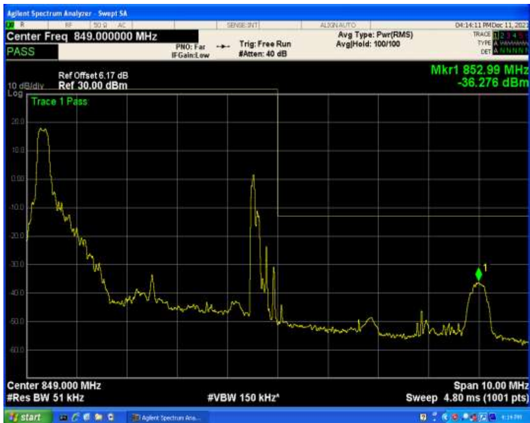
Band5 QAM16 BW=5MHz Channel=20625 RB Size=25 Position=#0
