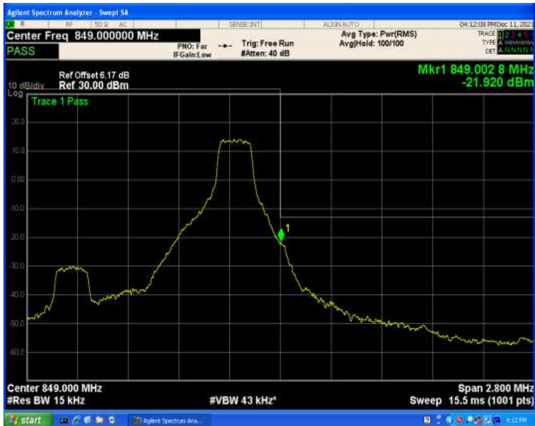
Band5 QPSK BW=1.4MHz Channel=20643 RB Size=6 Position=#0
