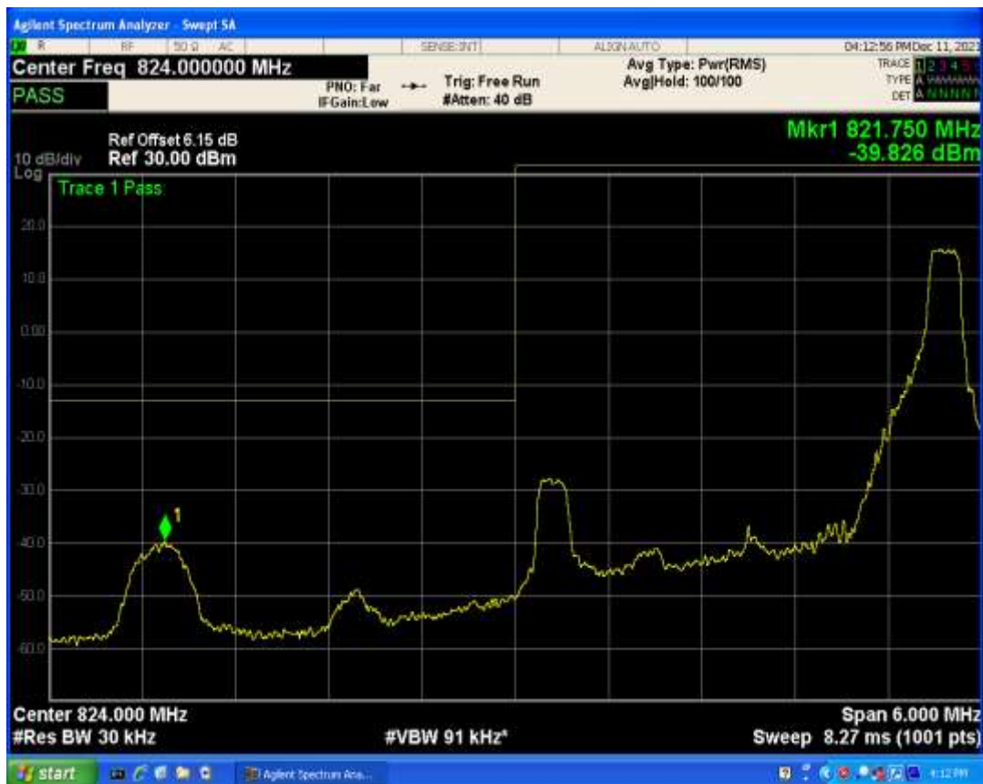
Band5 QAM16 BW=3MHz Channel=20415 RB Size=15 Position=#0
