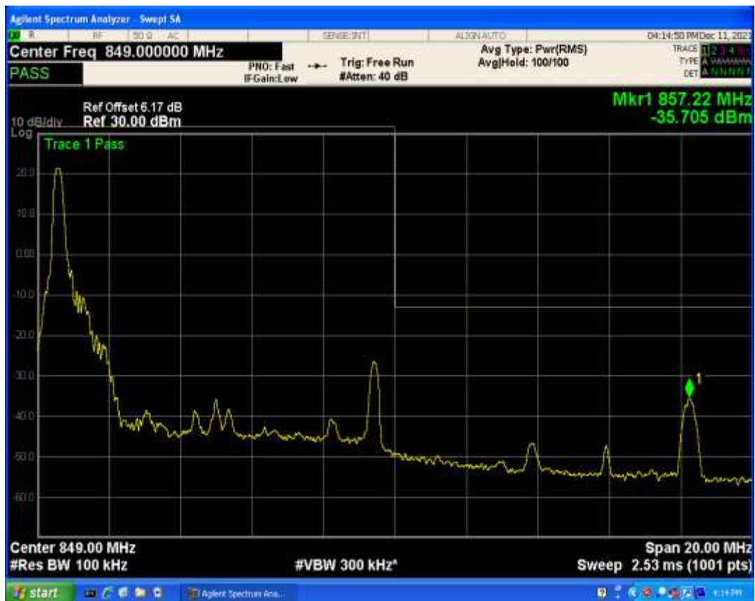
Band5 QPSK BW=10MHz Channel=20600 RB Size=1 Position=#Max
