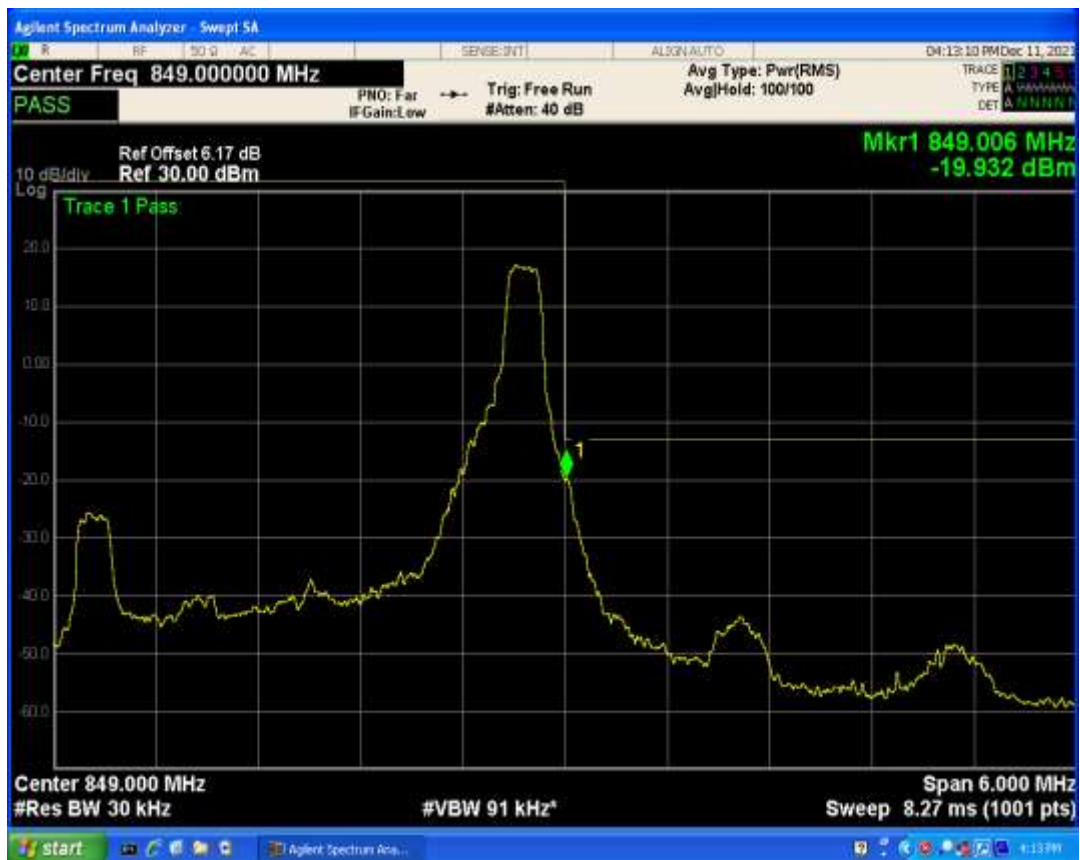
Band5 QPSK BW=3MHz Channel=20635 RB Size=1 Position=#0
