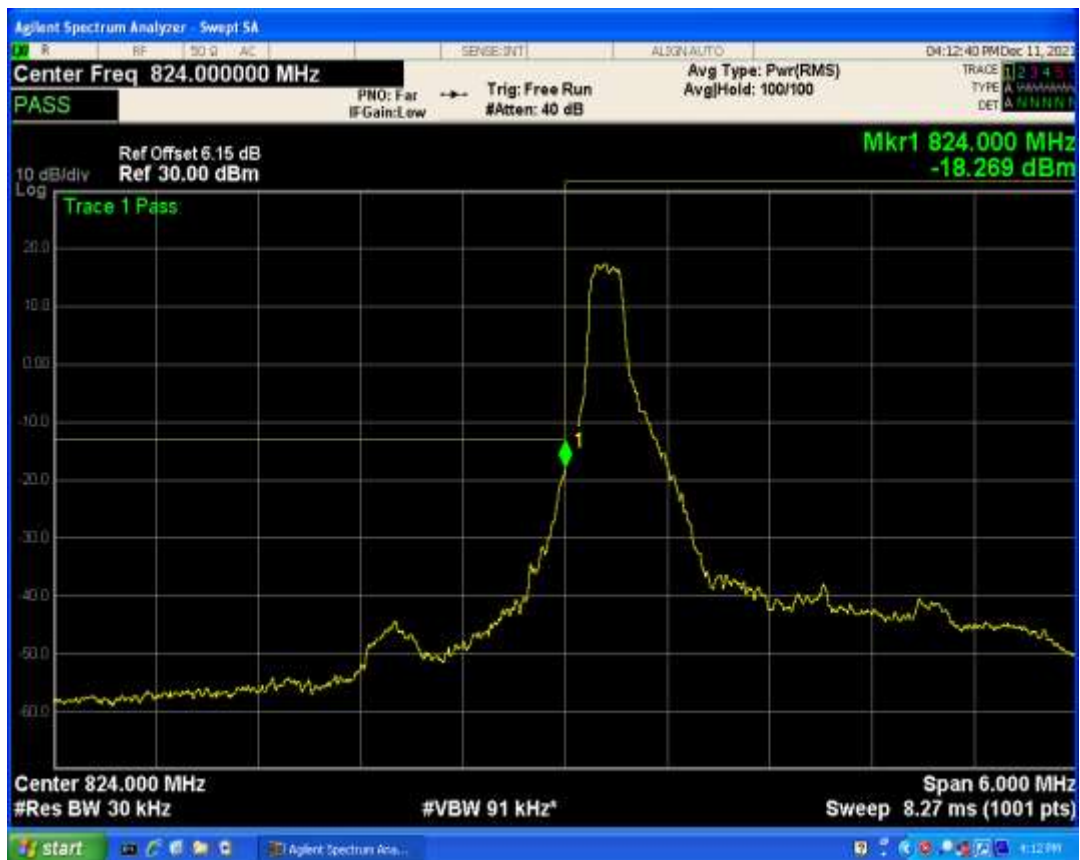
Band5 QPSK BW=3MHz Channel=20415 RB Size=1 Position=#Max
