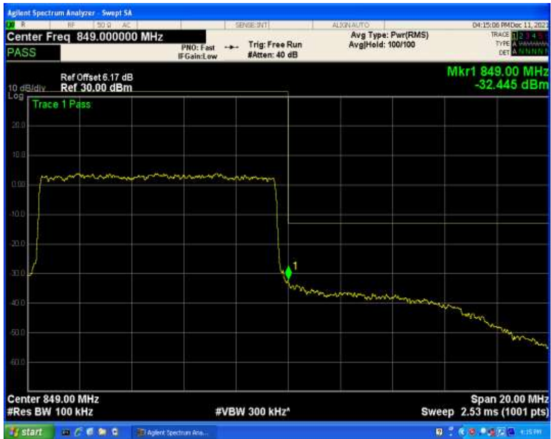
Band7 QPSK BW=5MHz Channel=20775 RB Size=1 Position=#0
