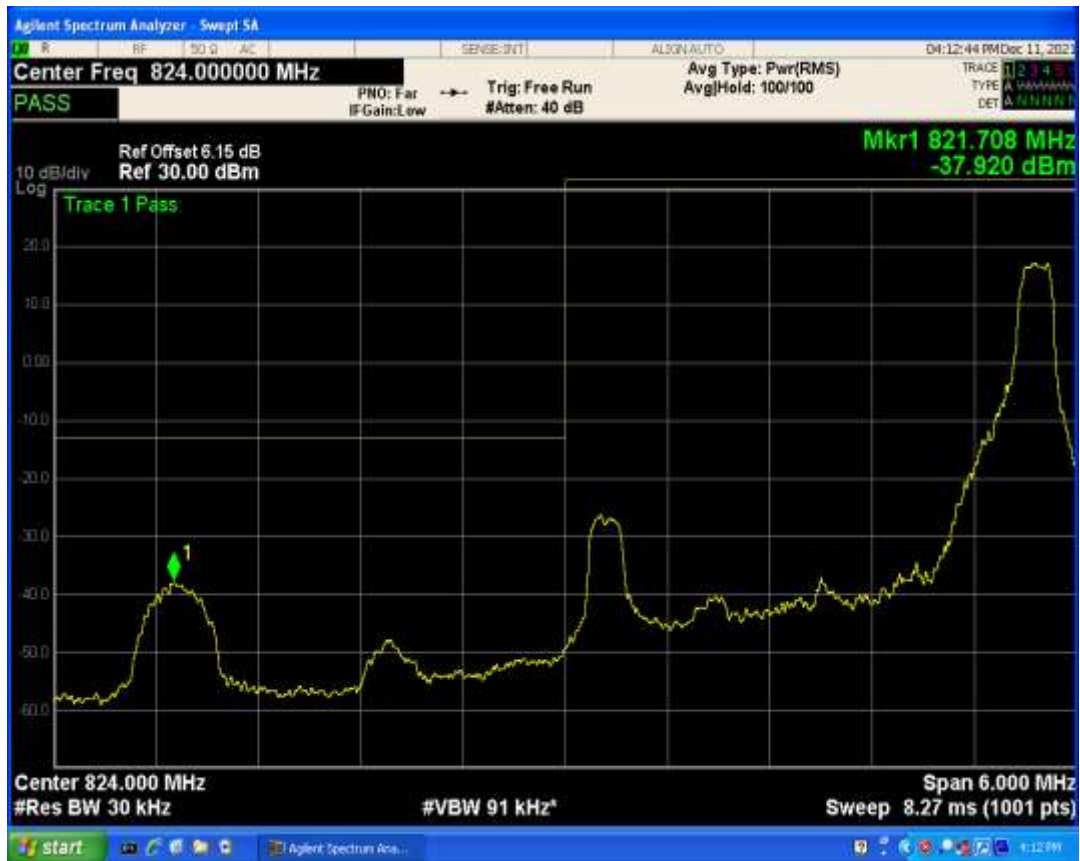
Band5 QPSK BW=3MHz Channel=20415 RB Size=15 Position=#0
