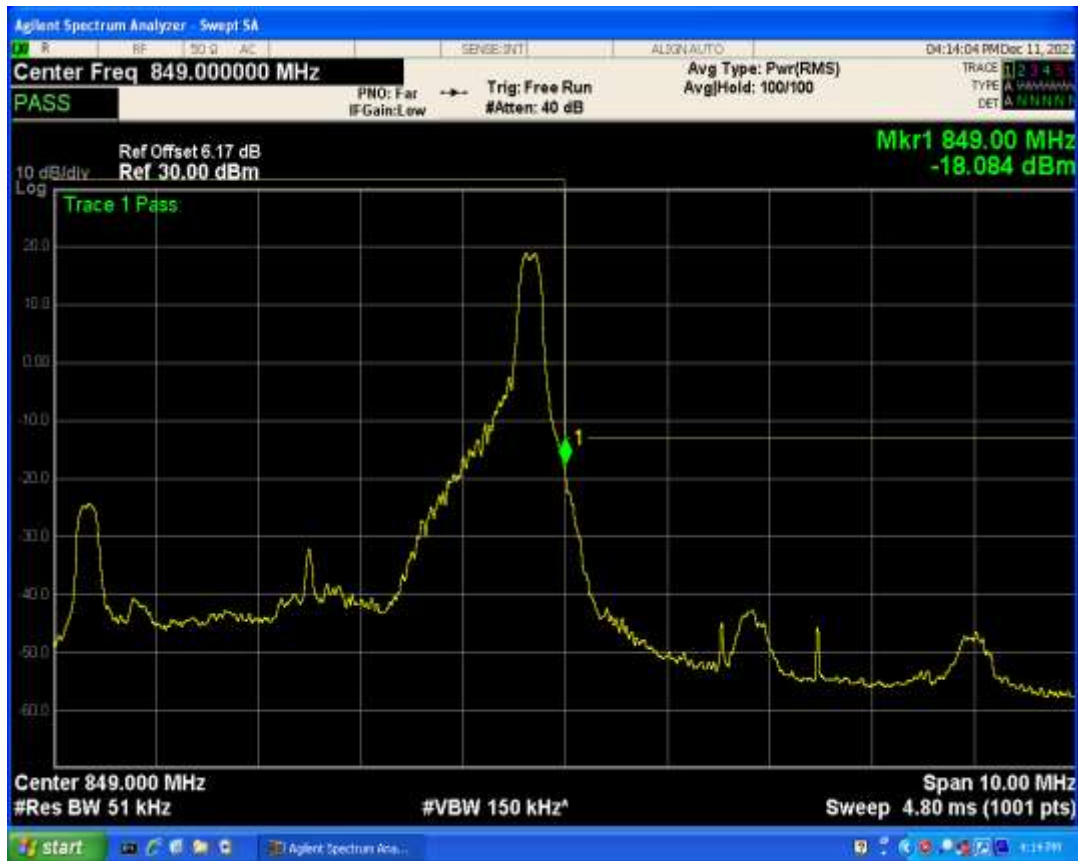
Band5 QPSK BW=5MHz Channel=20625 RB Size=25 Position=#0
