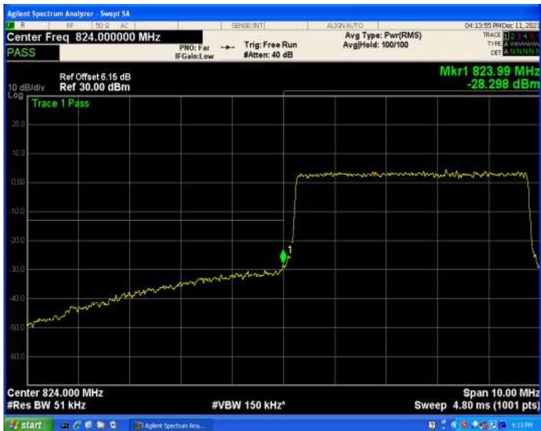
Band5 QAM16 BW=5MHz Channel=20425 RB Size=1 Position=#Max
