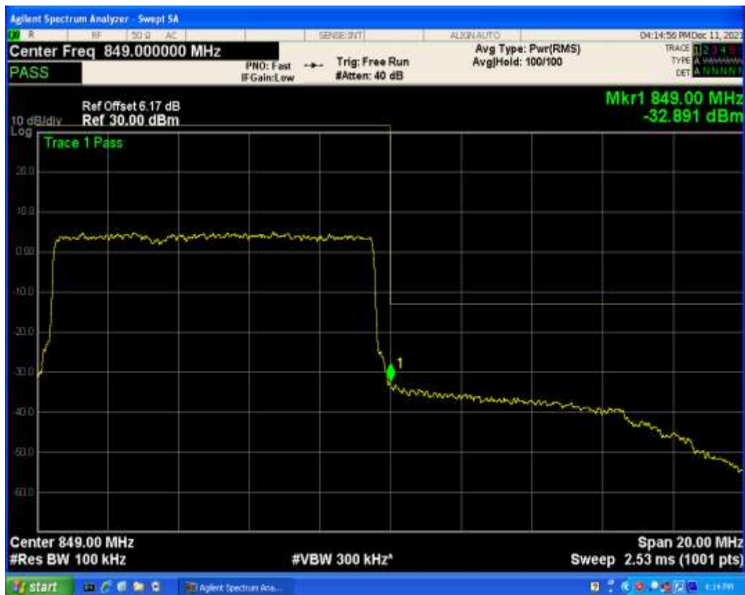
Band5 QAM16 BW=10MHz Channel=20600 RB Size=1 Position=#Max
