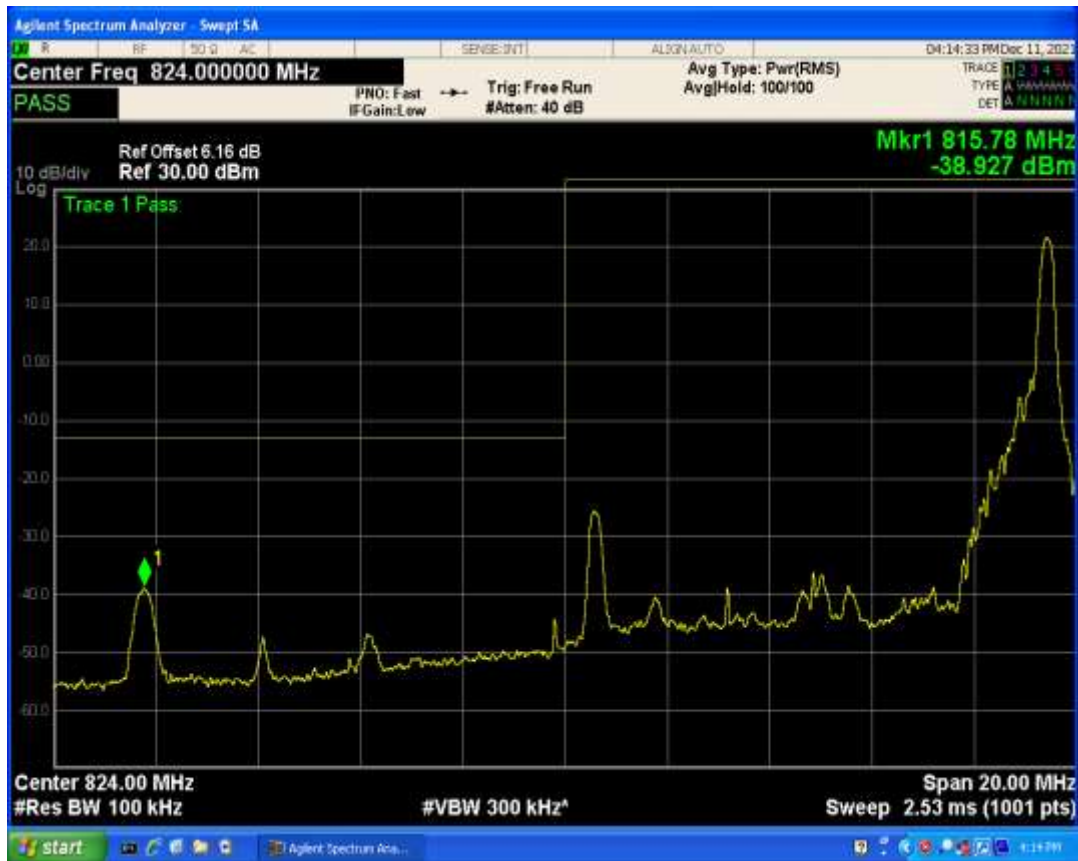
Band5 QPSK BW=10MHz Channel=20450 RB Size=50 Position=#0
