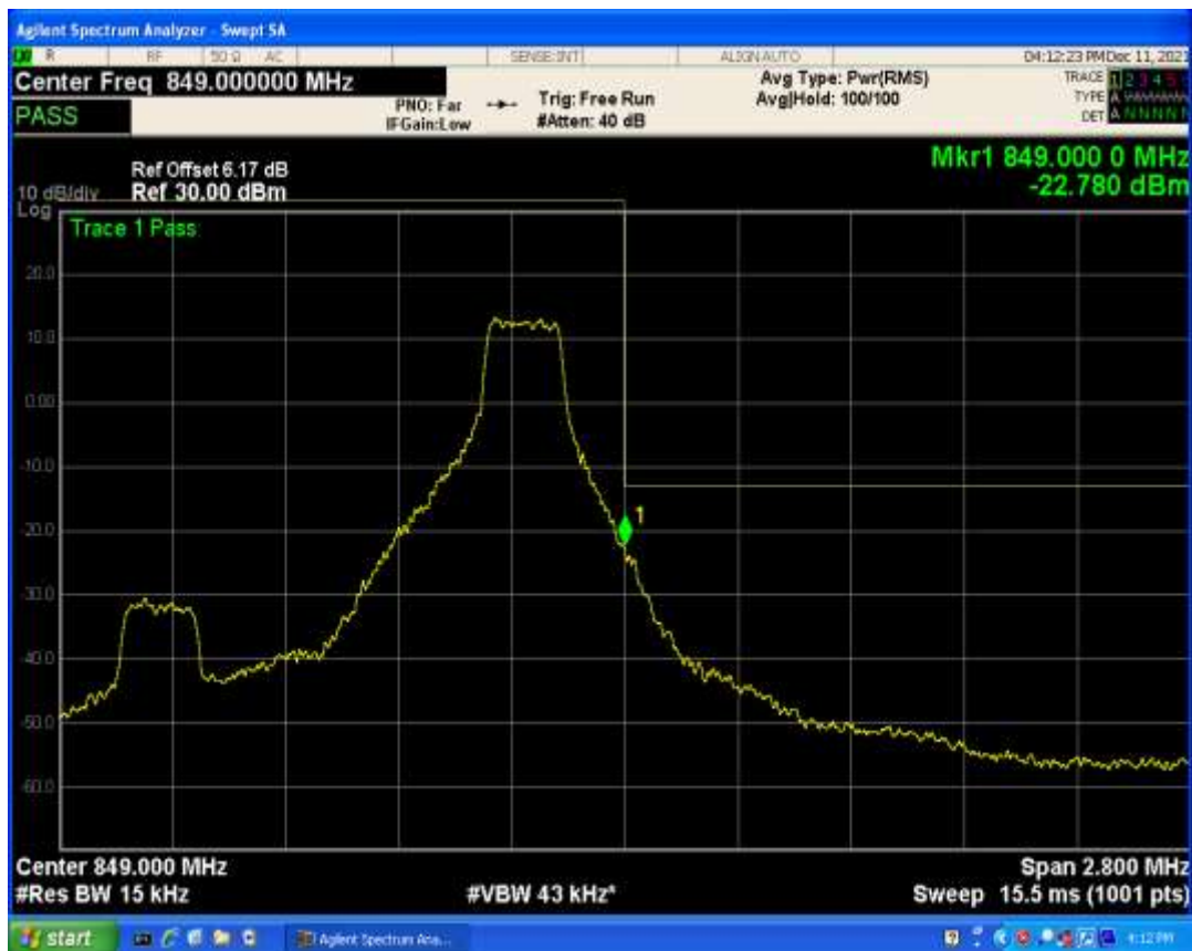
Band5 QAM16 BW=1.4MHz Channel=20643 RB Size=6 Position=#0
