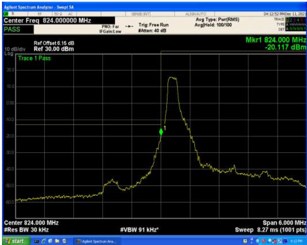
Band5 QAM16 BW=3MHz Channel=20415 RB Size=1 Position=#Max
