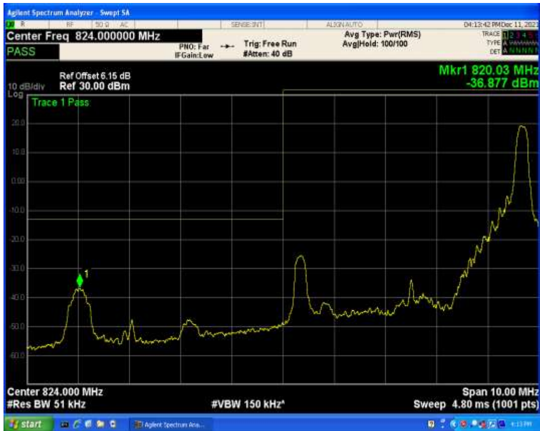
Band5 QPSK BW=5MHz Channel=20425 RB Size=25 Position=#0
