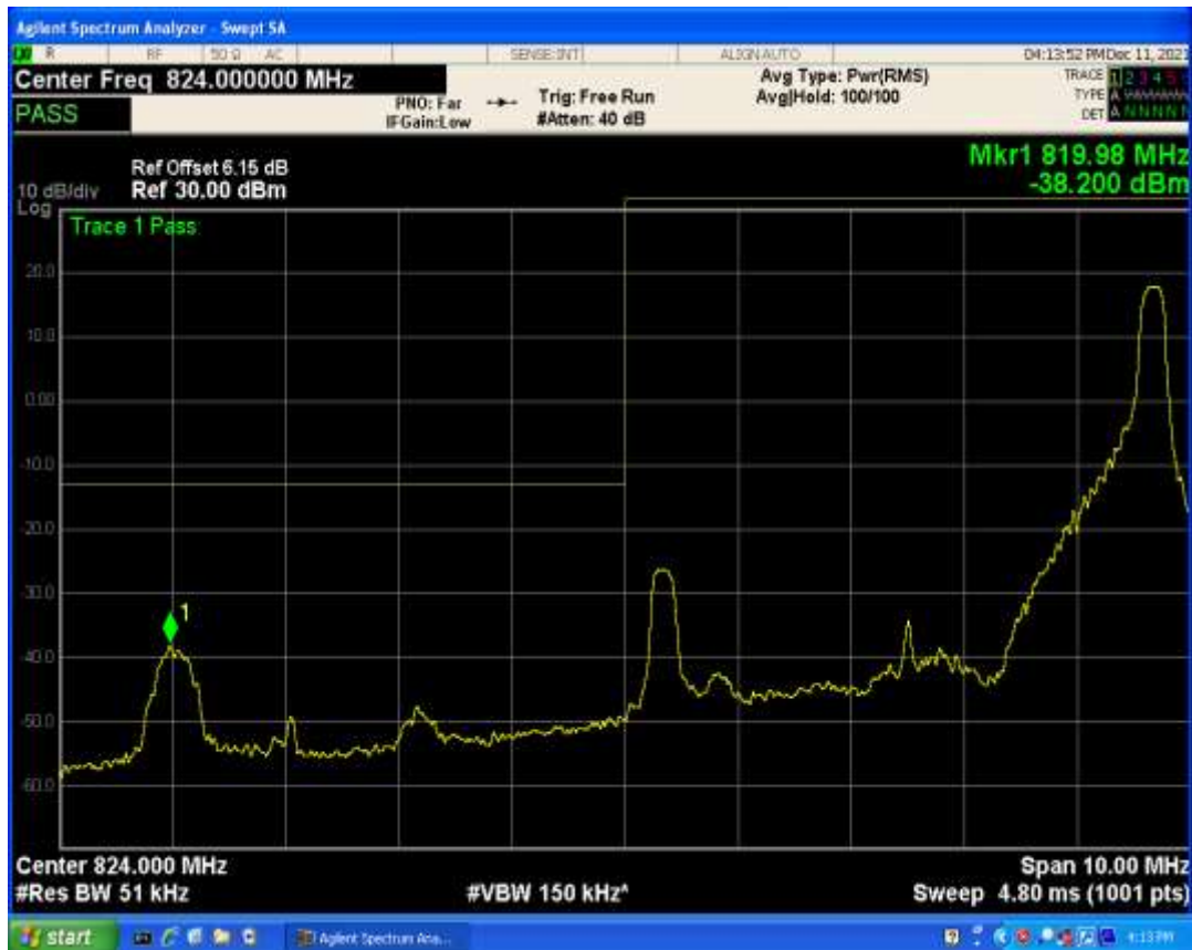
Band5 QPSK BW=5MHz Channel=20625 RB Size=1 Position=#0
