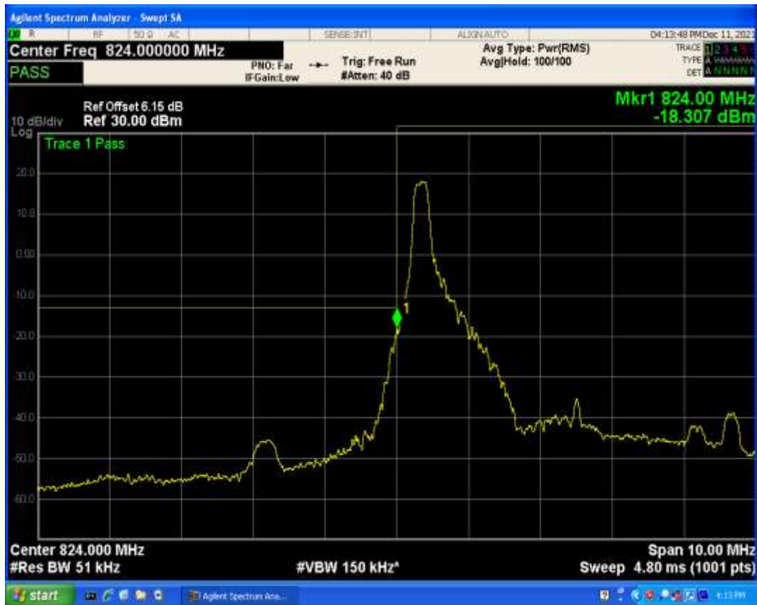
Band5 QAM16 BW=5MHz Channel=20425 RB Size=25 Position=#0
