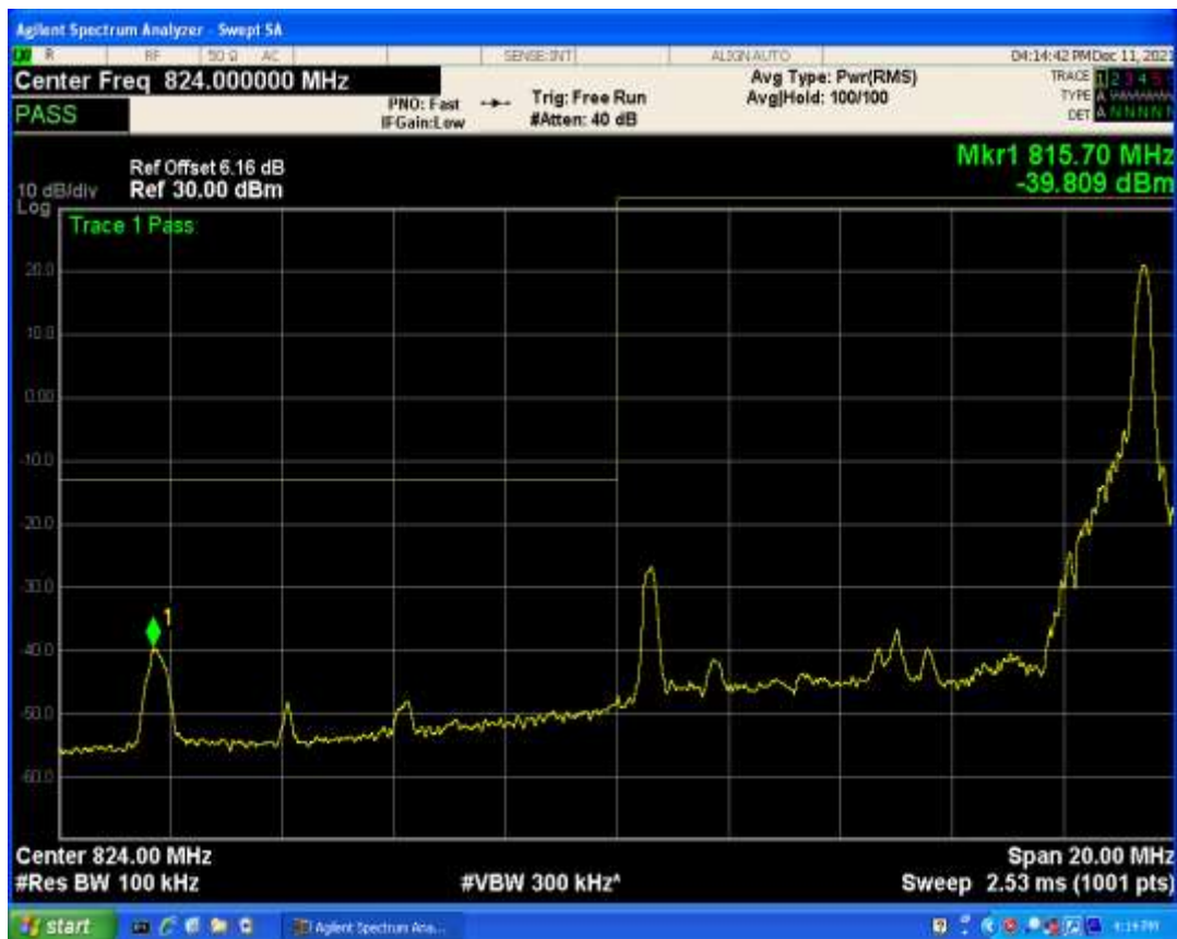
Band5 QAM16 BW=10MHz Channel=20450 RB Size=50 Position=#0
