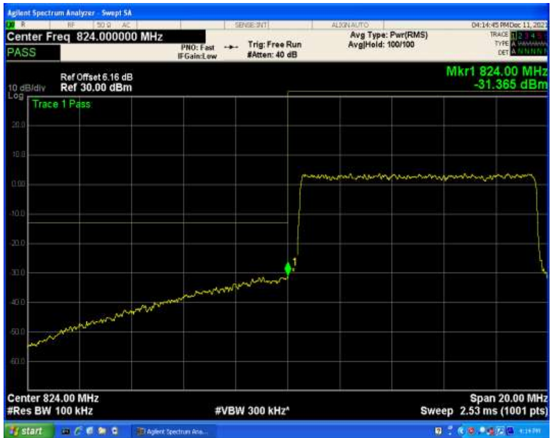
Band5 QPSK BW=10MHz Channel=20600 RB Size=1 Position=#0
