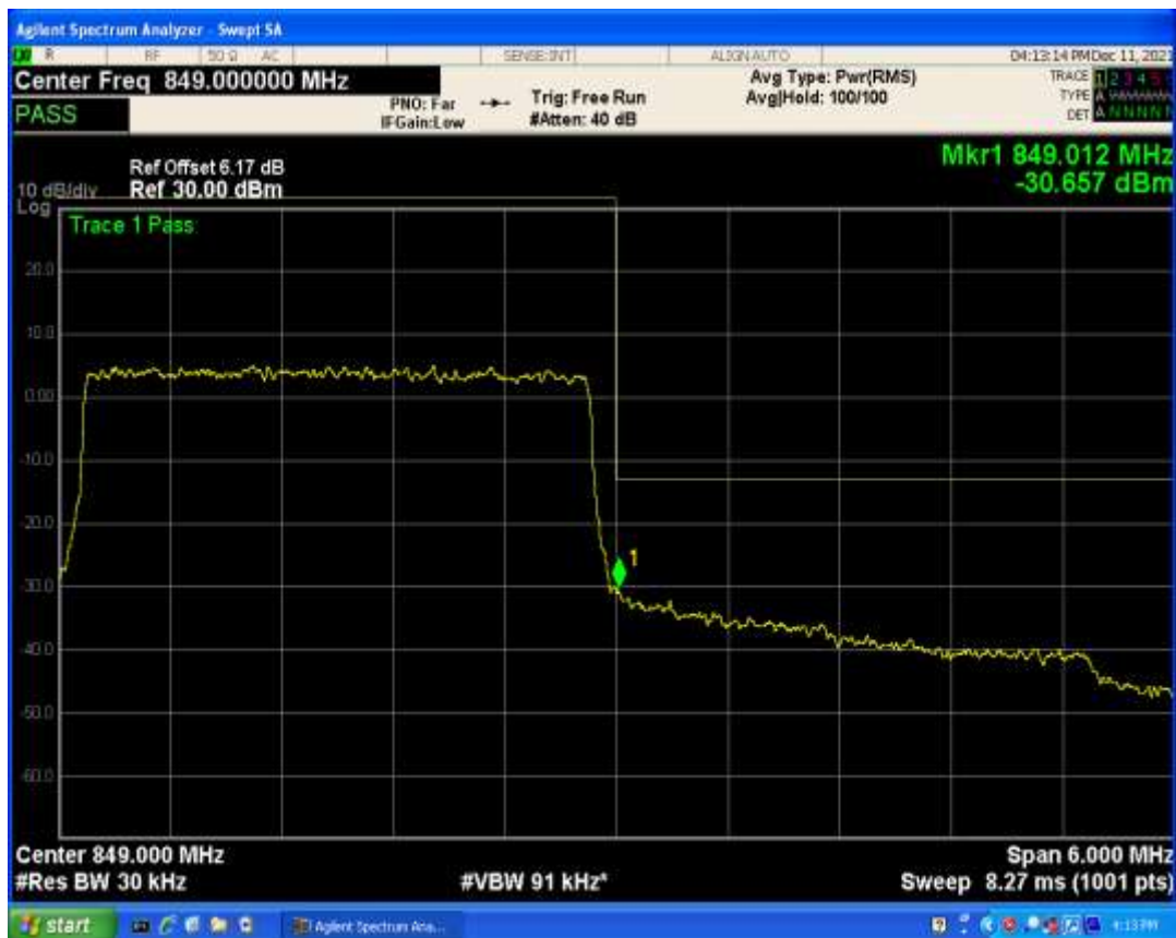
Band5 QAM16 BW=3MHz Channel=20635 RB Size=1 Position=#Max
