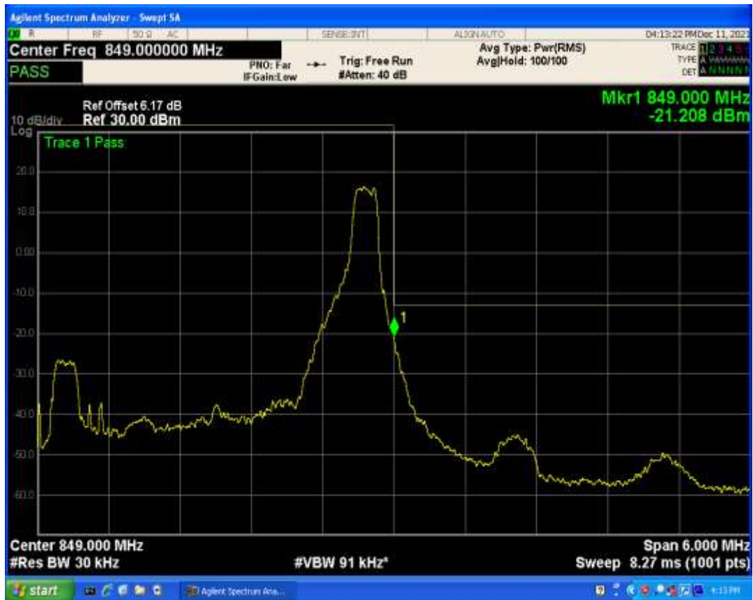
Band5 QAM16 BW=3MHz Channel=20635 RB Size=1 Position=#0
