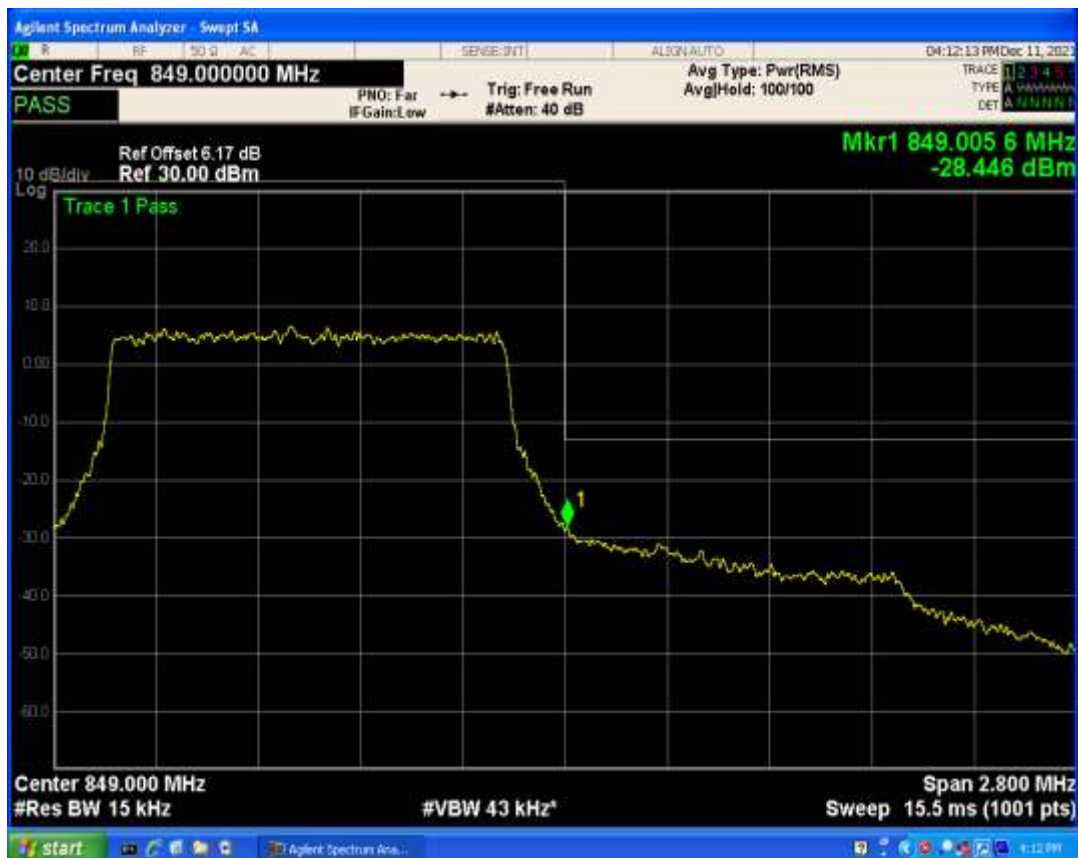
Band5 QAM16 BW=1.4MHz Channel=20643 RB Size=1 Position=#0
