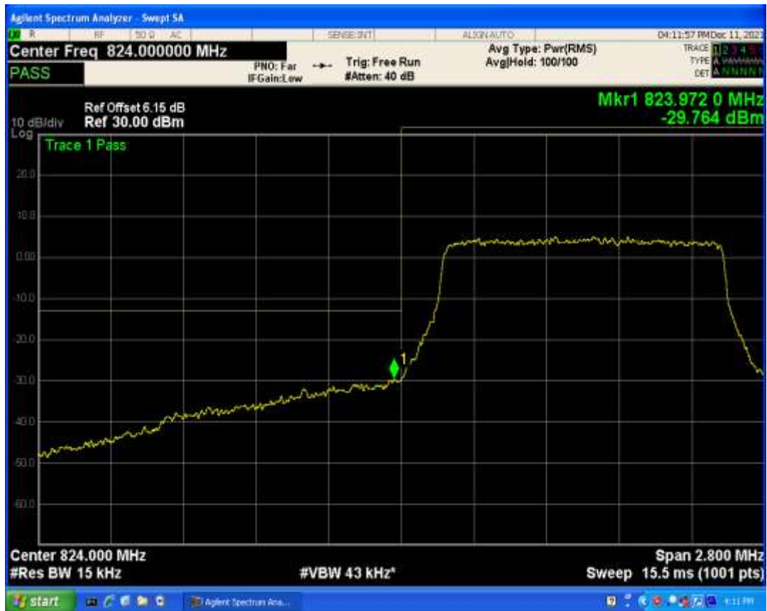
Band5 QPSK BW=1.4MHz Channel=20643 RB Size=1 Position=#0
