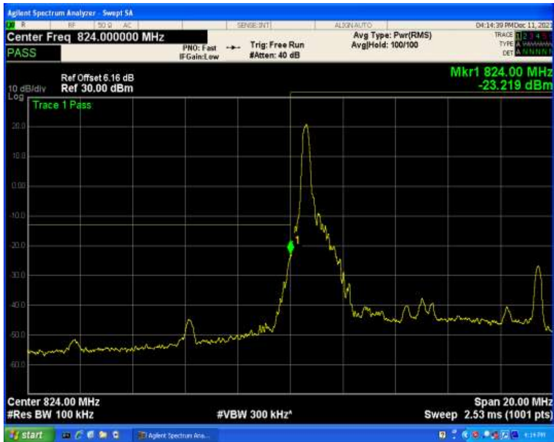
Band5 QAM16 BW=10MHz Channel=20450 RB Size=1 Position=#Max
