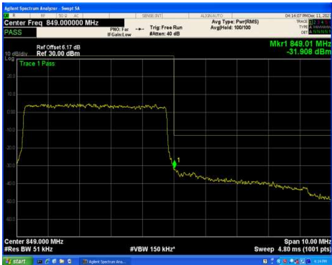
Band5 QAM16 BW=5MHz Channel=20625 RB Size=1 Position=#Max
