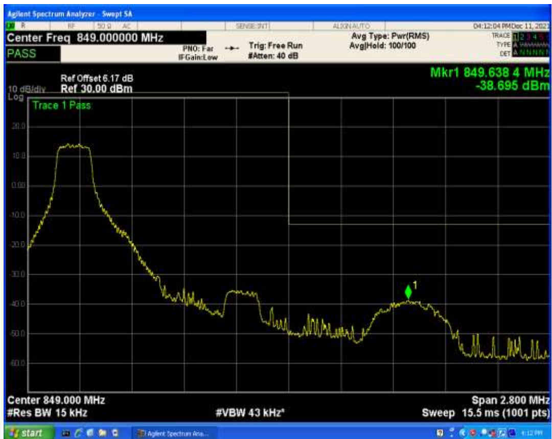
Band5 QPSK BW=1.4MHz Channel=20643 RB Size=1 Position=#Max
