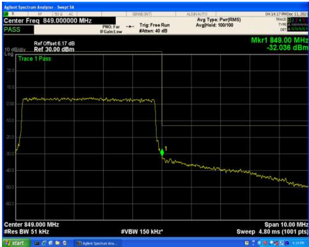
Band5 QPSK BW=10MHz Channel=20450 RB Size=1 Position=#0
