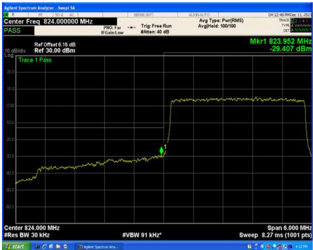
Band5 QAM16 BW=3MHz Channel=20415 RB Size=1 Position=#0
