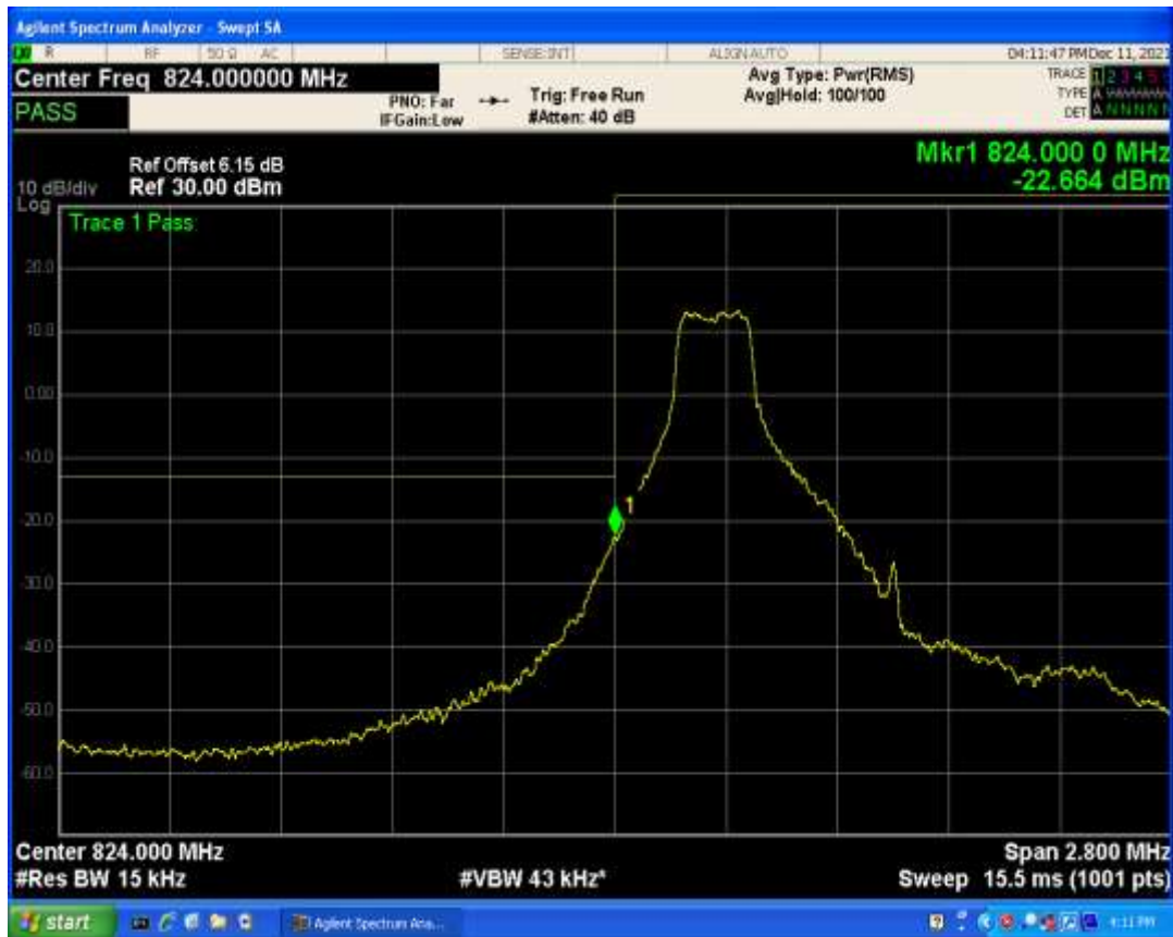
Band5 QAM16 BW=1.4MHz Channel=20407 RB Size=1 Position=#Max
