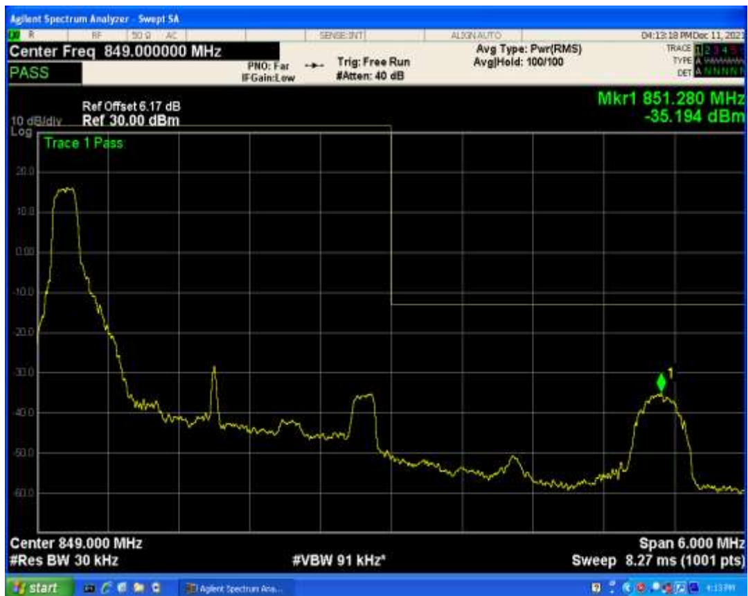
Band5 QAM16 BW=3MHz Channel=20635 RB Size=15 Position=#0
