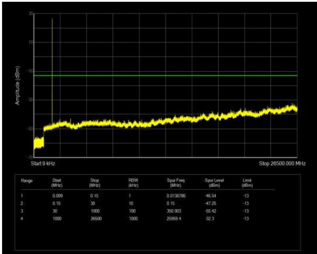
Band2 QAM16 BW=1.4MHz Channel=18607 RB Size=1 Position=#0
