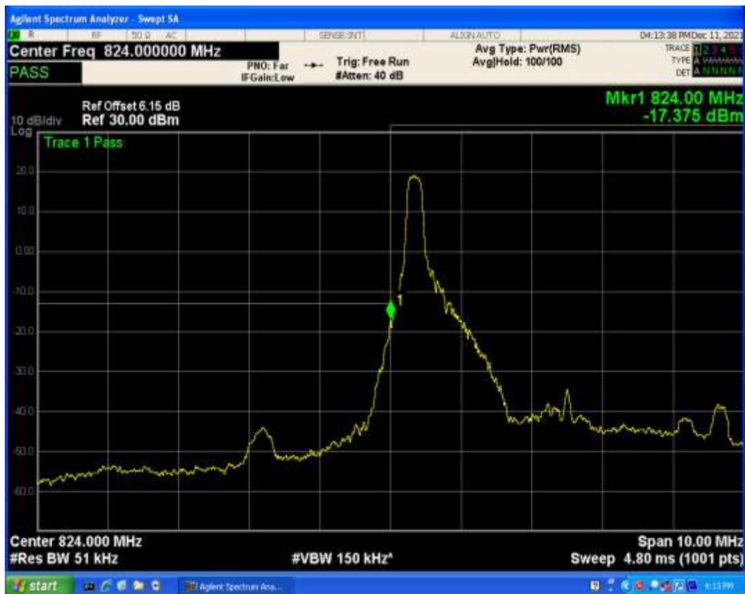
Band5 QPSK BW=5MHz Channel=20425 RB Size=1 Position=#Max
