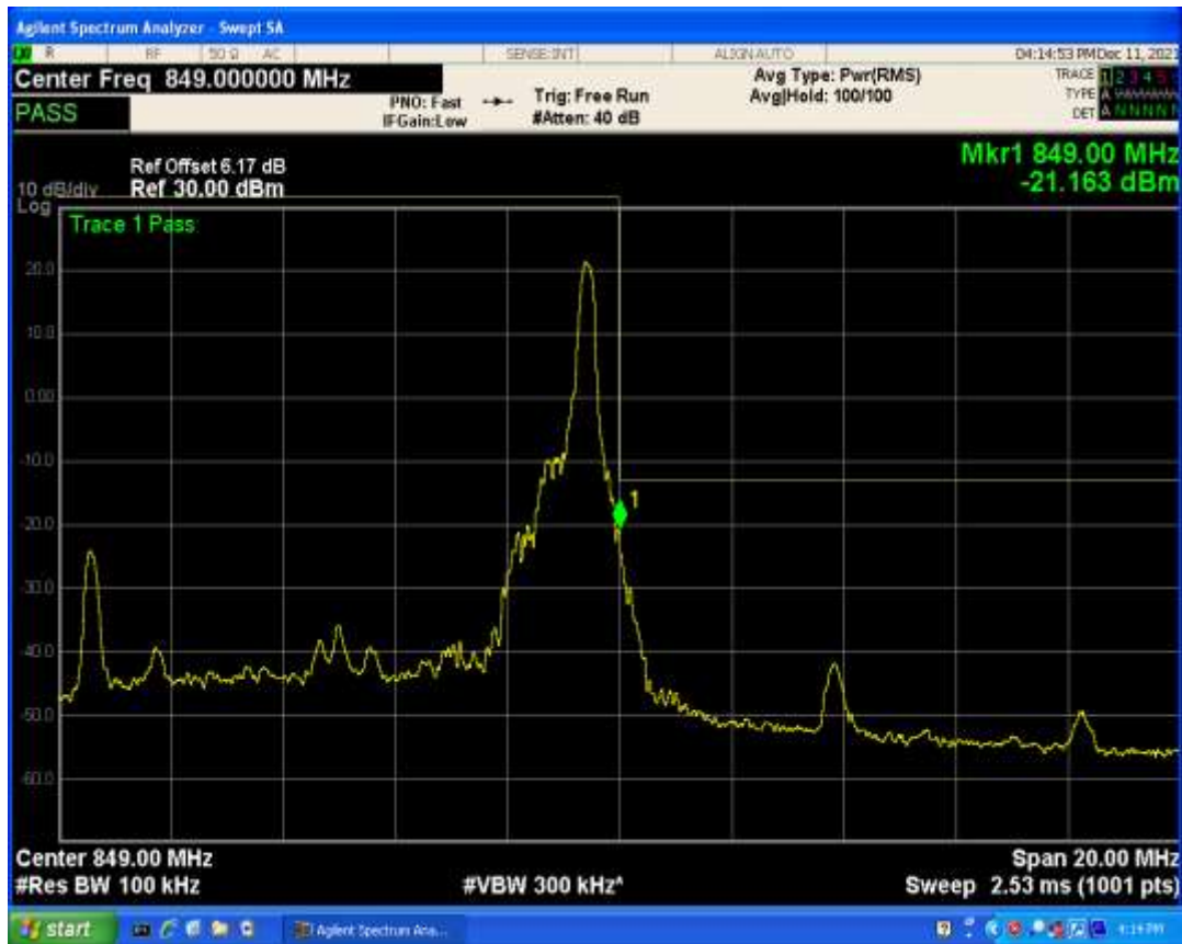
Band5 QPSK BW=10MHz Channel=20600 RB Size=50 Position=#0
