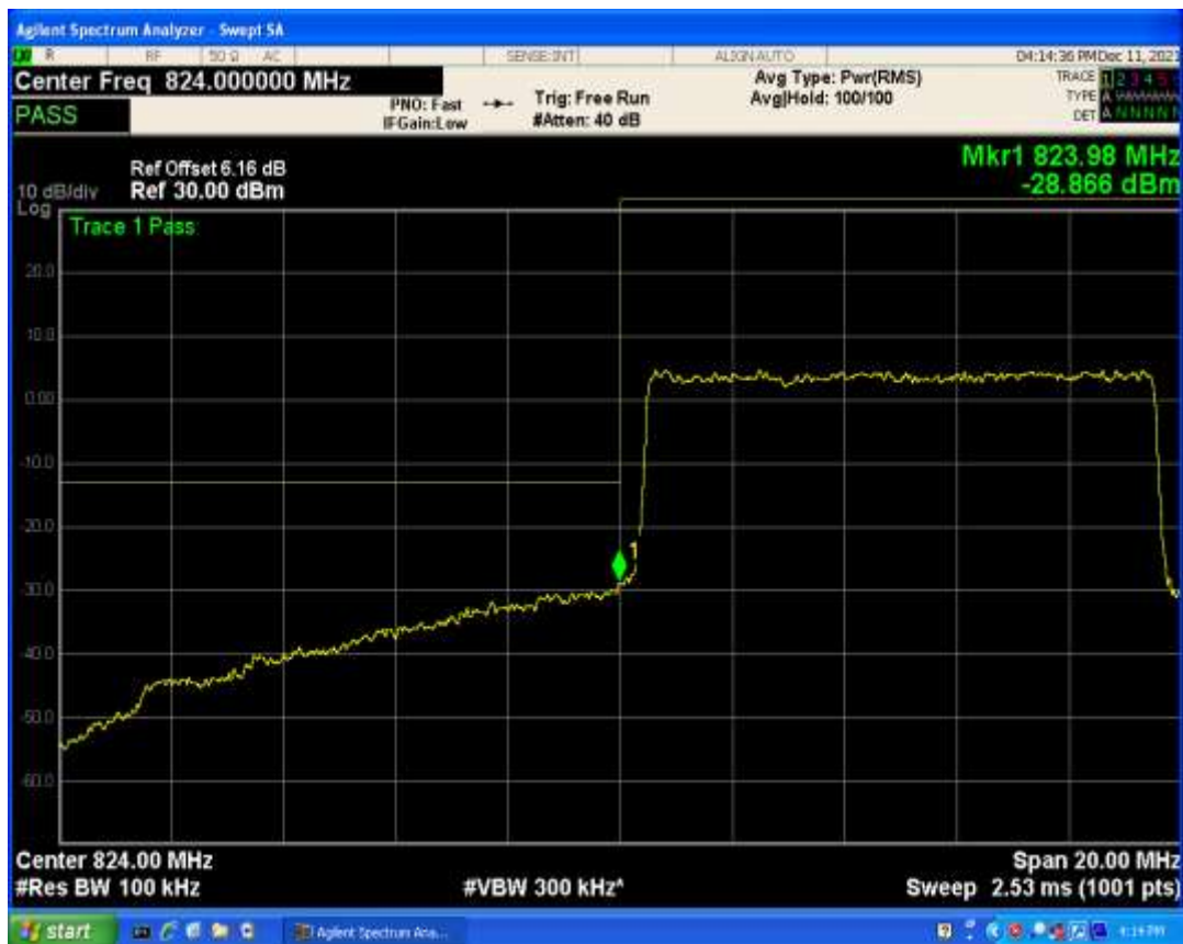
Band5 QAM16 BW=10MHz Channel=20450 RB Size=1 Position=#0
