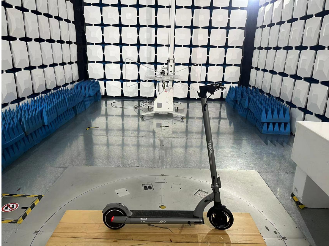
Above 1GHz for radiated emission test setup
