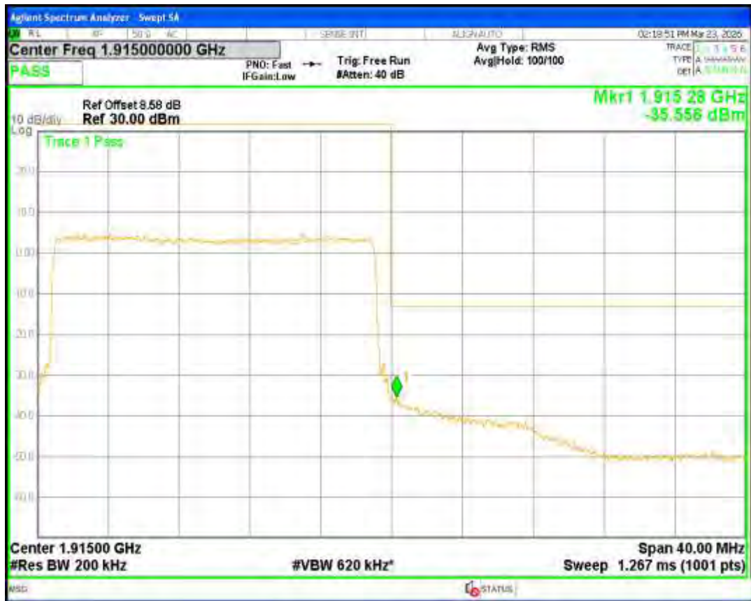
Band25 QPSK BW=3MHz Channel=26055 RB Size=15 Position=#0
