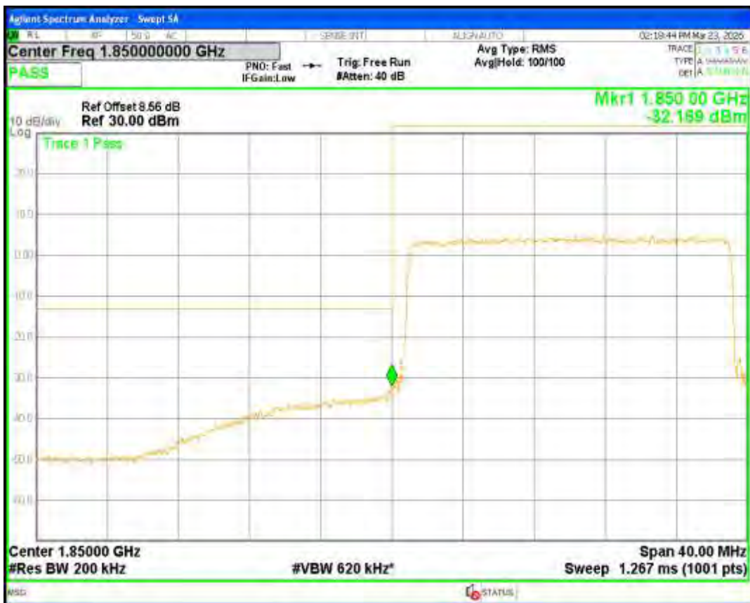
Band25 QPSK BW=20MHz Channel=26590 RB Size=100 Position=#0
