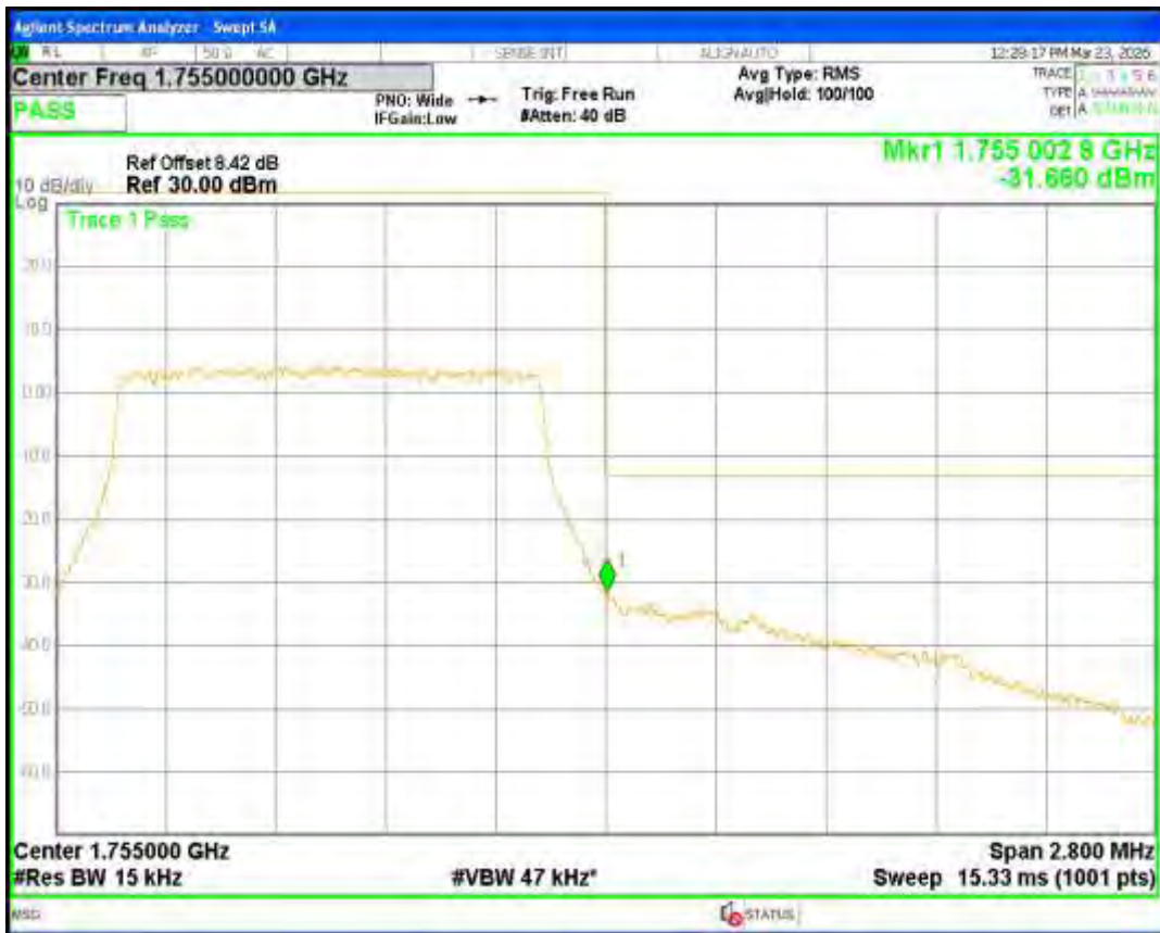
Band4 16QAM BW=10MHz Channel=20000 RB Size=50 Position=#0
