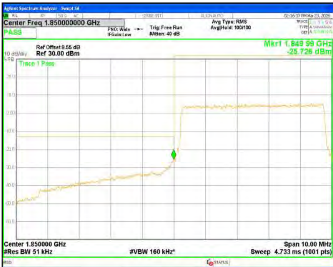
Band25 QPSK BW=5MHz Channel=26665 RB Size=25 Position=#0
