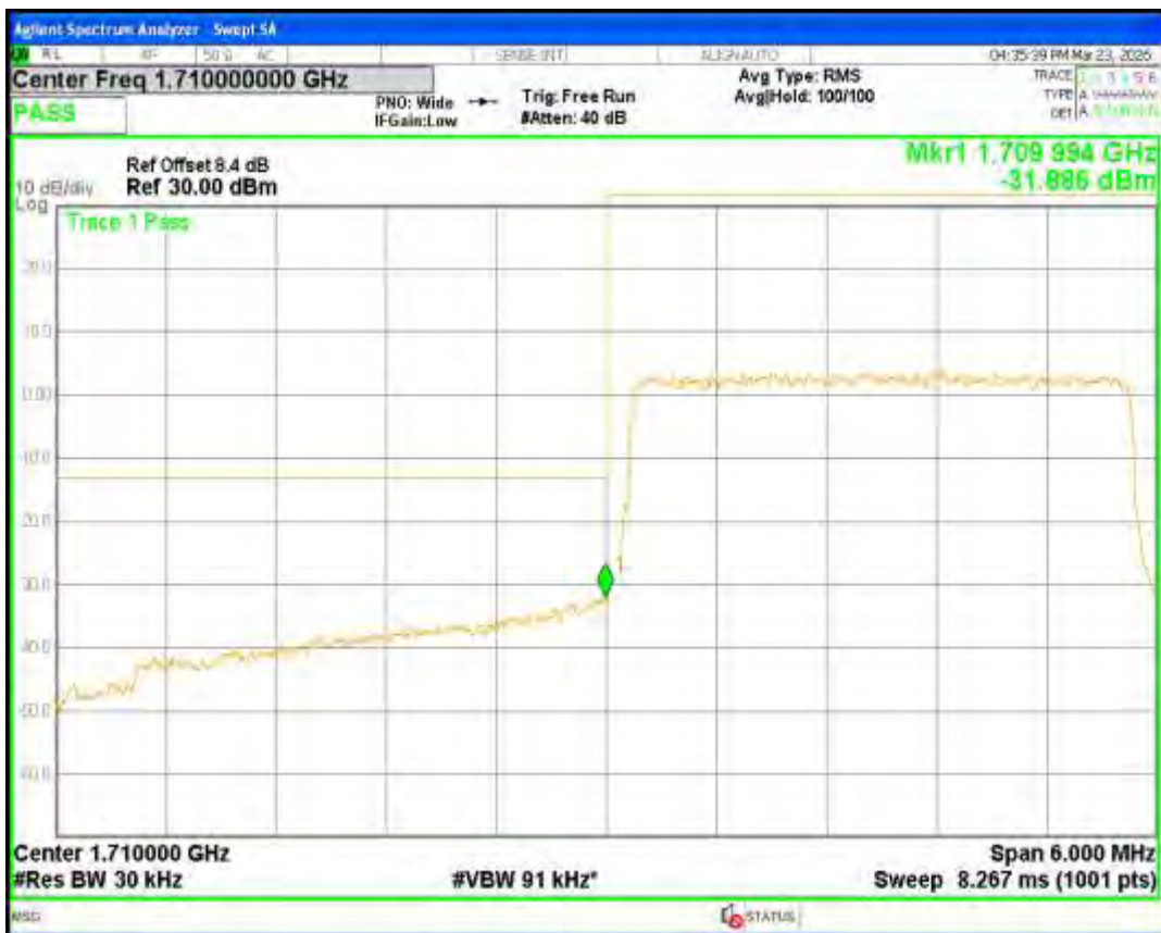
Band66 QPSK BW=3MHz Channel=132657 RB Size=15 Position=#0
