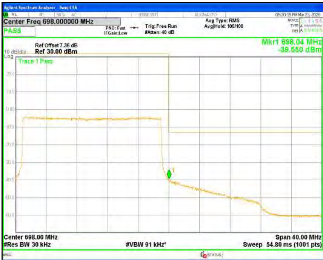
Band71 16QAM BW=5MHz Channel=133147 RB Size=25 Position=#0
