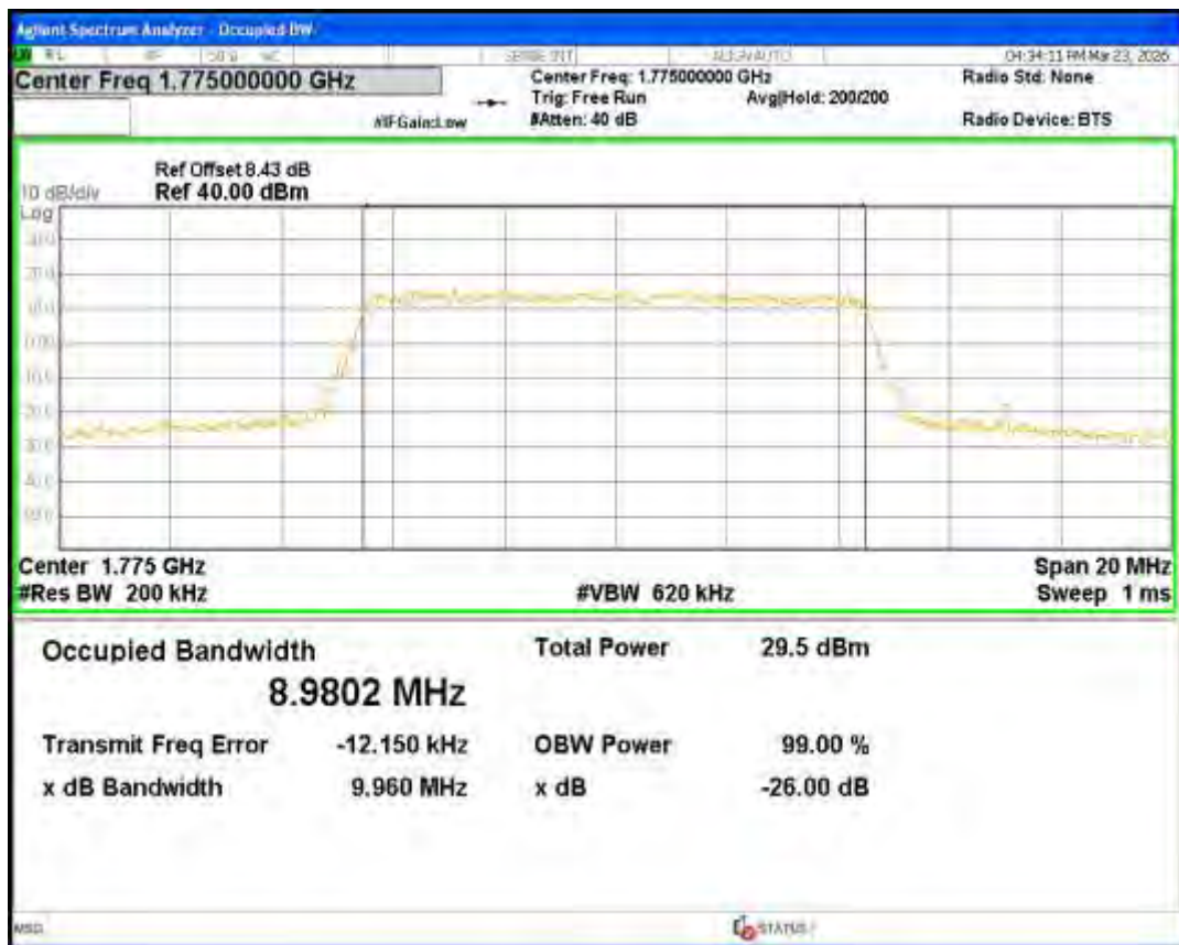
Band66 QPSK BW=15MHz Channel=132047 RB Size=75 Position=#0
