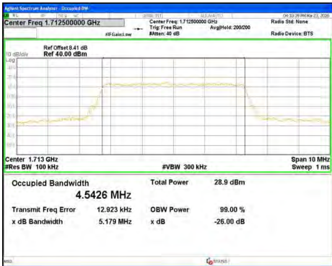
Band66 QPSK BW=1.4MHz Channel=132665 RB Size=6 Position=#0
