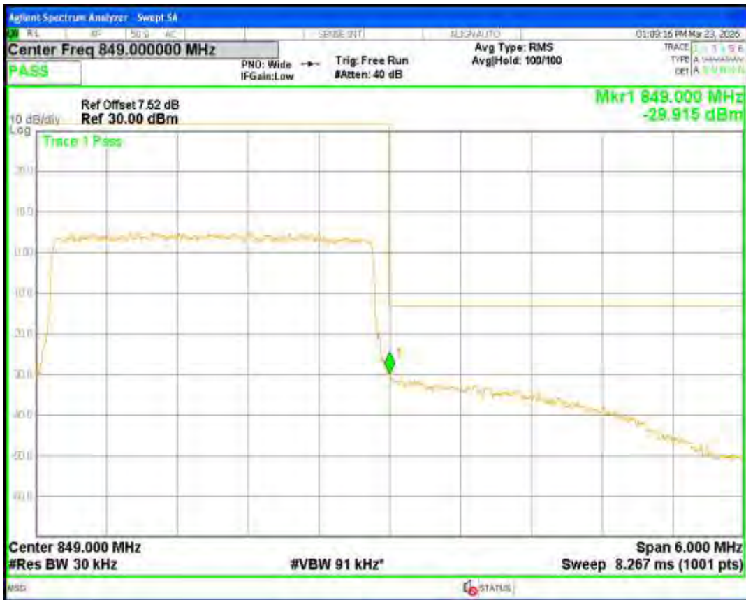
Band5 QPSK BW=5MHz Channel=20425 RB Size=25 Position=#0
