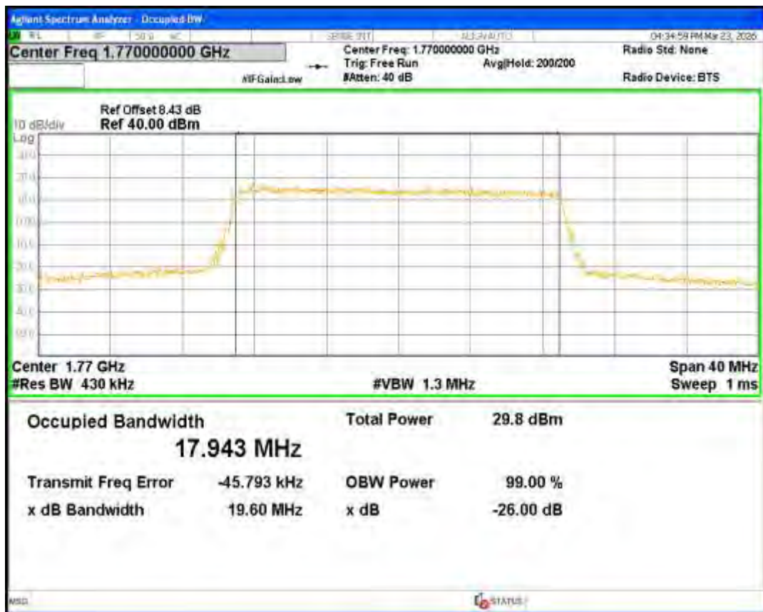
Band66 QPSK BW=3MHz Channel=131987 RB Size=15 Position=#0
