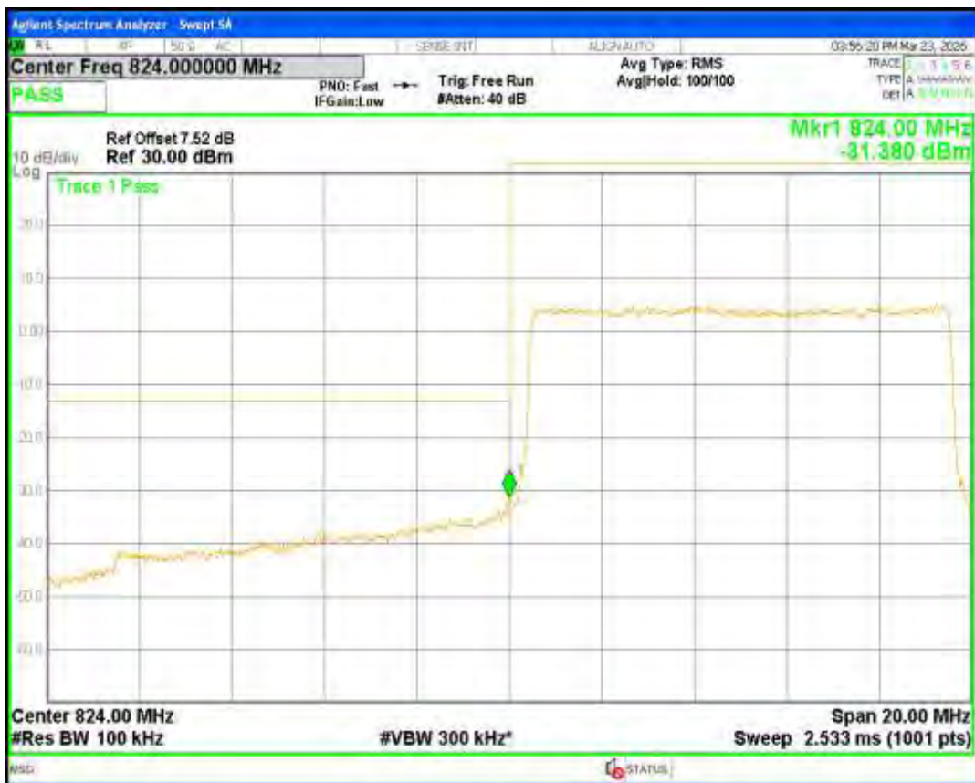
Band26(824-849) QPSK BW=10MHz Channel=26990 RB Size=50 Position=#0
