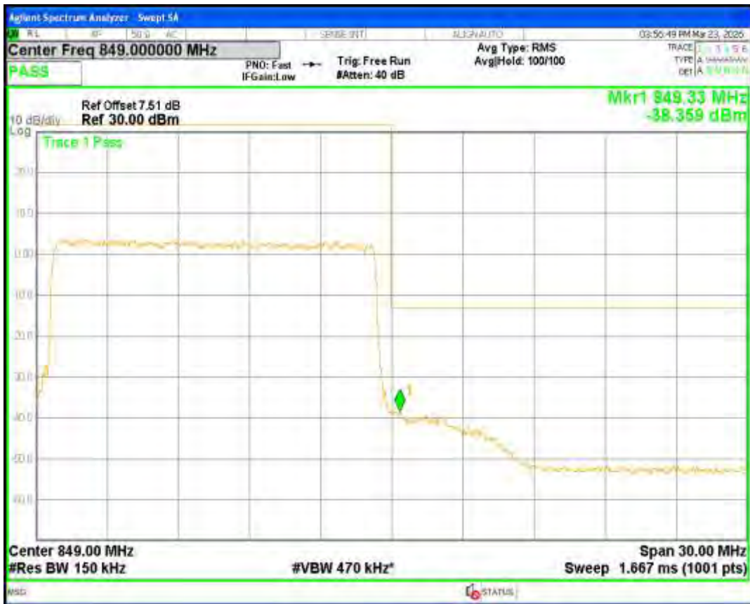
Band26(824-849) 16QAM BW=3MHz Channel=26805 RB Size=15 Position=#0
