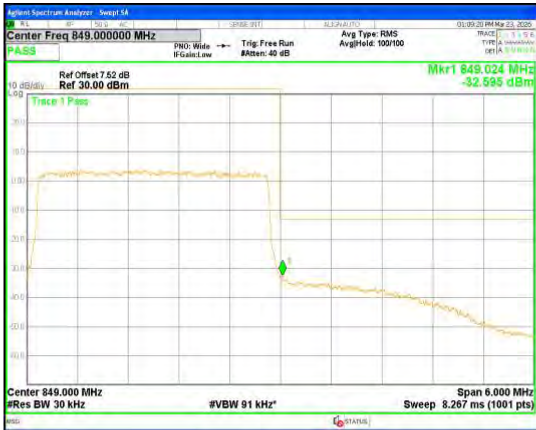
Band5 16QAM BW=5MHz Channel=20425 RB Size=25 Position=#0
