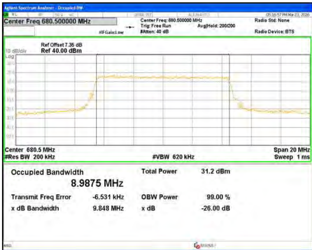
Band71 QPSK BW=10MHz Channel=133422 RB Size=50 Position=#0
