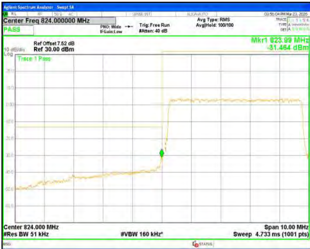
Band26(824-849) QPSK BW=10MHz Channel=26840 RB Size=50 Position=#0
