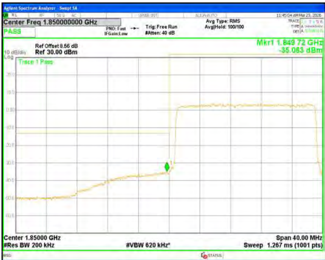
Band2 16QAM BW=5MHz Channel=18625 RB Size=25 Position=#0
