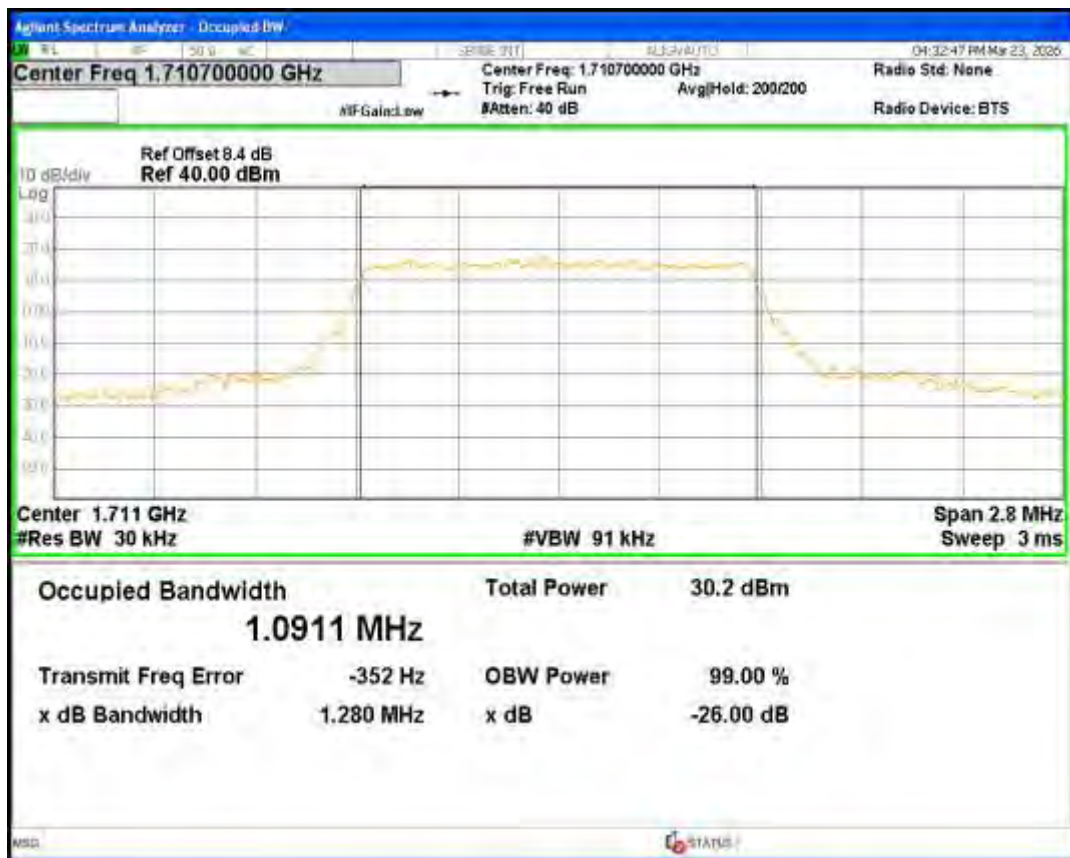
Band66 QPSK BW=10MHz Channel=132322 RB Size=50 Position=#0
