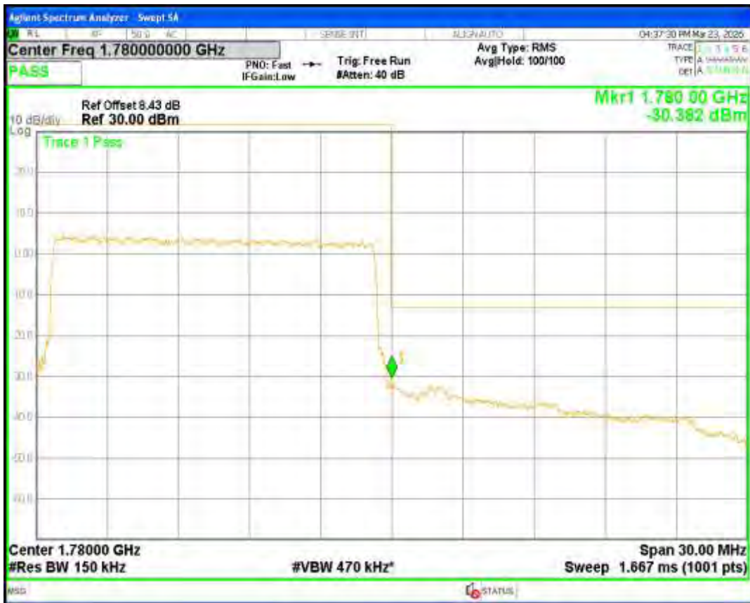
Band66 QPSK BW=20MHz Channel=132072 RB Size=100 Position=#0
