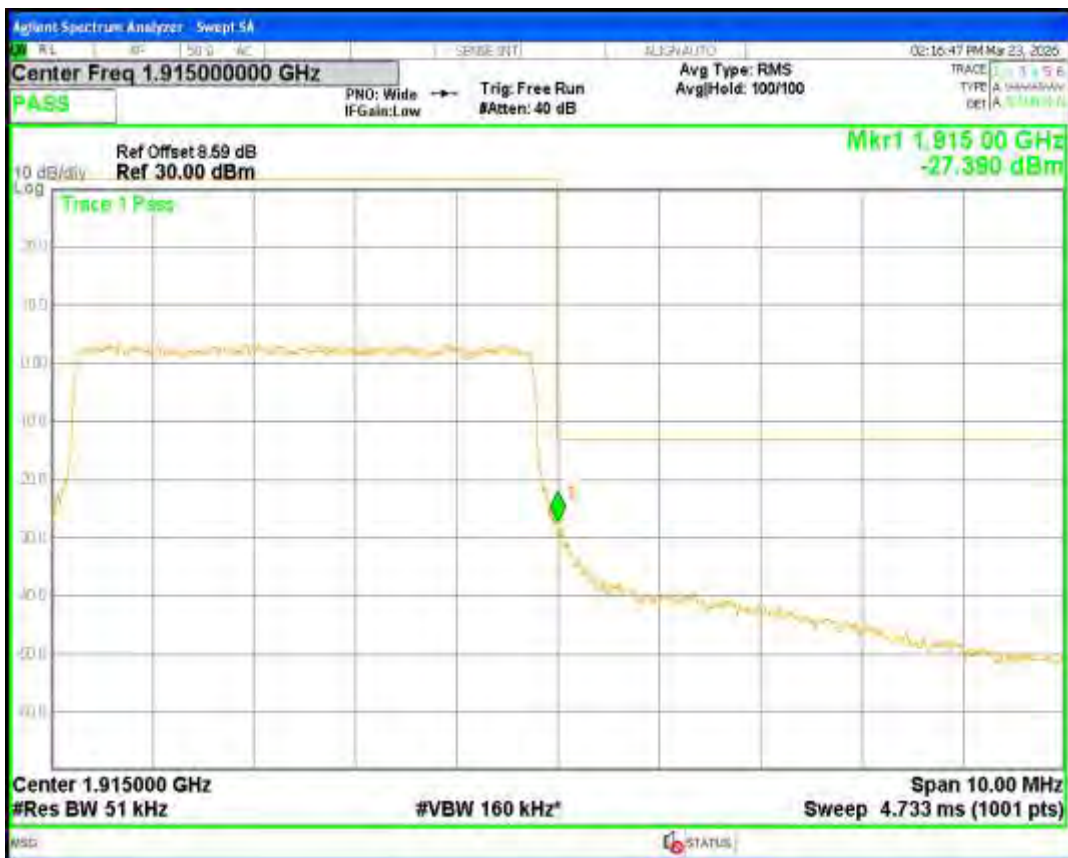
Band25 16QAM BW=5MHz Channel=26065 RB Size=25 Position=#0
