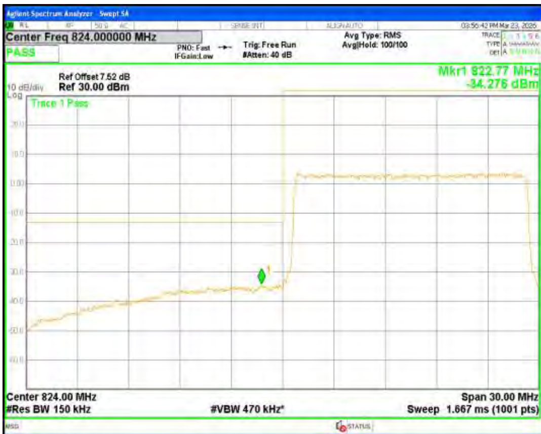
Band26(824-849) 16QAM BW=15MHz Channel=26965 RB Size=75 Position=#0
