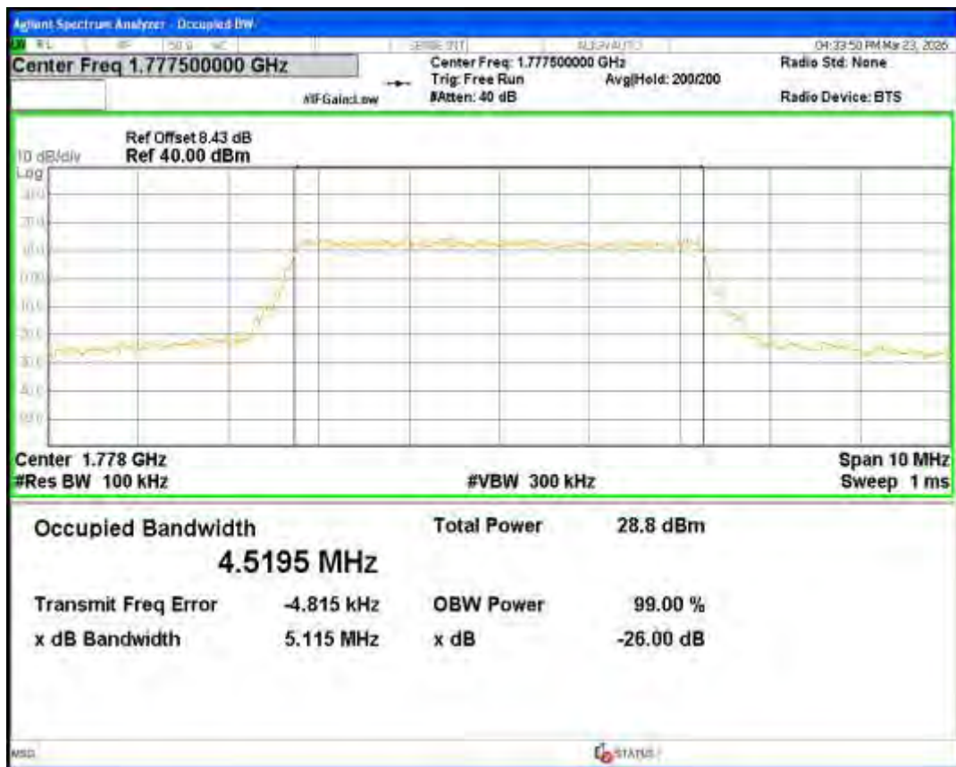
Band66 16QAM BW=5MHz Channel=132322 RB Size=25 Position=#0
