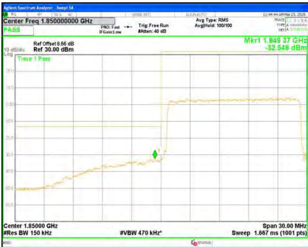
Band2 16QAM BW=15MHz Channel=19125 RB Size=75 Position=#0
