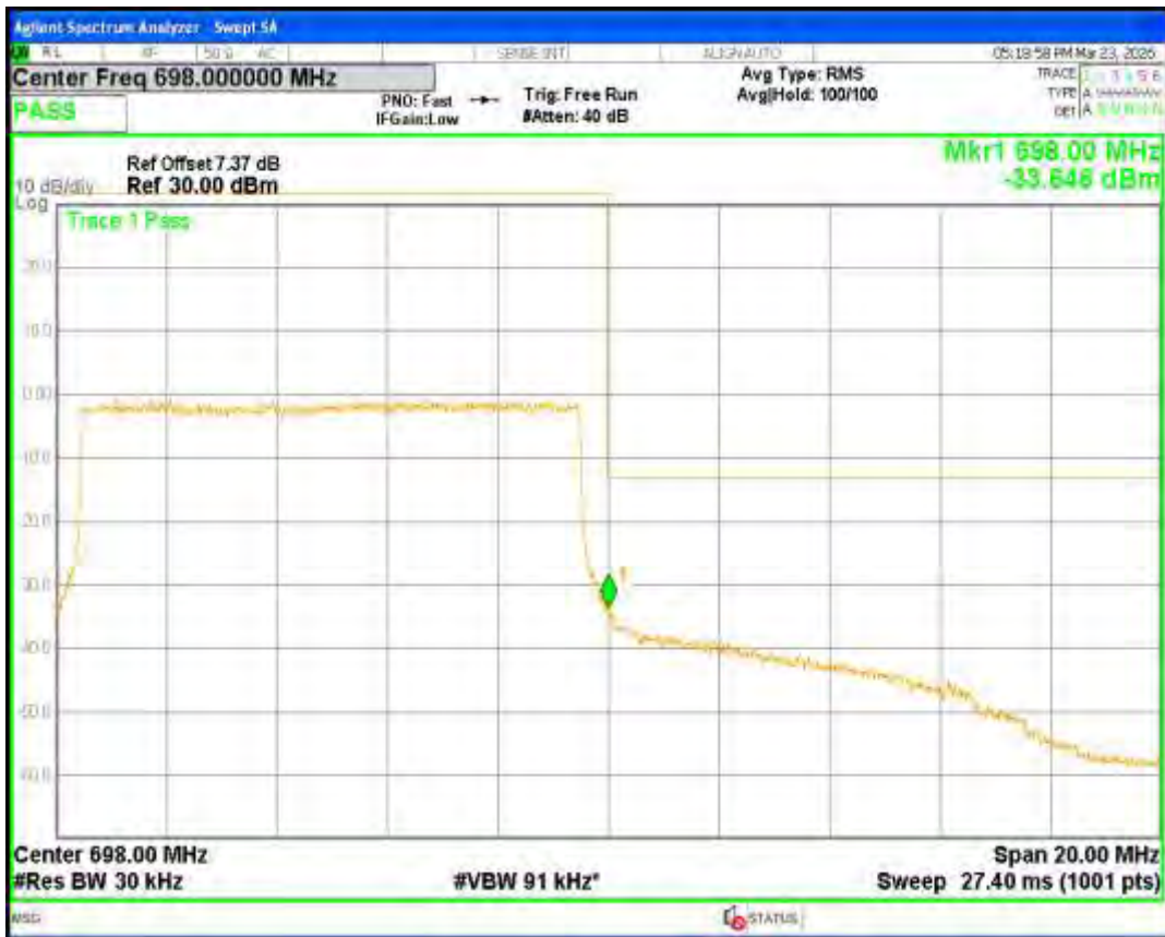
Band71 16QAM BW=15MHz Channel=133197 RB Size=75 Position=#0
