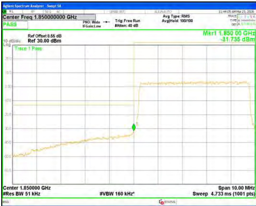
Band2 16QAM BW=3MHz Channel=19185 RB Size=15 Position=#0
