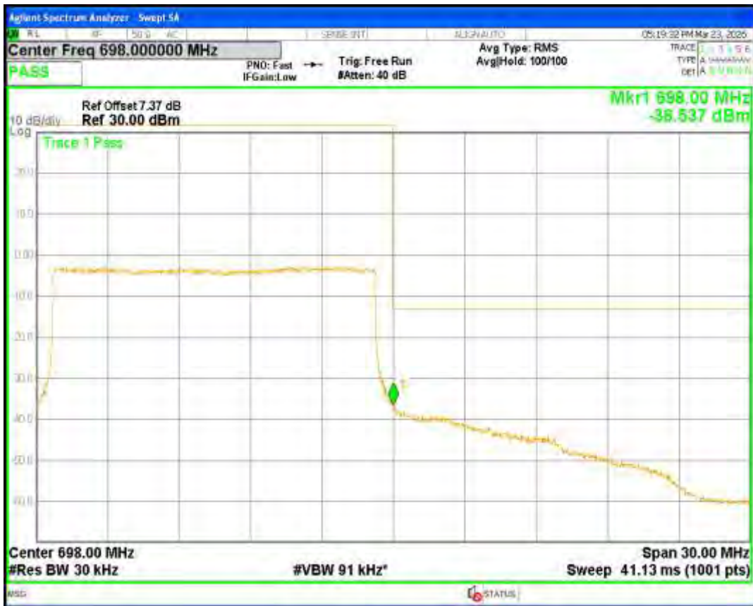
Band71 16QAM BW=20MHz Channel=133222 RB Size=100 Position=#0
