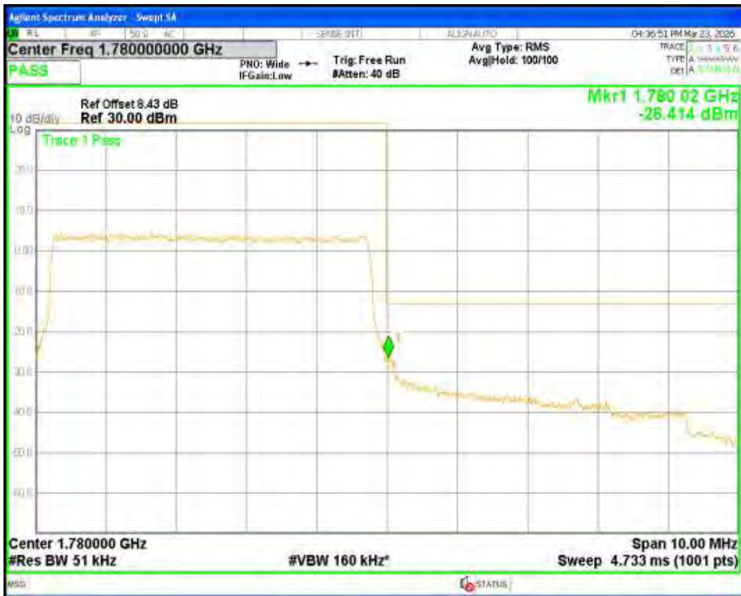
Band71 16QAM BW=10MHz Channel=133172 RB Size=50 Position=#0
