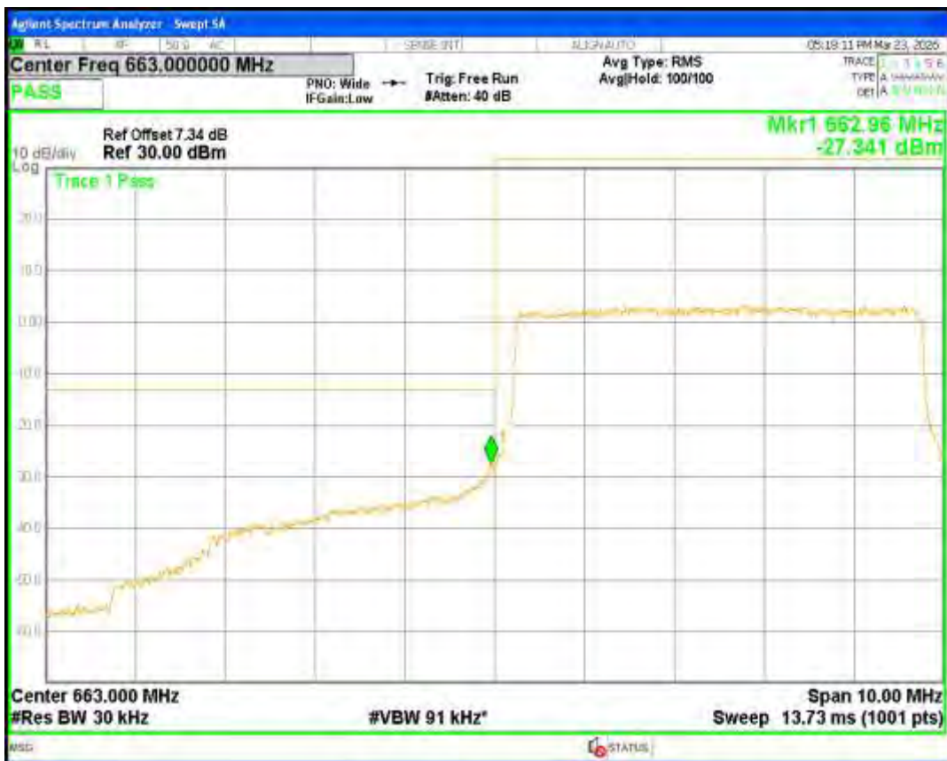
Band71 QPSK BW=5MHz Channel=133447 RB Size=25 Position=#0
