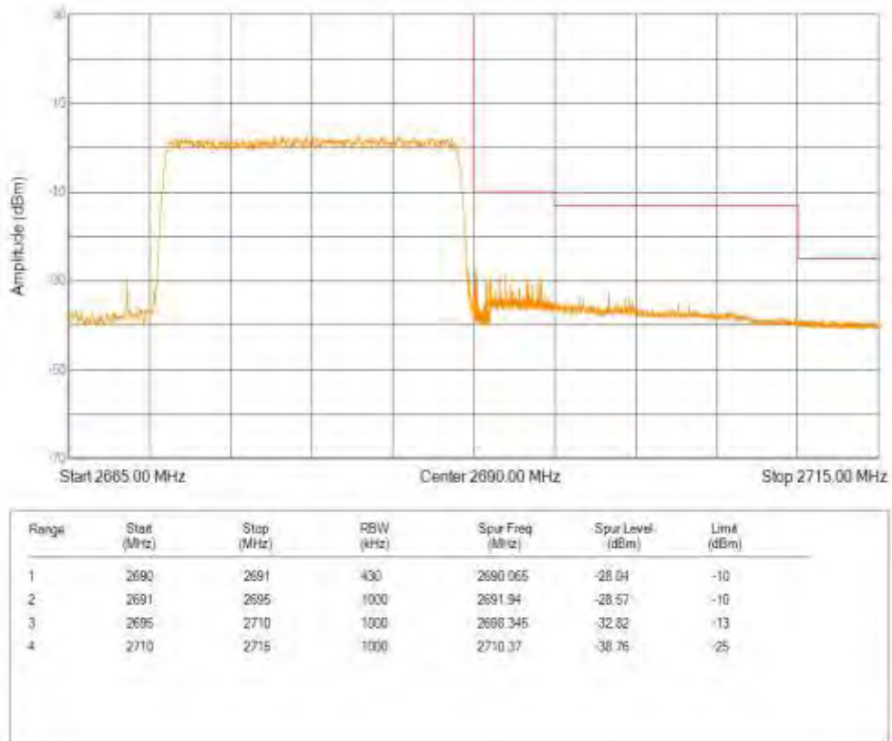
Band41 16QAM BW=5MHz Channel=39675 RB Size=25 Position=#0
