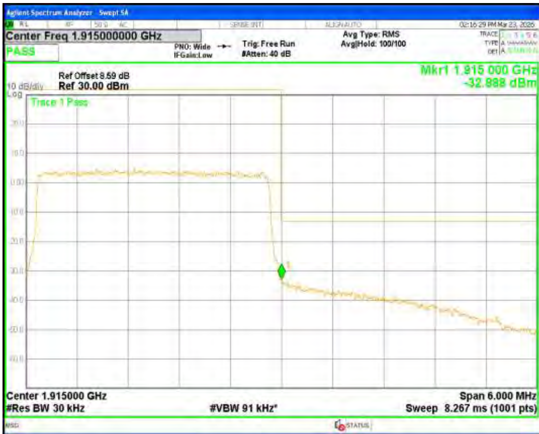
Band25 QPSK BW=5MHz Channel=26065 RB Size=25 Position=#0
