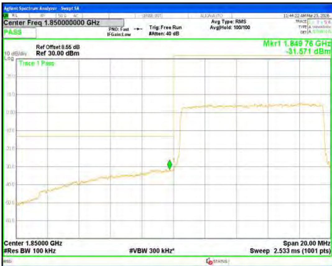
Band2 QPSK BW=10MHz Channel=19150 RB Size=50 Position=#0
