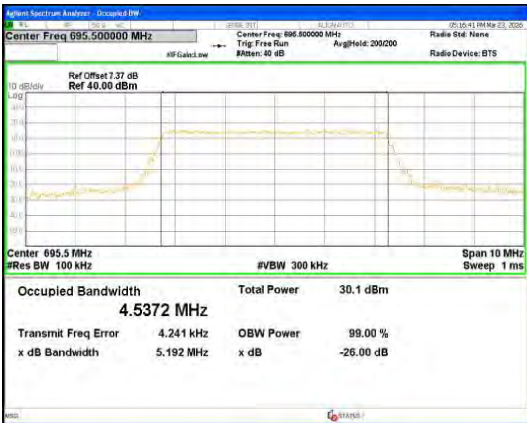
Band71 16QAM BW=20MHz Channel=133297 RB Size=100 Position=#0
