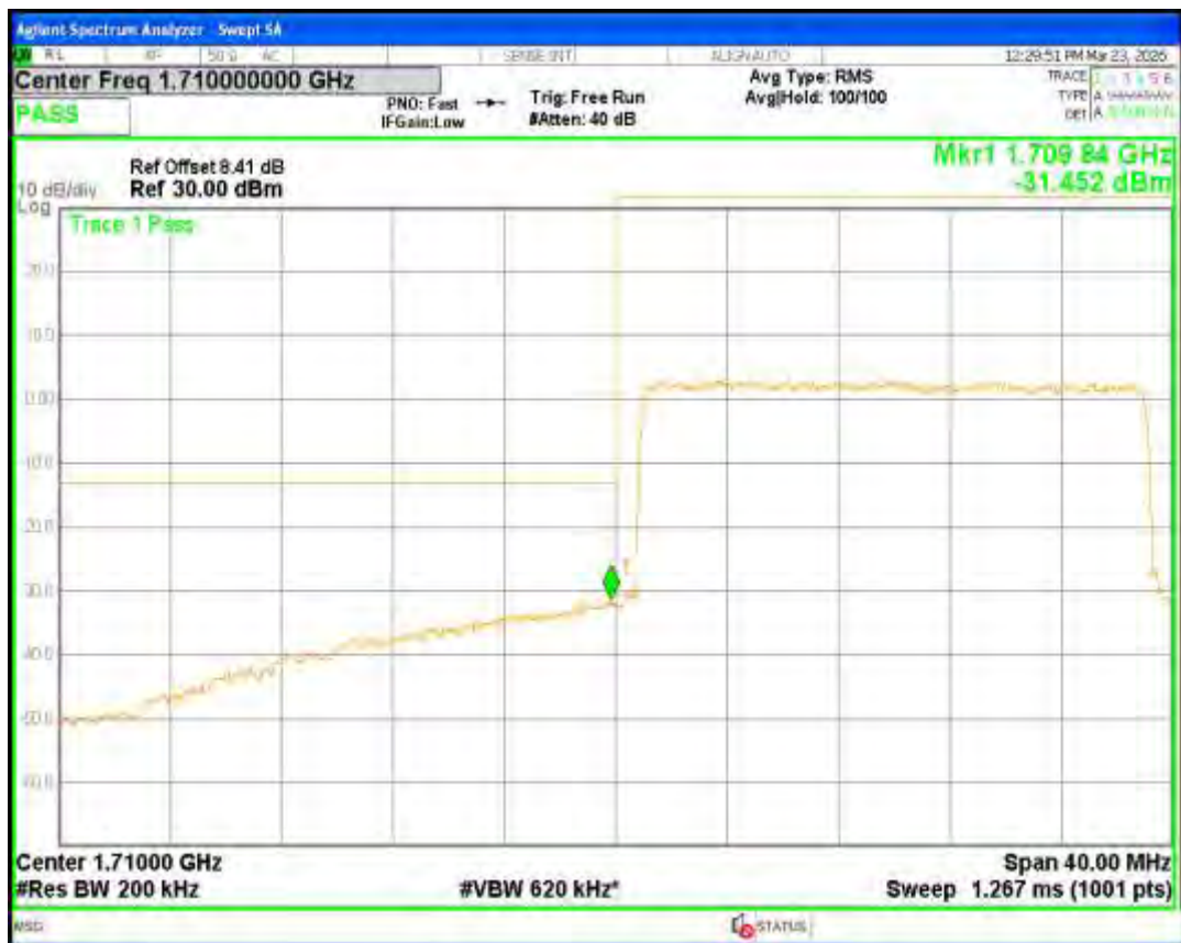
Band4 16QAM BW=20MHz Channel=20300 RB Size=100 Position=#0
