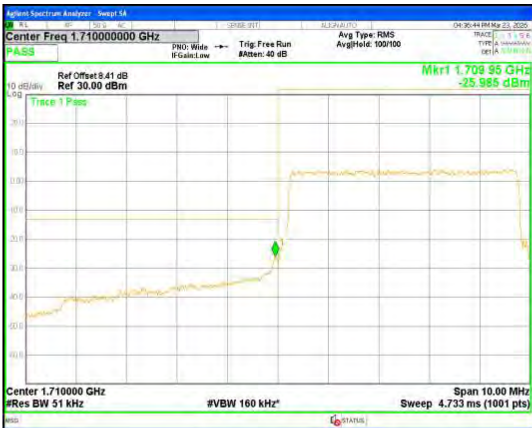
Band66 QPSK BW=5MHz Channel=132647 RB Size=25 Position=#0
