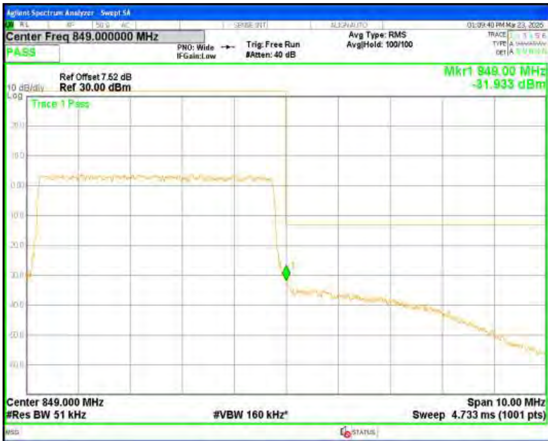
Band5 QPSK BW=1.4MHz Channel=20407 RB Size=6 Position=#0
