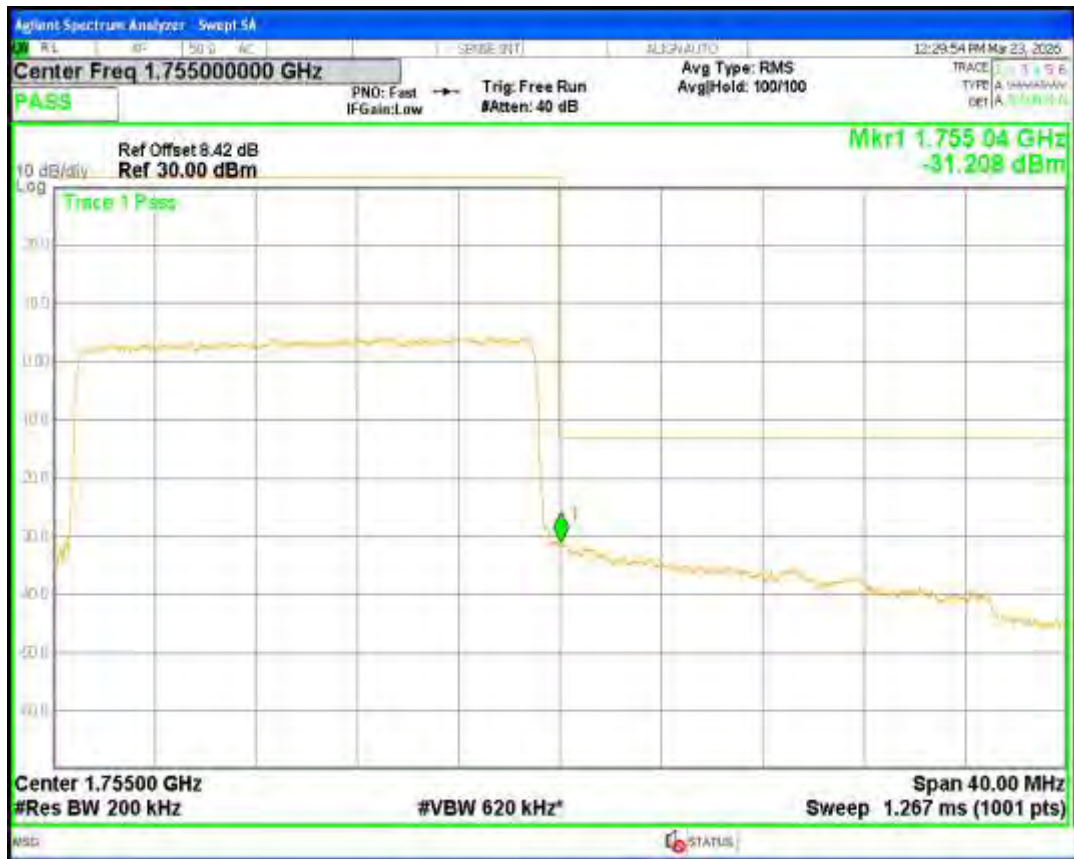
Band4 QPSK BW=5MHz Channel=19975 RB Size=25 Position=#0
