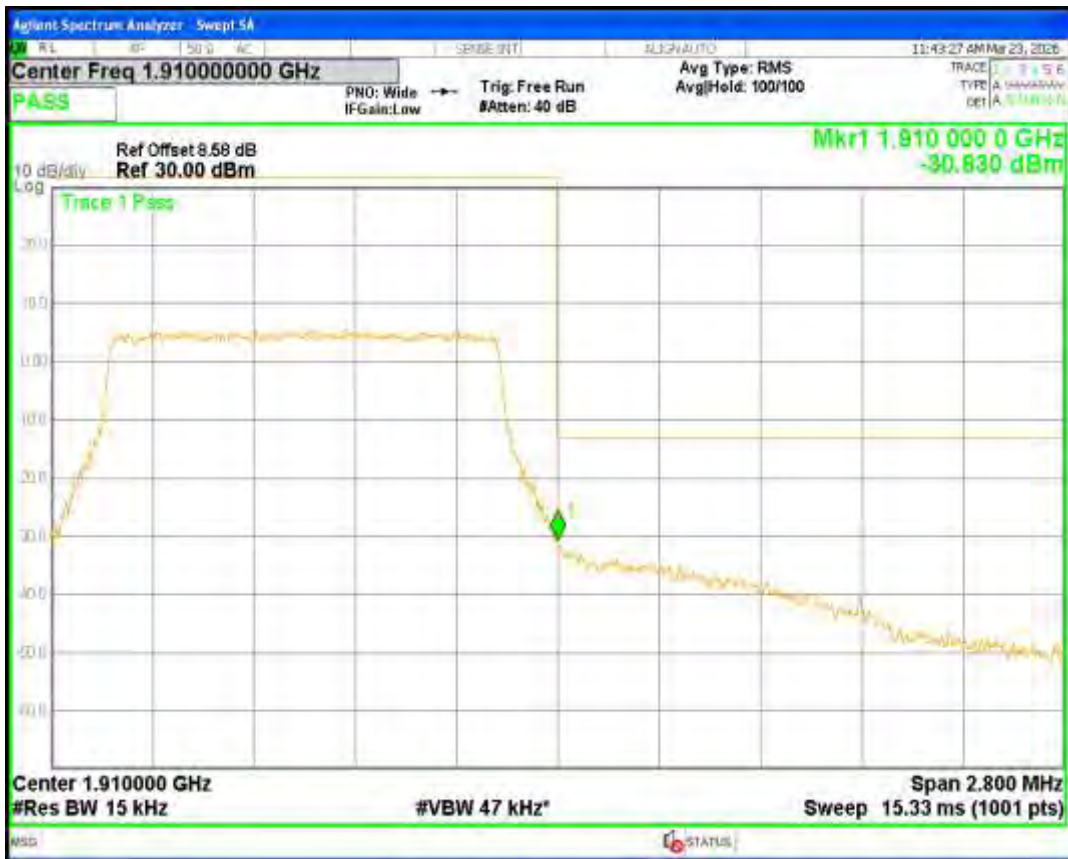
Band2 QPSK BW=10MHz Channel=18650 RB Size=50 Position=#0
