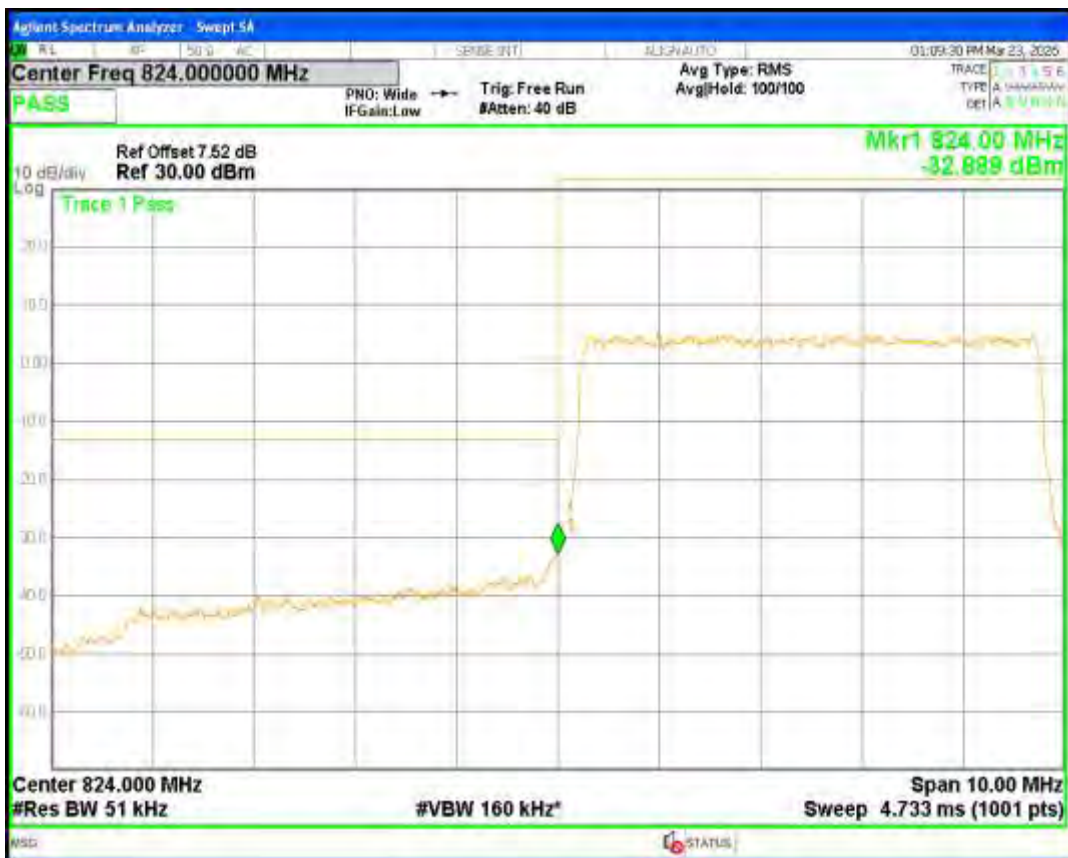
Band5 QPSK BW=5MHz Channel=20625 RB Size=25 Position=#0
