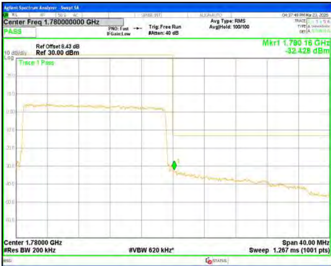
Band66 QPSK BW=3MHz Channel=131987 RB Size=15 Position=#0
