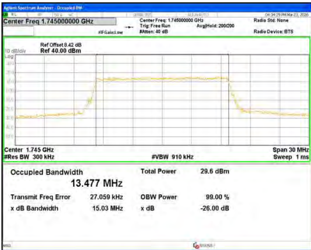
Band66 QPSK BW=15MHz Channel=132597 RB Size=75 Position=#0
