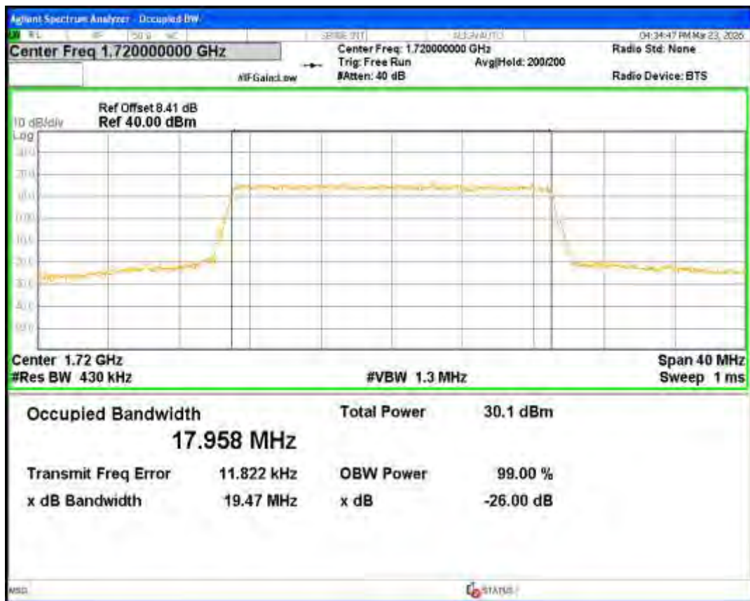
Band66 QPSK BW=20MHz Channel=132322 RB Size=100 Position=#0
