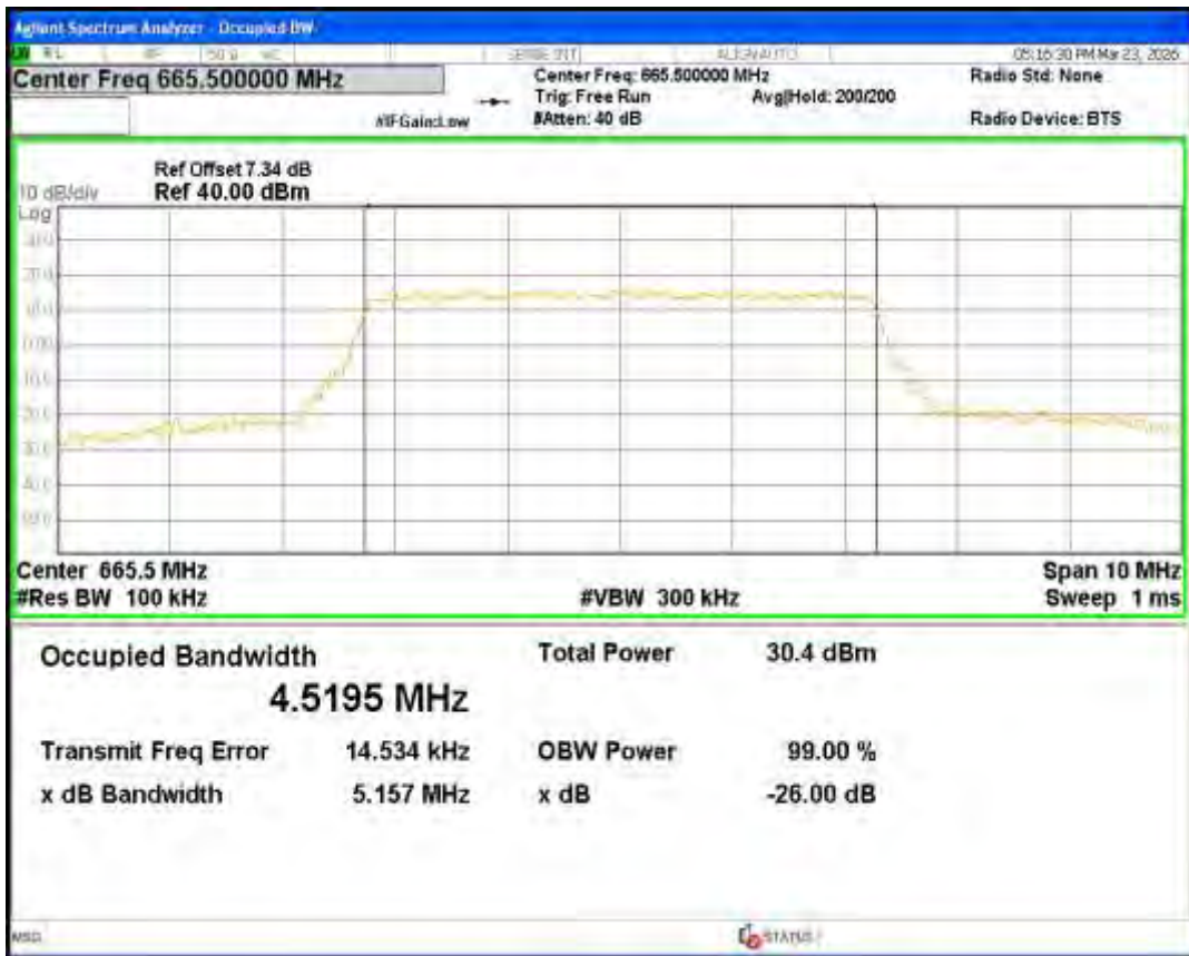
Band71 16QAM BW=5MHz Channel=133447 RB Size=25 Position=#0
