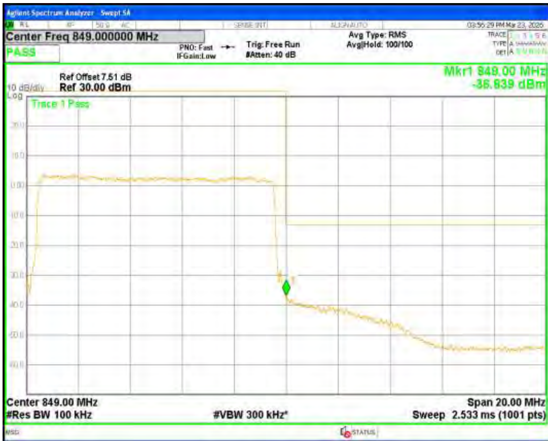
Band26(824-849) 16QAM BW=15MHz Channel=26865 RB Size=75 Position=#0
