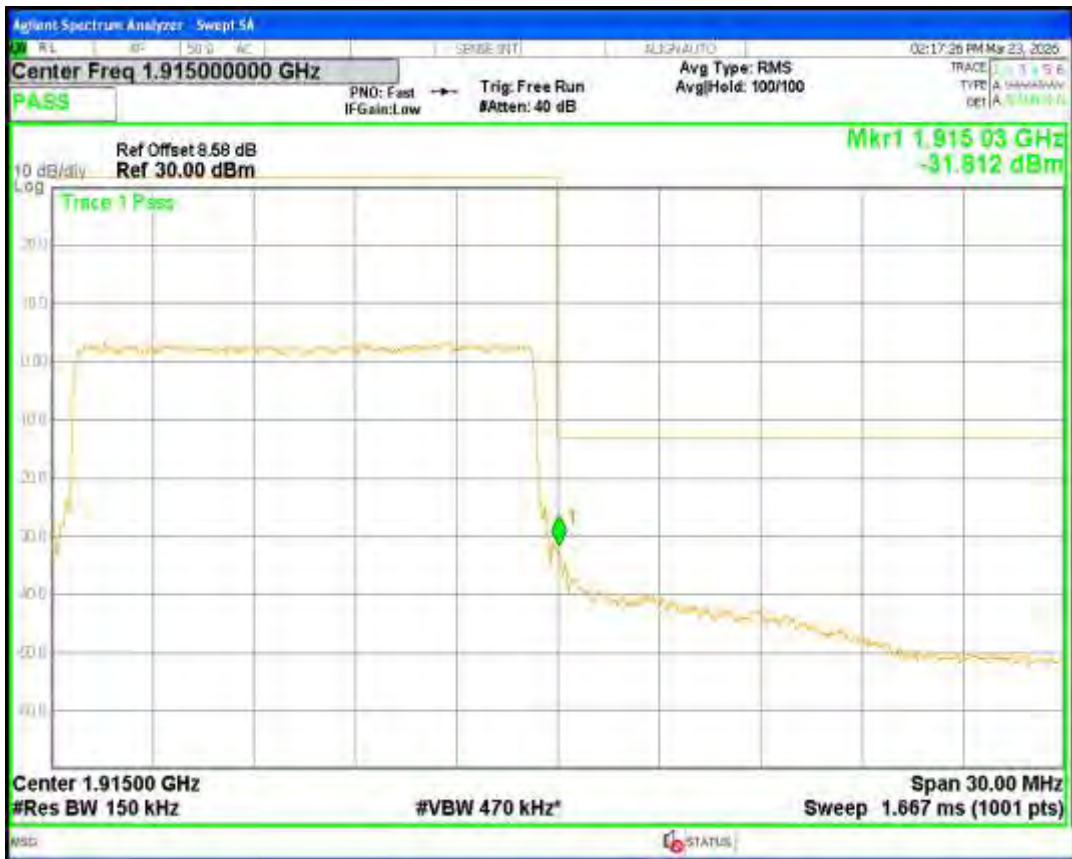
Band25 16QAM BW=20MHz Channel=26140 RB Size=100 Position=#0
