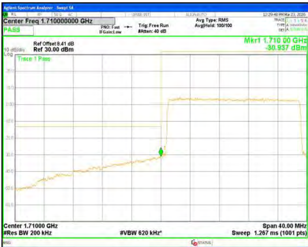
Band4 QPSK BW=20MHz Channel=20300 RB Size=100 Position=#0
