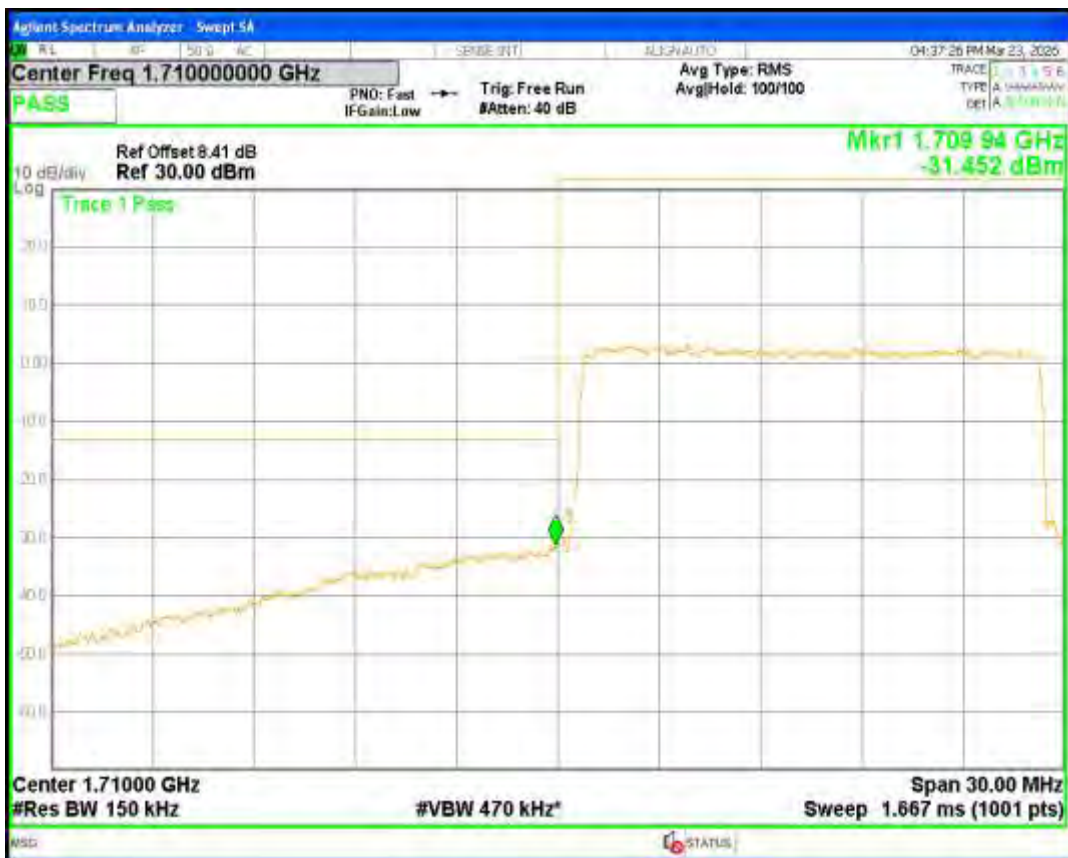
Band66 16QAM BW=15MHz Channel=132597 RB Size=75 Position=#0
