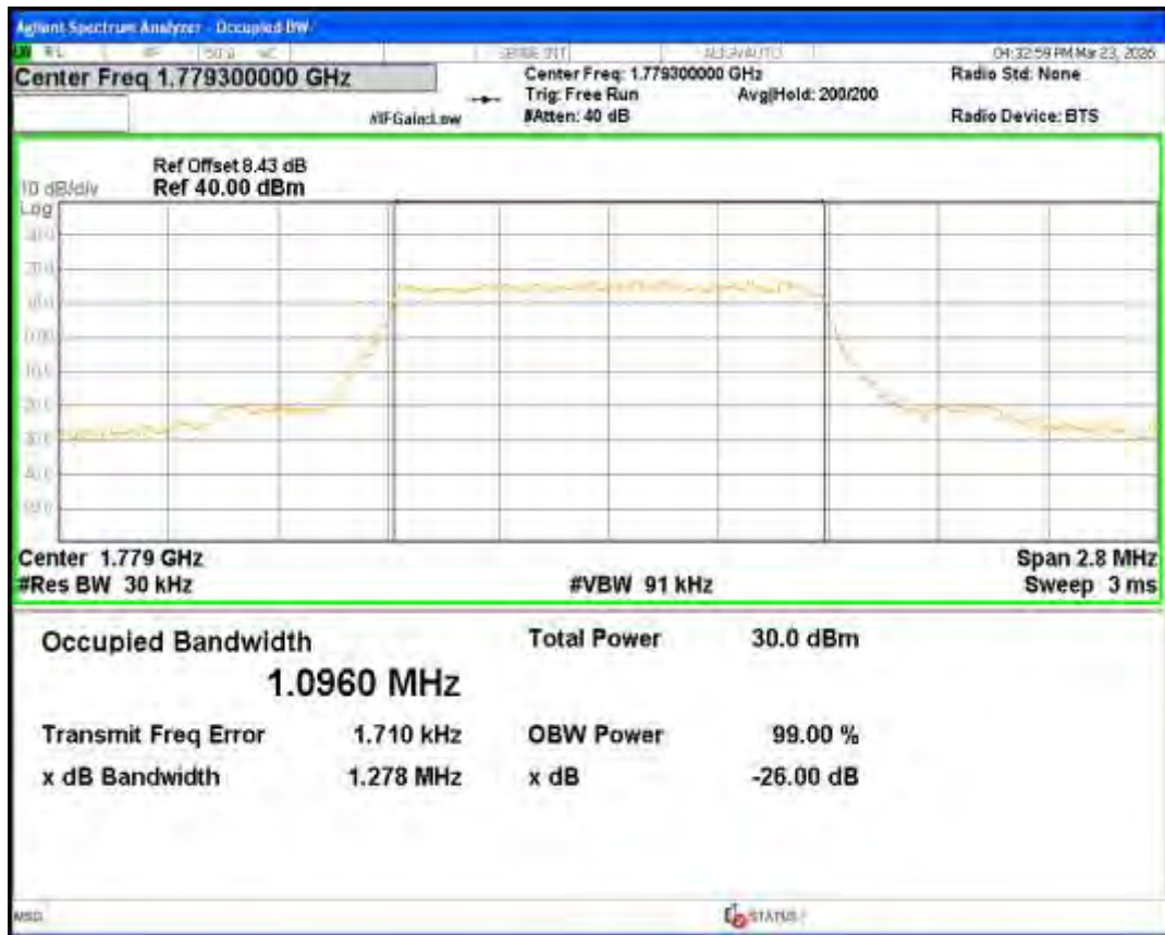
Band66 QPSK BW=10MHz Channel=132022 RB Size=50 Position=#0
