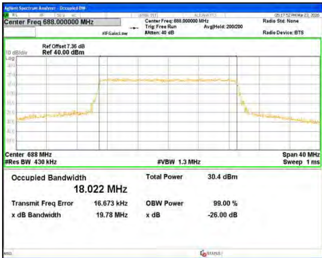
Band71 QPSK BW=10MHz Channel=133172 RB Size=50 Position=#0
