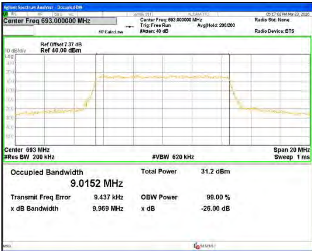
Band71 QPSK BW=15MHz Channel=133197 RB Size=75 Position=#0
