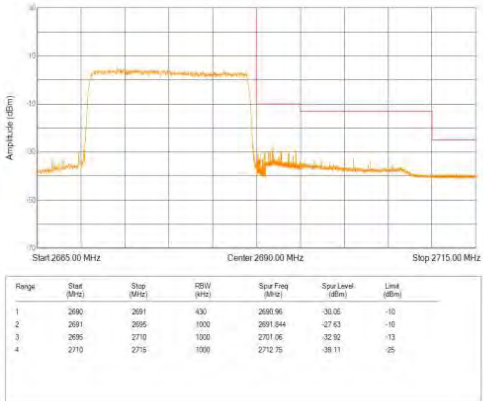
Band41 QPSK BW=5MHz Channel=39675 RB Size=25 Position=#0
