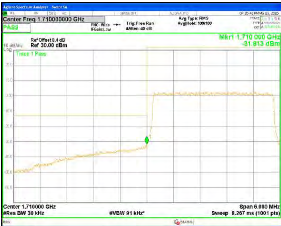
Band66 16QAM BW=3MHz Channel=132657 RB Size=15 Position=#0
