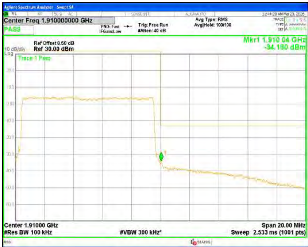
Band2 QPSK BW=15MHz Channel=18675 RB Size=75 Position=#0
