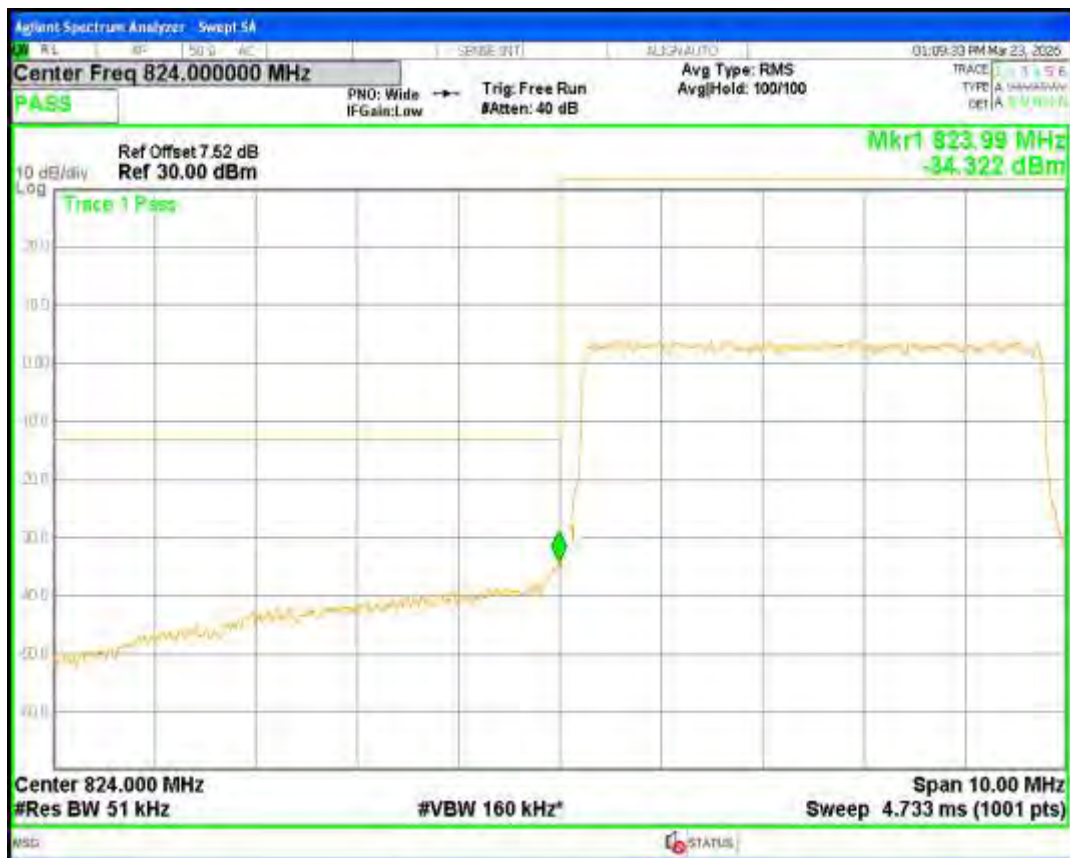
Band5 16QAM BW=5MHz Channel=20625 RB Size=25 Position=#0
