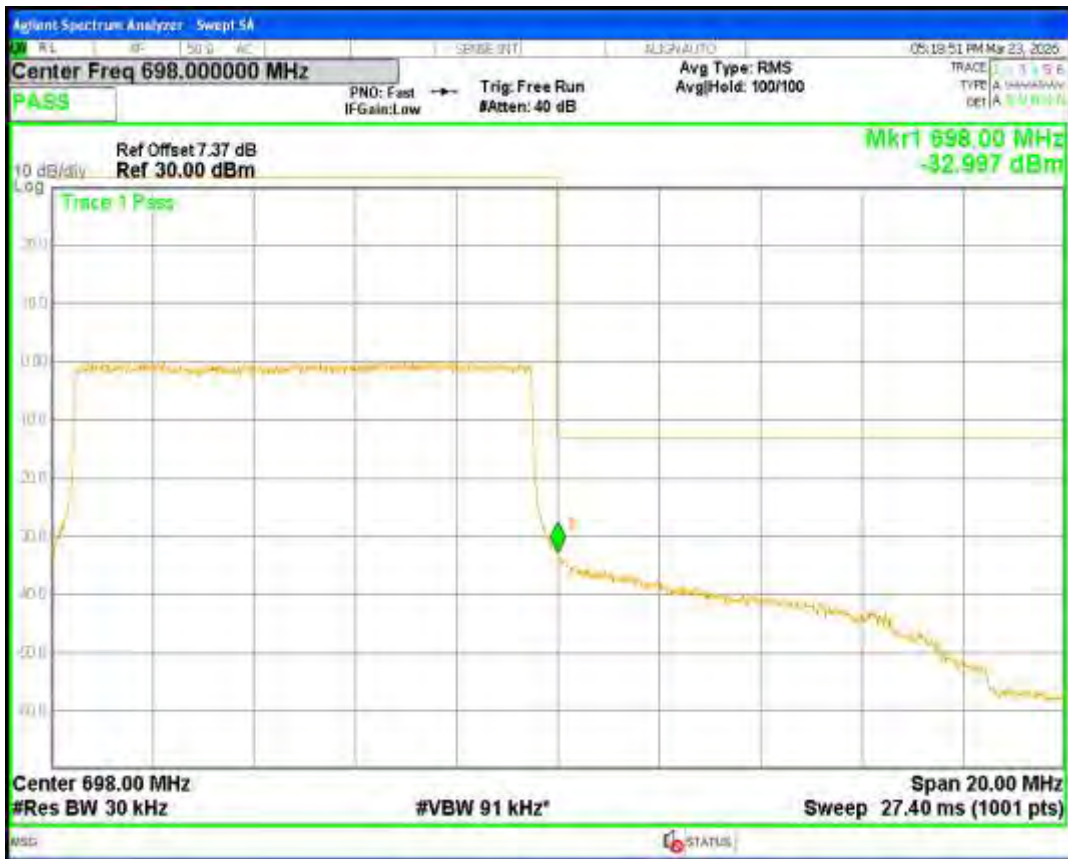
Band71 QPSK BW=15MHz Channel=133197 RB Size=75 Position=#0
