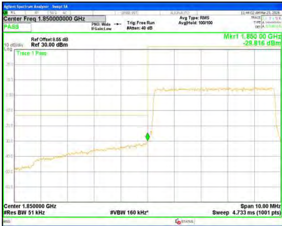
Band2 QPSK BW=3MHz Channel=19185 RB Size=15 Position=#0
