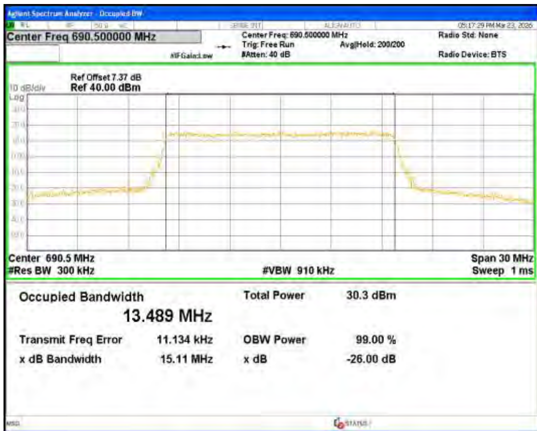
Band71 16QAM BW=20MHz Channel=133222 RB Size=100 Position=#0
