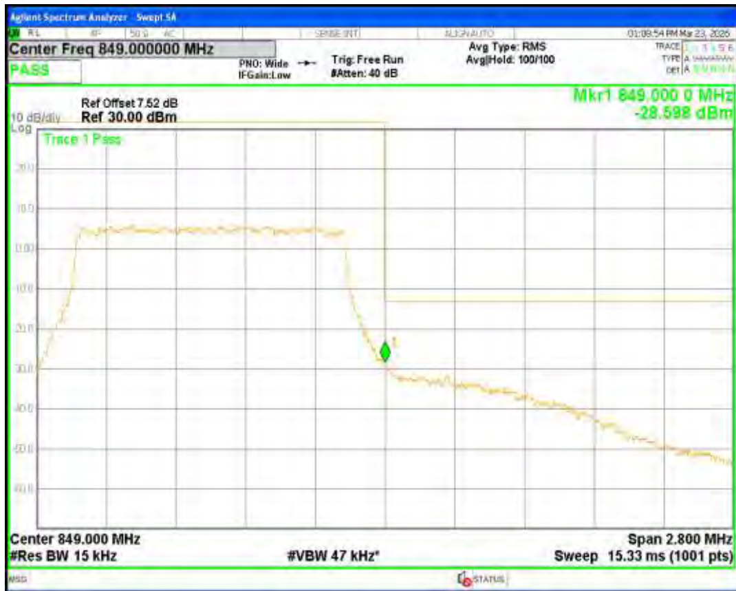
Band5 QPSK BW=10MHz Channel=20450 RB Size=50 Position=#0
