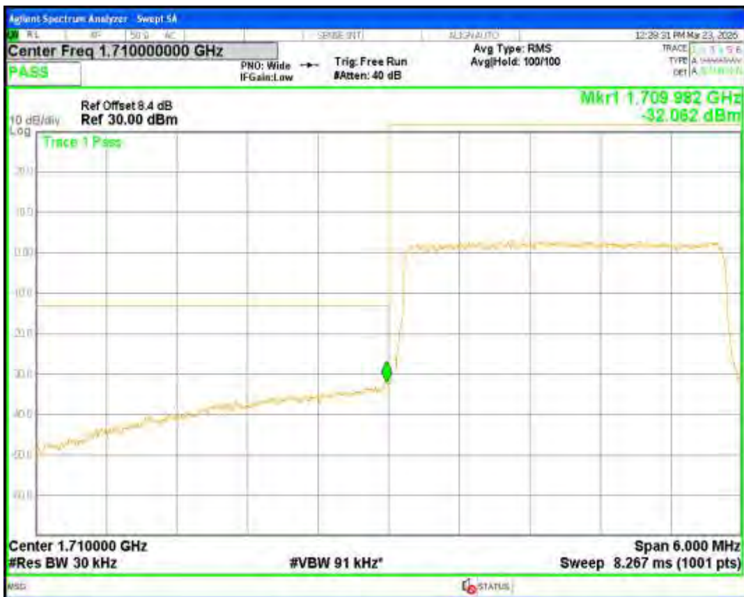
Band4 16QAM BW=3MHz Channel=20385 RB Size=15 Position=#0
