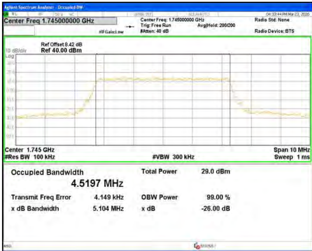
Band66 QPSK BW=1.4MHz Channel=131979 RB Size=6 Position=#0
