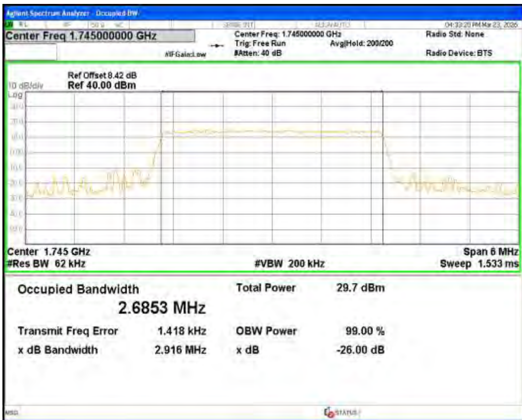
Band66 16QAM BW=3MHz Channel=132657 RB Size=15 Position=#0
