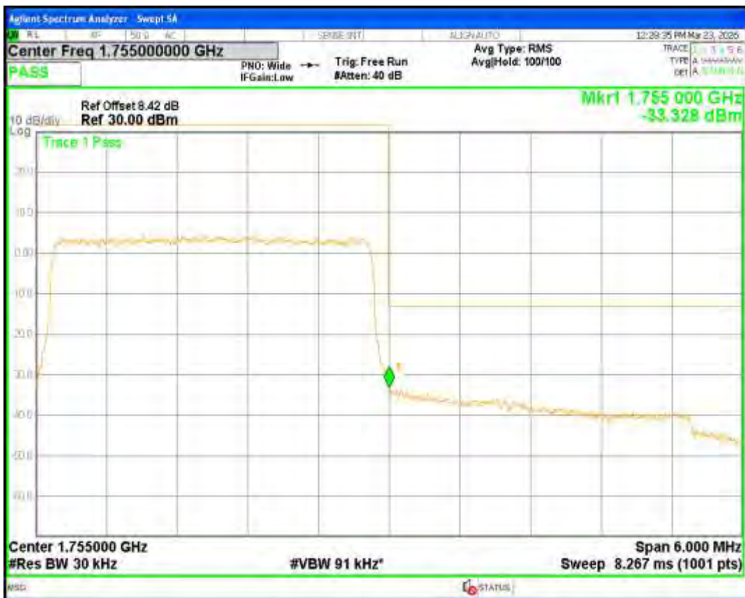
Band4 QPSK BW=5MHz Channel=20375 RB Size=25 Position=#0
