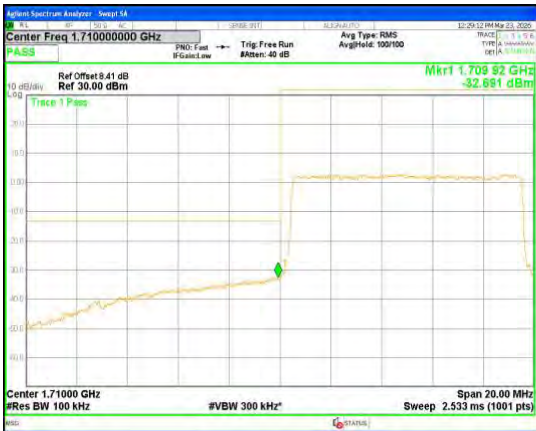
Band4 16QAM BW=10MHz Channel=20350 RB Size=50 Position=#0
