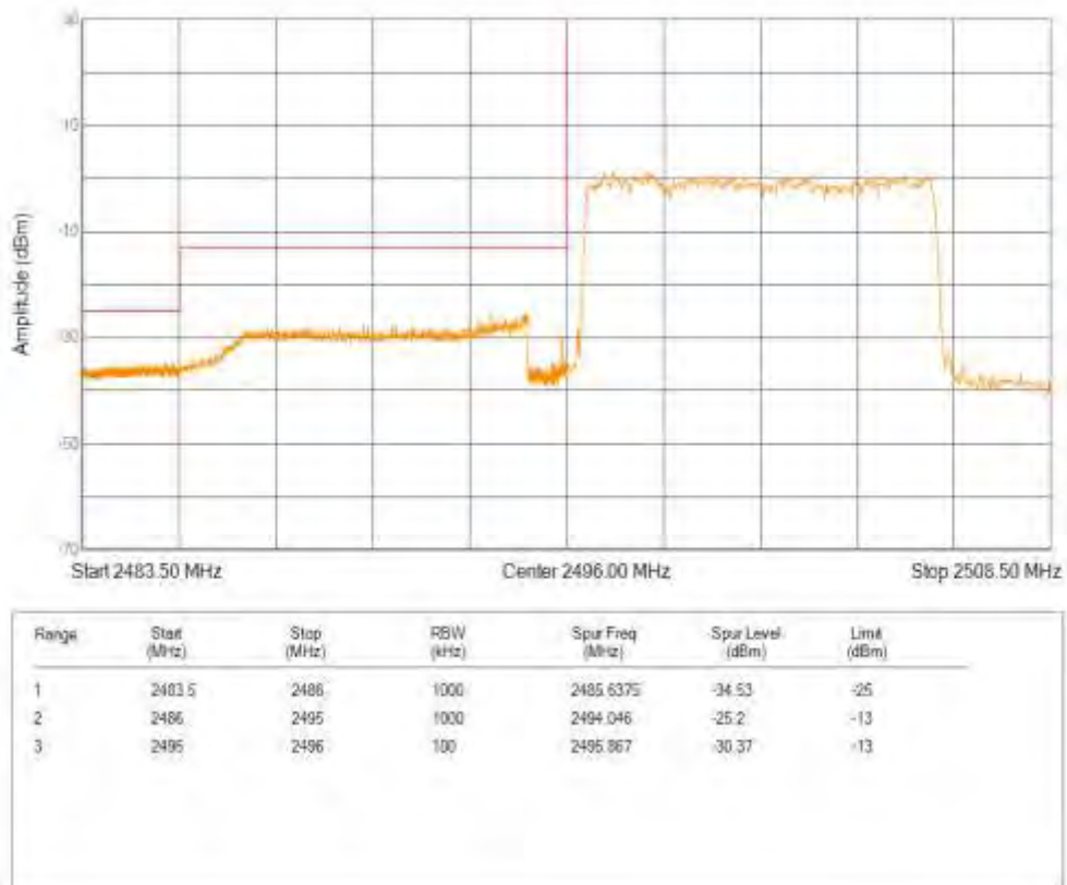
Band41 QPSK BW=10MHz Channel=41540 RB Size=50 Position=#0
