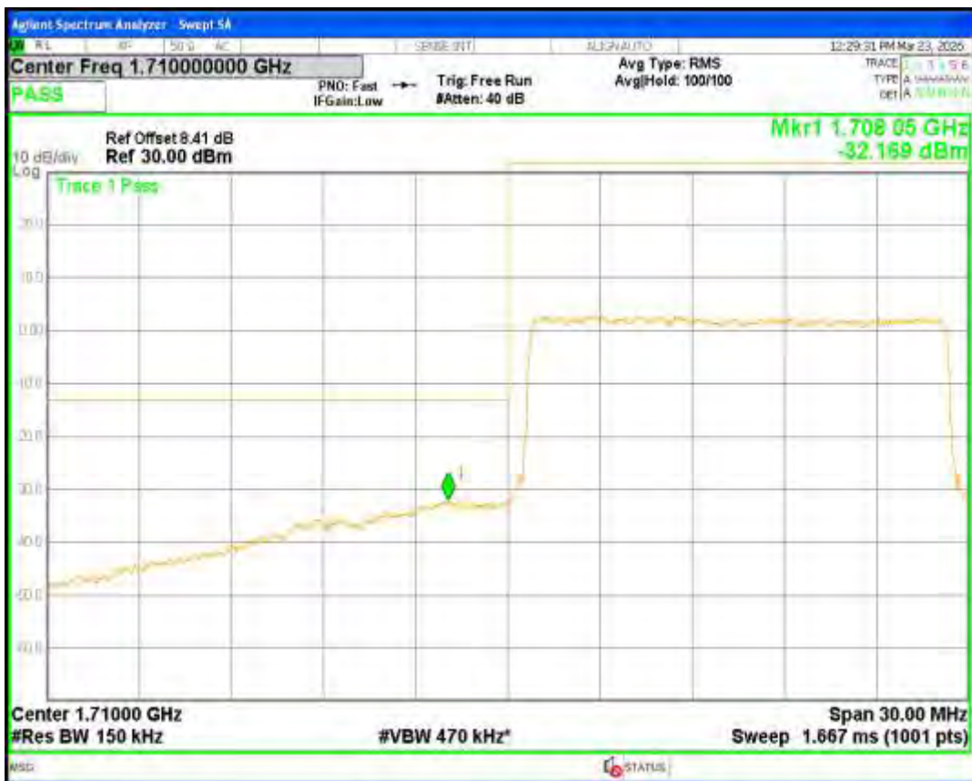
Band4 16QAM BW=15MHz Channel=20325 RB Size=75 Position=#0
