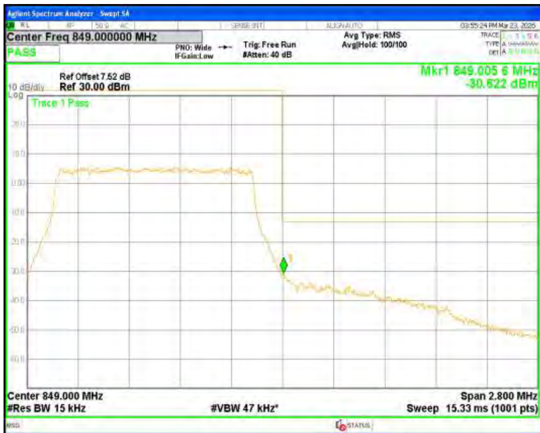
Band26(824-849) QPSK BW=1.4MHz Channel=26797 RB Size=6 Position=#0
