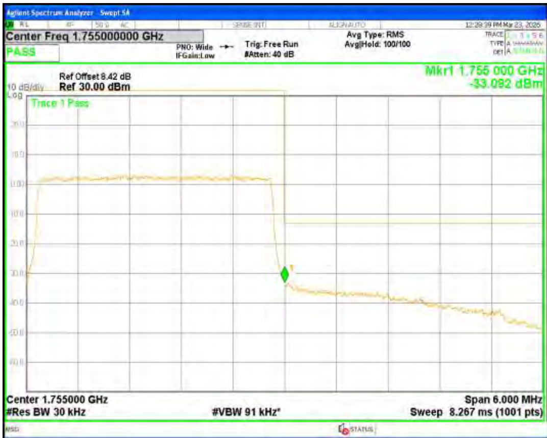
Band4 QPSK BW=10MHz Channel=20000 RB Size=50 Position=#0
