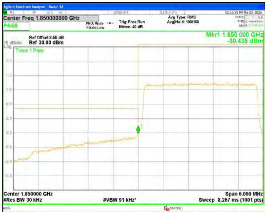
Band25 QPSK BW=3MHz Channel=26675 RB Size=15 Position=#0
