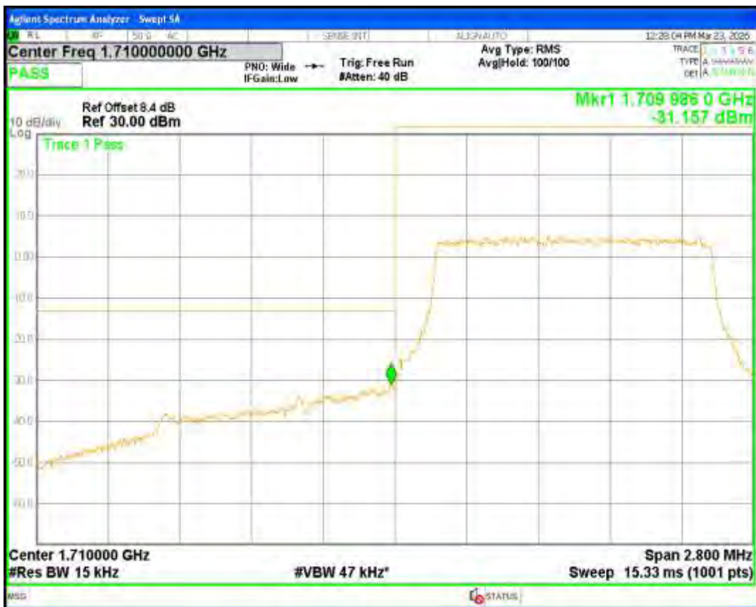
Band4 QPSK BW=10MHz Channel=20350 RB Size=50 Position=#0
