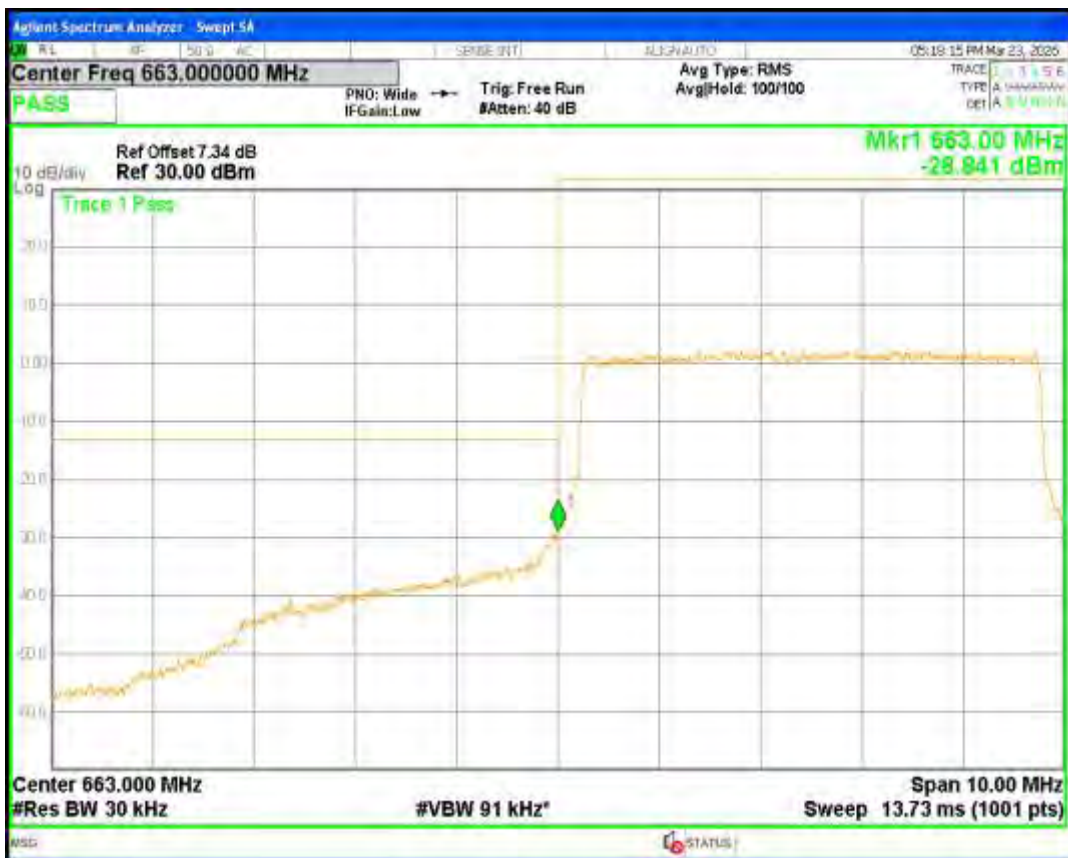
Band71 16QAM BW=5MHz Channel=133447 RB Size=25 Position=#0
