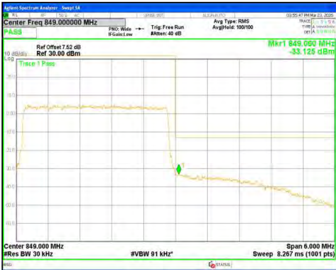
Band26(824-849) QPSK BW=5MHz Channel=26815 RB Size=25 Position=#0
