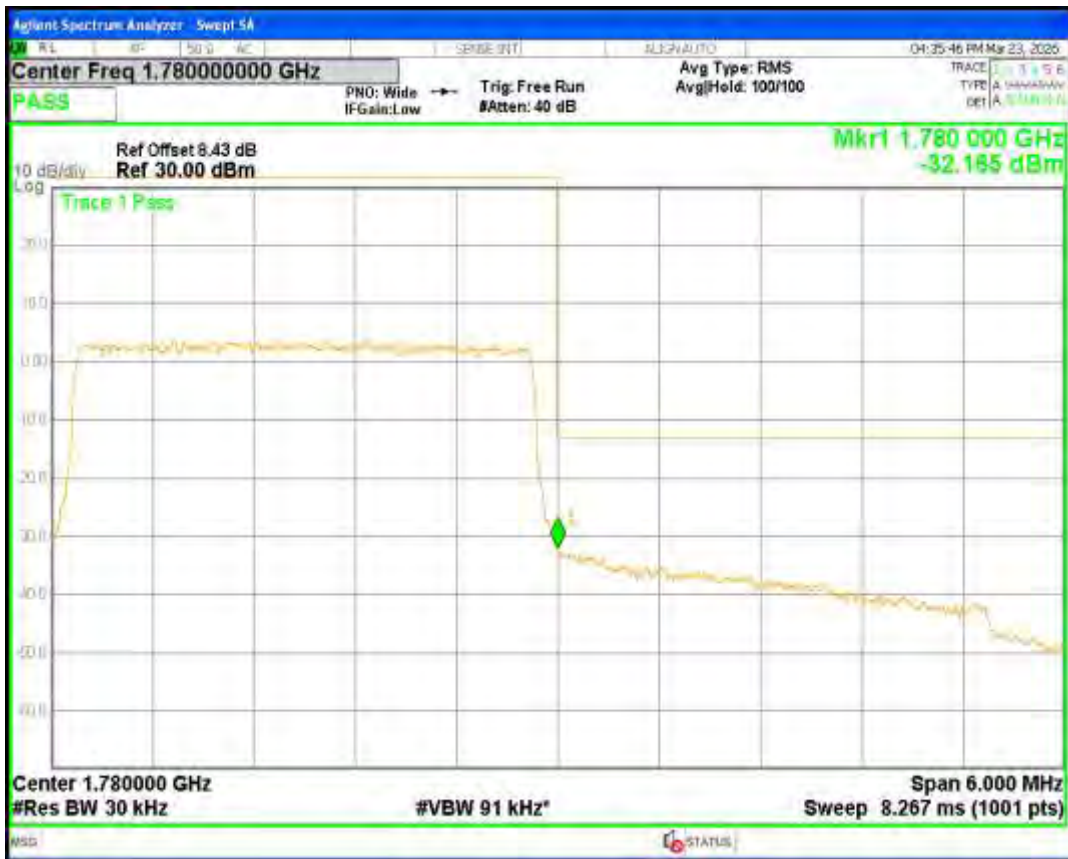
Band66 QPSK BW=5MHz Channel=131997 RB Size=25 Position=#0
