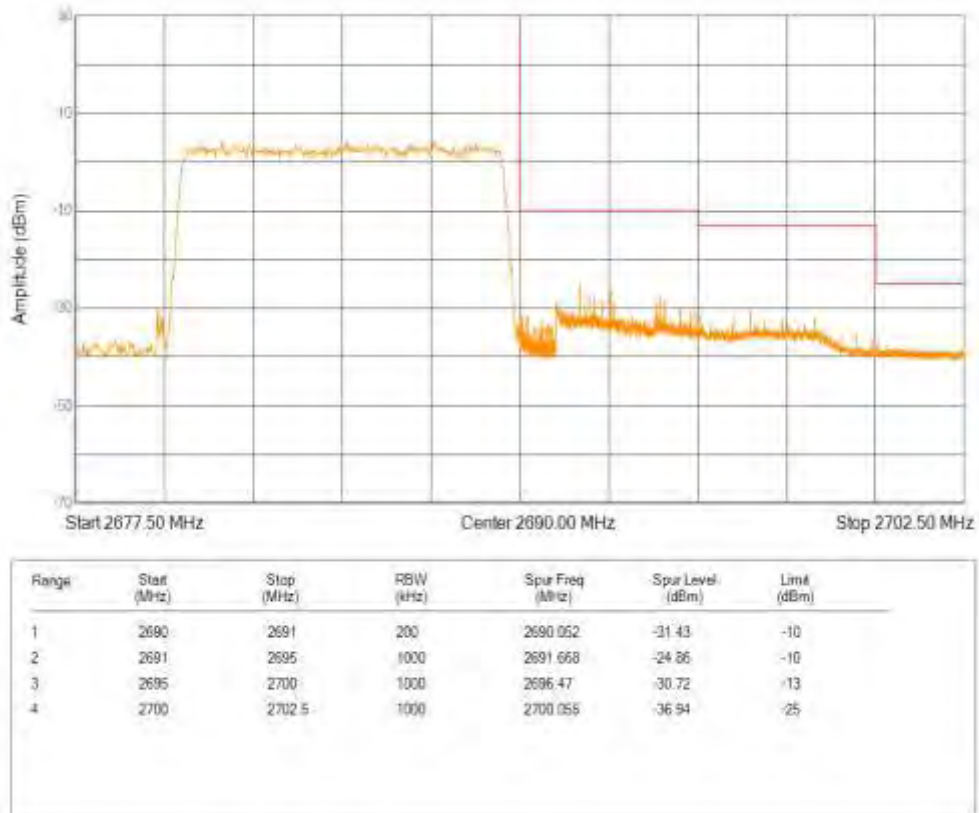
Band41 QPSK BW=15MHz Channel=39725 RB Size=75 Position=#0
