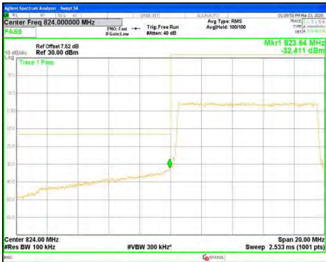
Band5 QPSK BW=10MHz Channel=20600 RB Size=50 Position=#0
