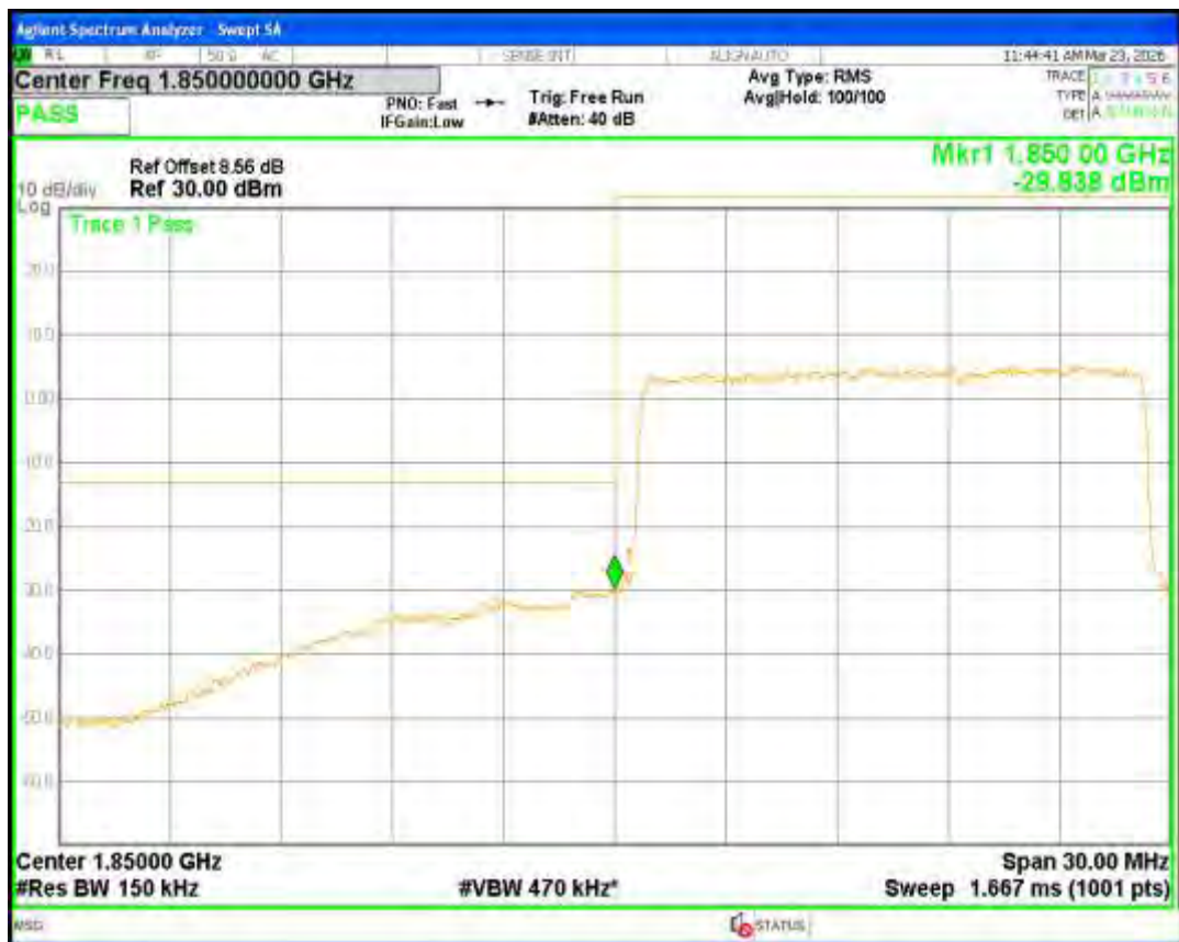
Band2 QPSK BW=15MHz Channel=19125 RB Size=75 Position=#0
