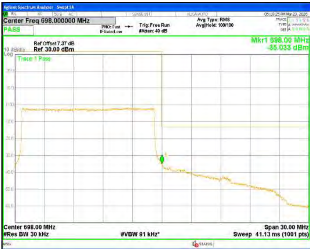
Band71 QPSK BW=20MHz Channel=133222 RB Size=100 Position=#0
