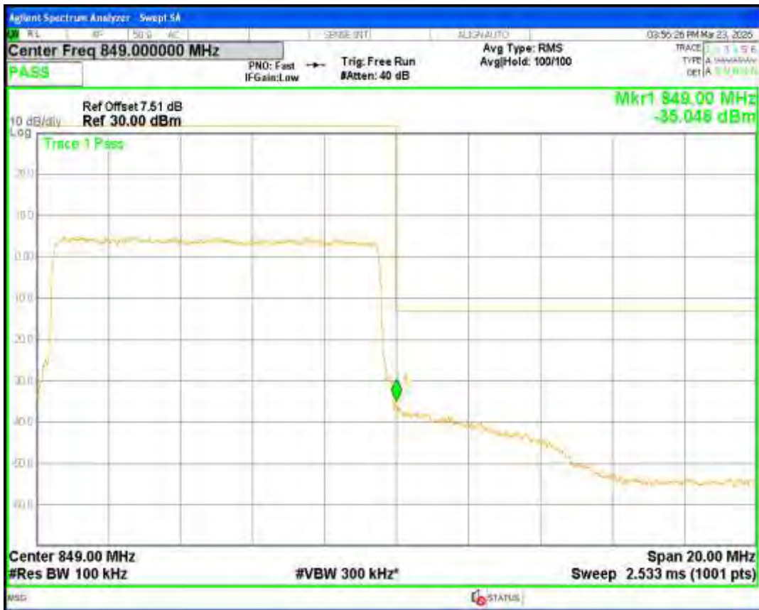
Band26(824-849) QPSK BW=15MHz Channel=26865 RB Size=75 Position=#0
