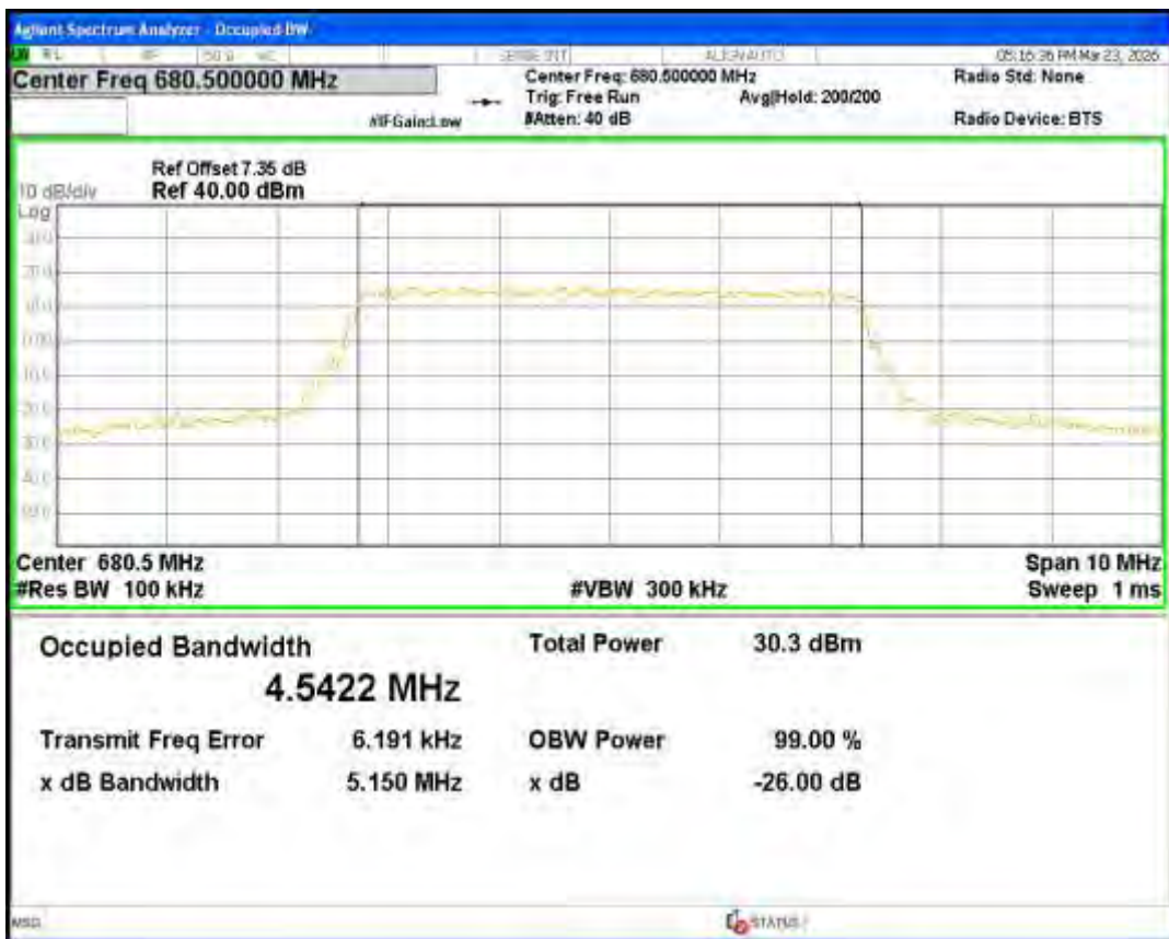
Band71 16QAM BW=5MHz Channel=133147 RB Size=25 Position=#0
