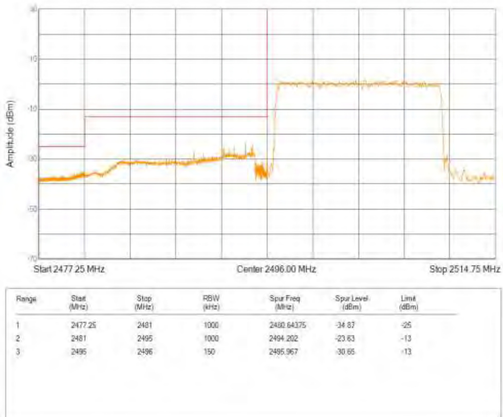
Band41 QPSK BW=15MHz Channel=41515 RB Size=75 Position=#0
