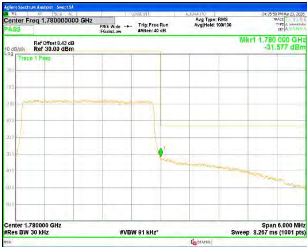
Band66 QPSK BW=1.4MHz Channel=131979 RB Size=6 Position=#0
