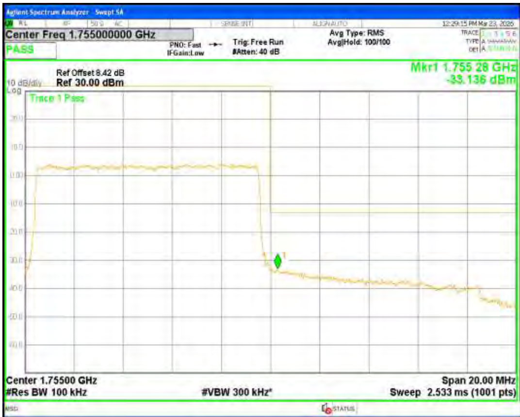
Band4 QPSK BW=15MHz Channel=20025 RB Size=75 Position=#0
