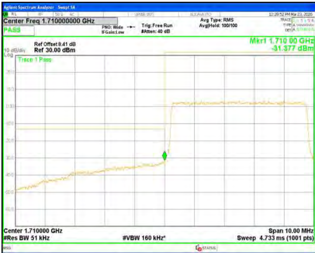
Band4 QPSK BW=1.4MHz Channel=19957 RB Size=6 Position=#0
