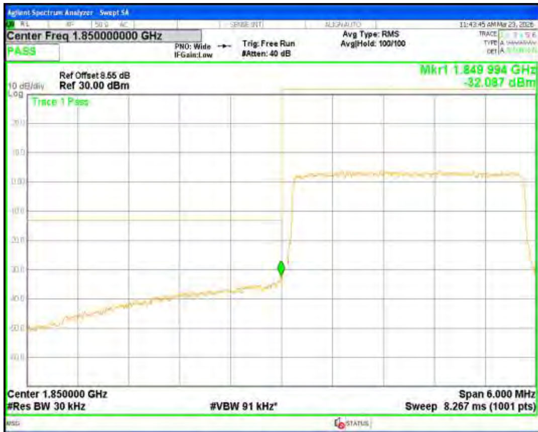
Band2 QPSK BW=1.4MHz Channel=18607 RB Size=6 Position=#0
