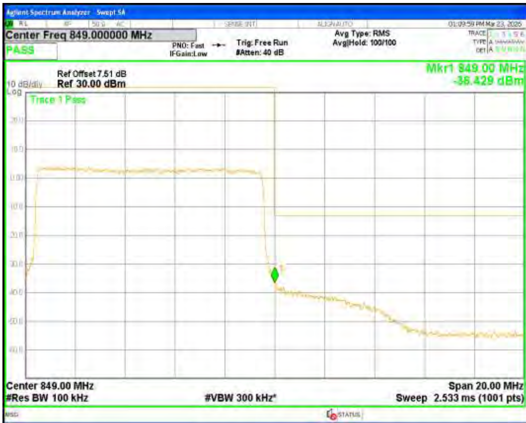
Band5 16QAM BW=3MHz Channel=20415 RB Size=15 Position=#0
