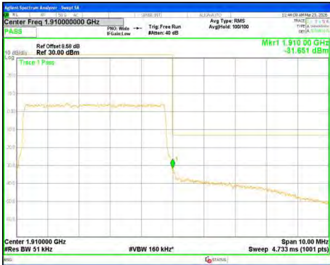
Band25 16QAM BW=1.4MHz Channel=26047 RB Size=6 Position=#0
