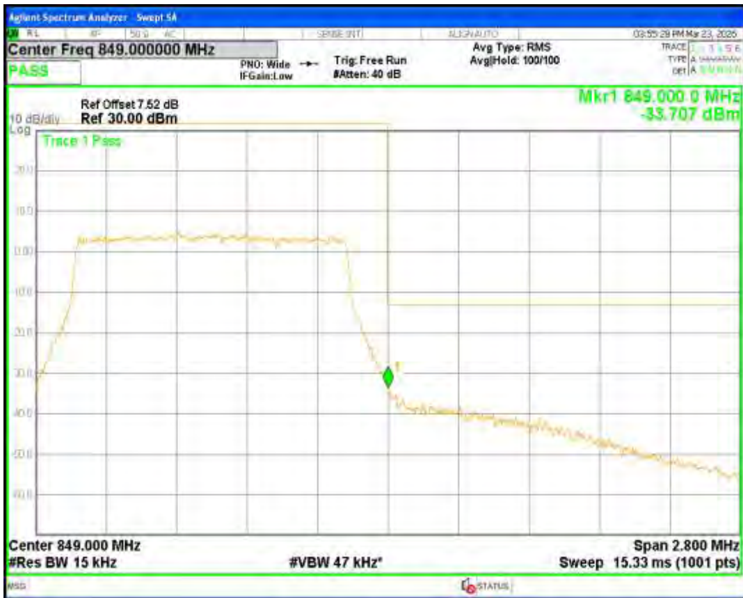
Band26(824-849) 16QAM BW=10MHz Channel=26840 RB Size=50 Position=#0
