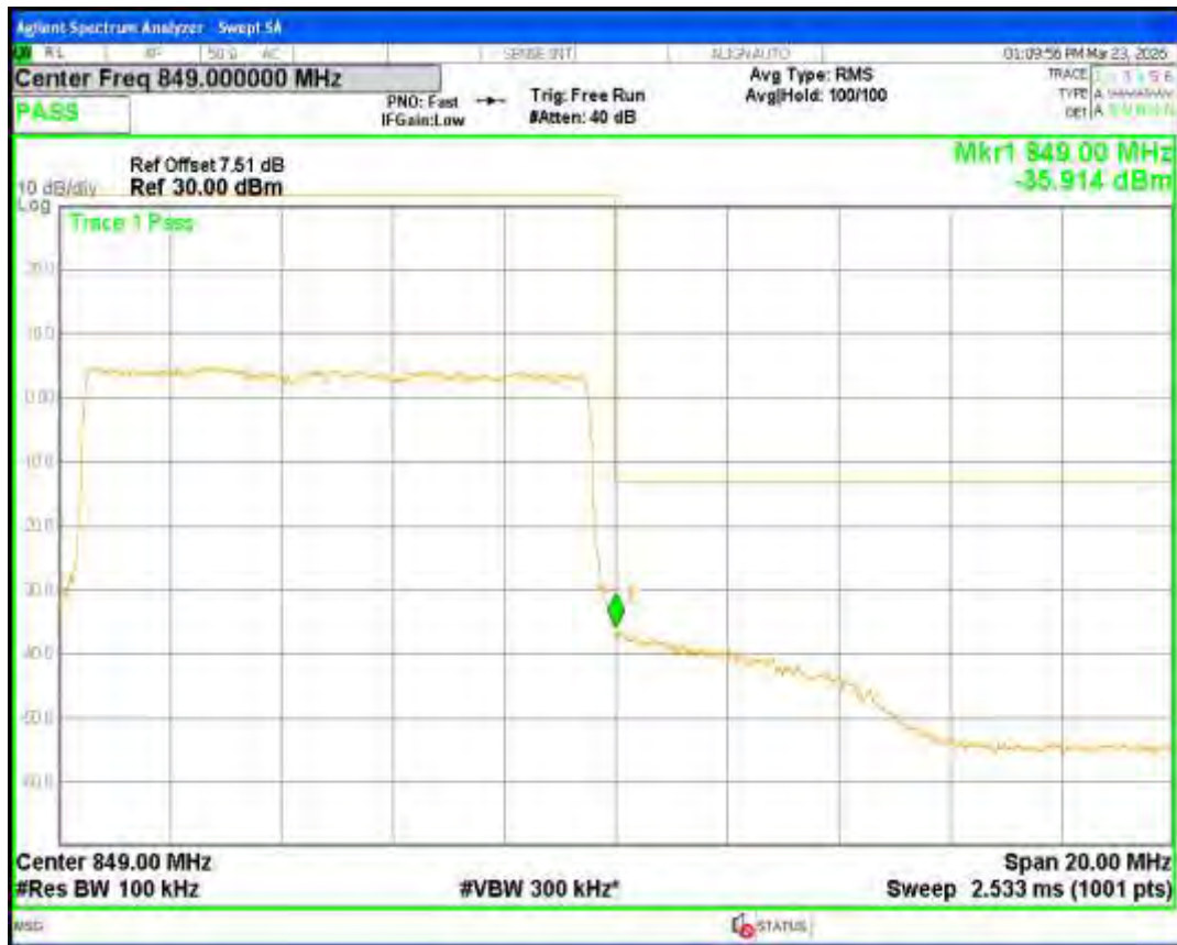
Band5 QPSK BW=3MHz Channel=20415 RB Size=15 Position=#0
