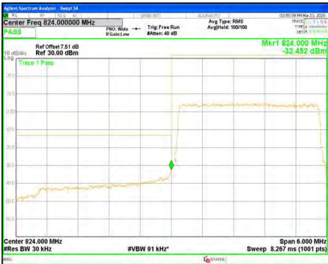
Band26(824-849) QPSK BW=3MHz Channel=27025 RB Size=15 Position=#0
