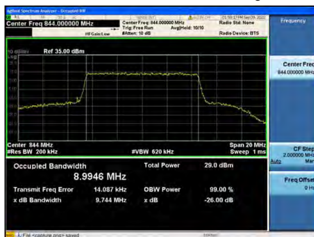
Band26Part22 / 10MHz / QPSK/ High CH
