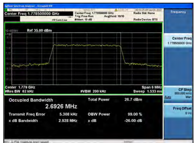
Band66 / 3MHz / 16QAM/ High CH
