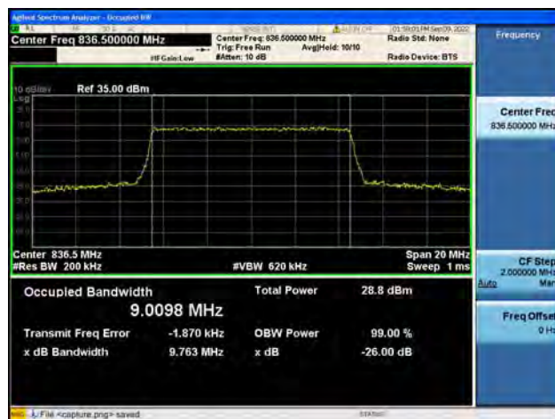
Band26Part22 / 10MHz / QPSK/ High CH
