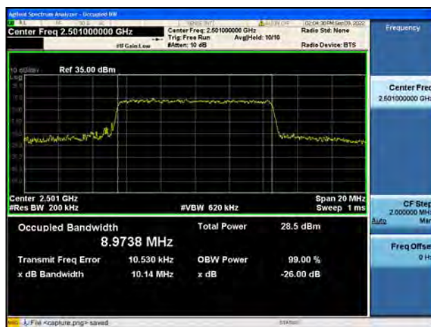
Band41 / 10MHz / 16QAM/ Mid CH
