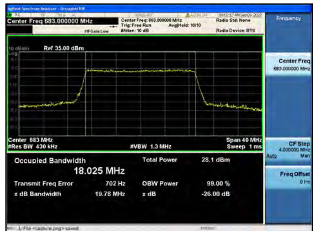
Band71 / 20MHz / 16QAM/ High CH
