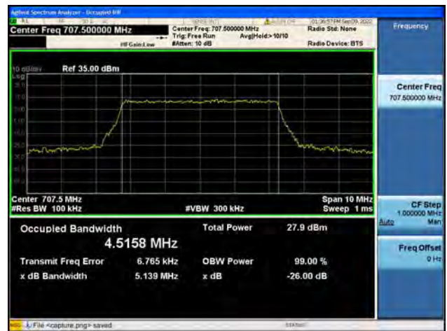
Band12 / 5MHz / 16QAM/ High CH
