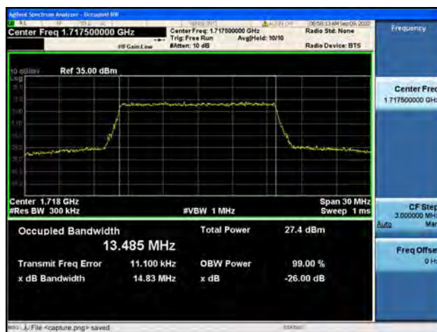
Band66 / 15MHz / 16QAM/ Mid CH
