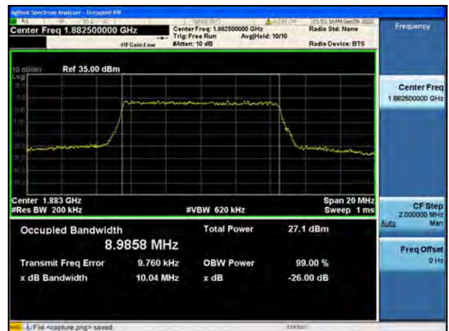
Band25 / 10MHz / 16QAM/ High CH
