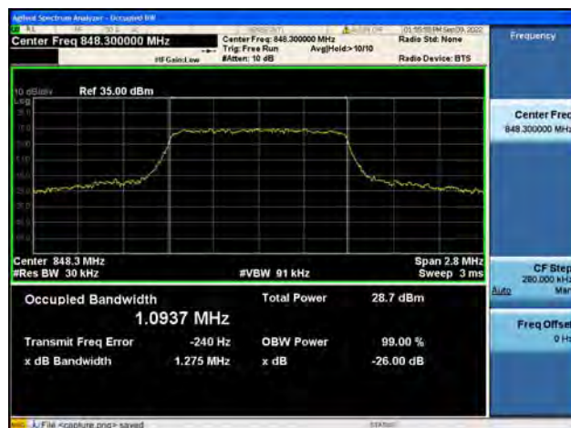
Band26Part22 / 1.4MHz / QPSK/ High CH
