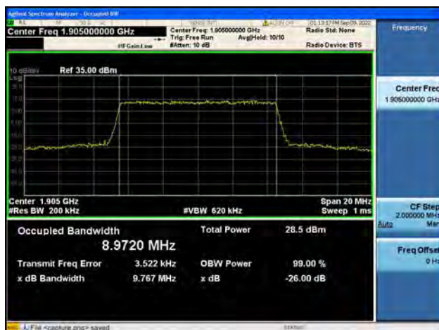
Band2 / 10MHz / QPSK/ High CH
