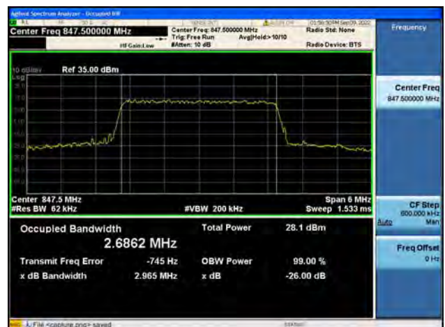
Band26Part22 / 3MHz / 16QAM/ High CH
