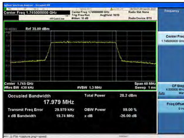
Band66 / 20MHz / QPSK/ High CH
