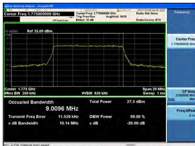
Band66 / 10MHz / QPSK/ High CH
