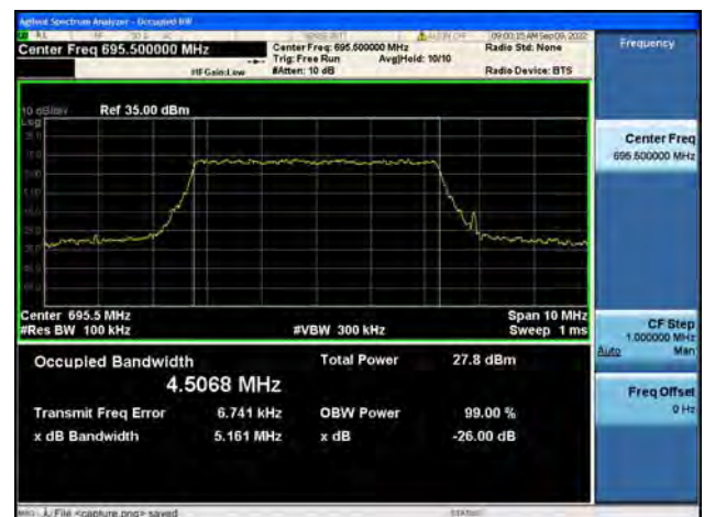
Band71 / 5MHz / 16QAM/ High CH
