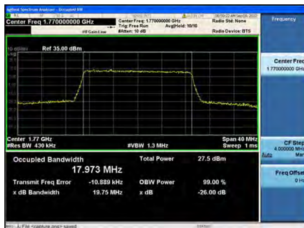
Band66 / 20MHz / QPSK/ High CH
