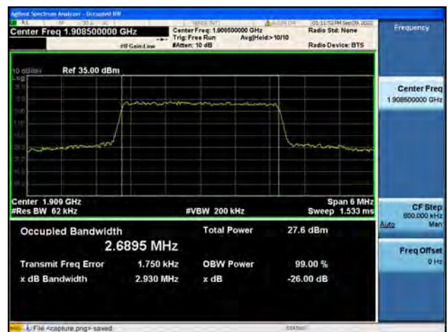
Band2 / 3MHz / 16QAM/ High CH
