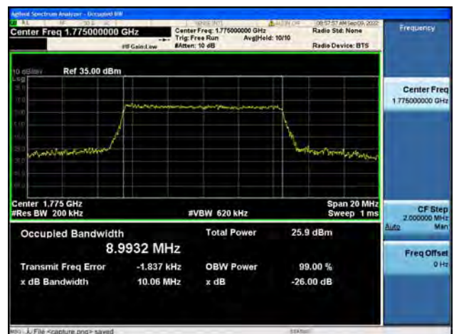
Band66 / 10MHz / 16QAM/ High CH
