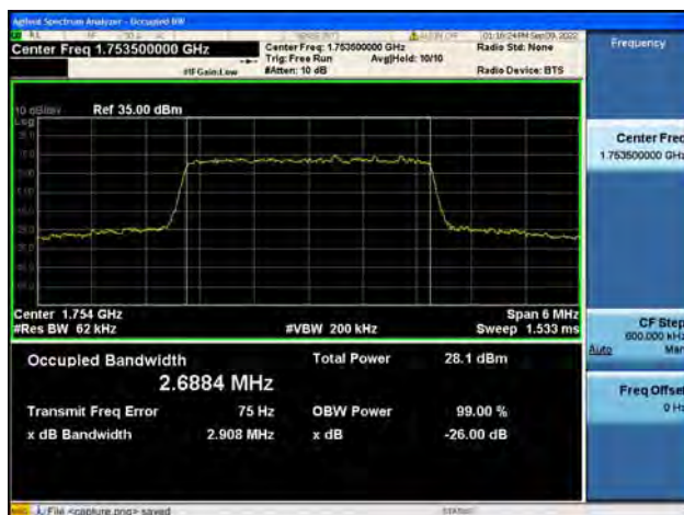
Band4 / 3MHz / QPSK/ High CH
