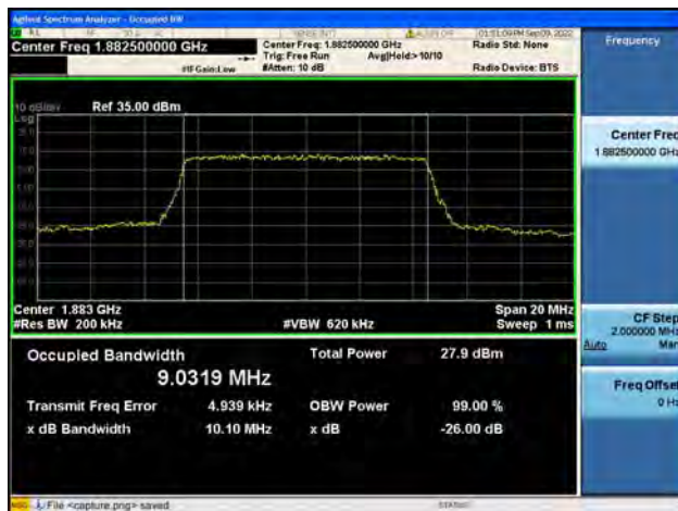
Band25 / 10MHz / QPSK/ High CH
