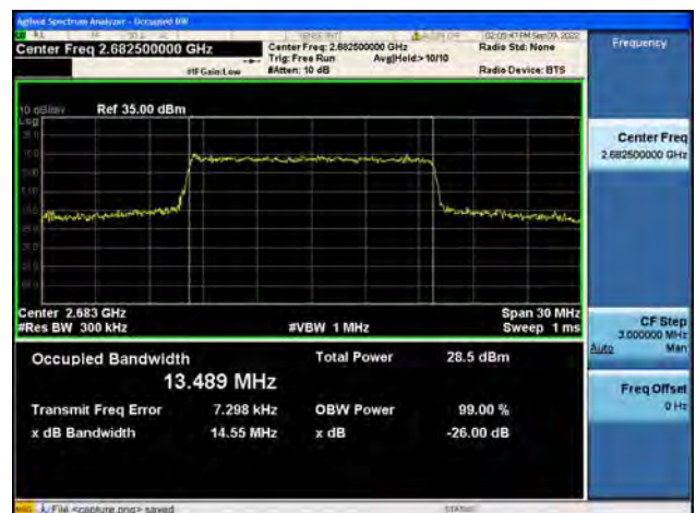
Band41 / 15MHz / 16QAM/ High CH
