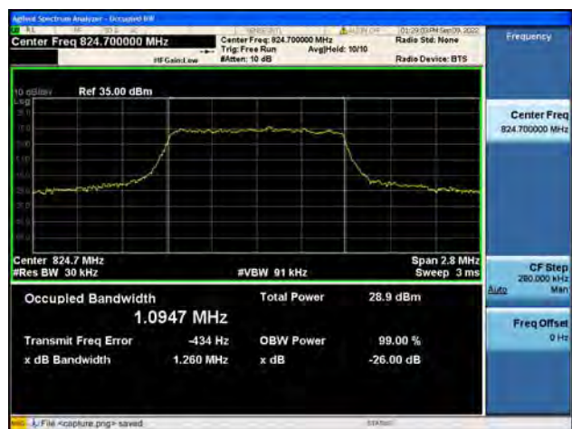
Band5 / 1.4MHz / QPSK/ Mid CH
