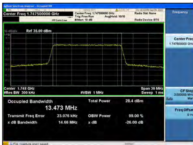
Band4 / 15MHz / QPSK/ High CH
