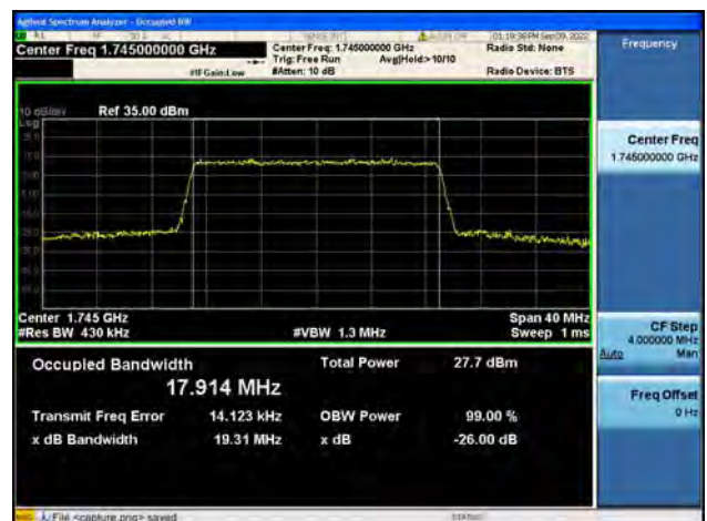
Band4 / 20MHz / 16QAM/ High CH
