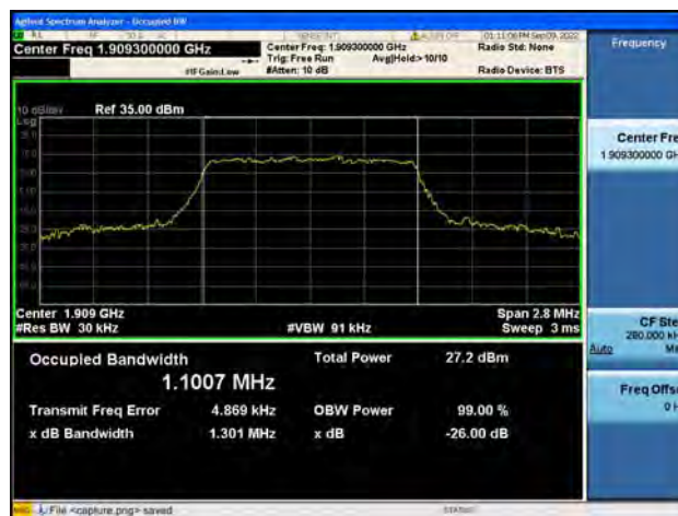
Band2 / 1.4MHz / 16QAM/ High CH
