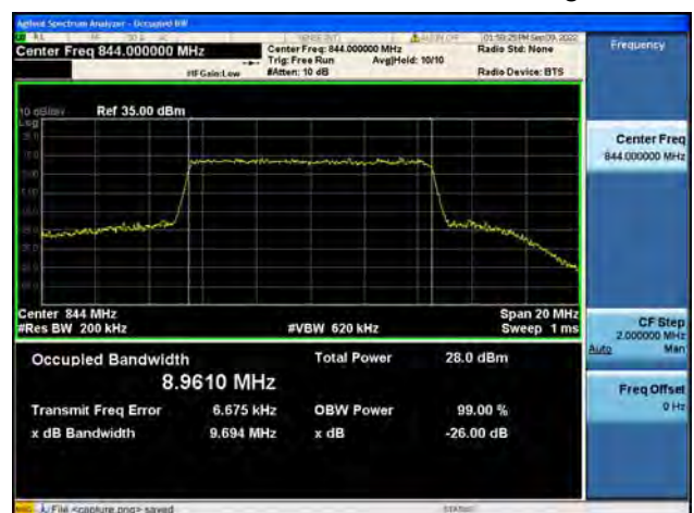
Band26Part22 / 10MHz / 16QAM/ High CH
