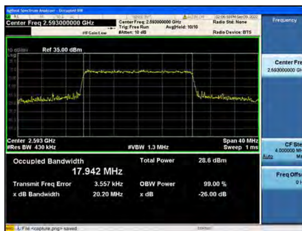
Band41 / 20MHz / 16QAM/ High CH
