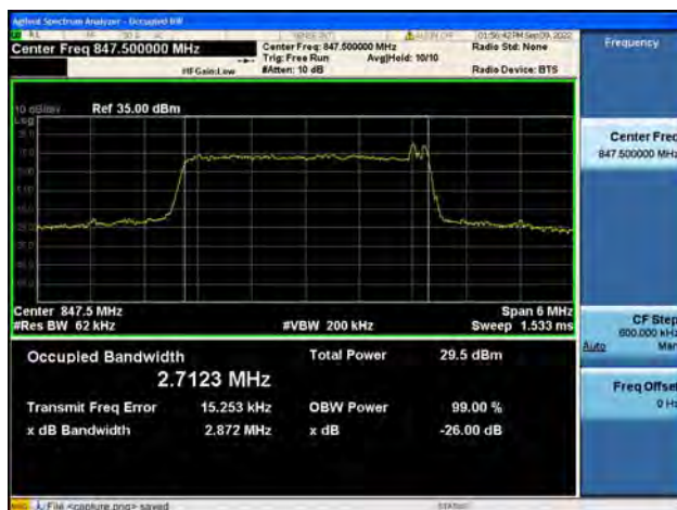
Band26Part22 / 3MHz / QPSK/ High CH
