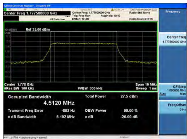
Band66 / 5MHz / QPSK/ High CH
