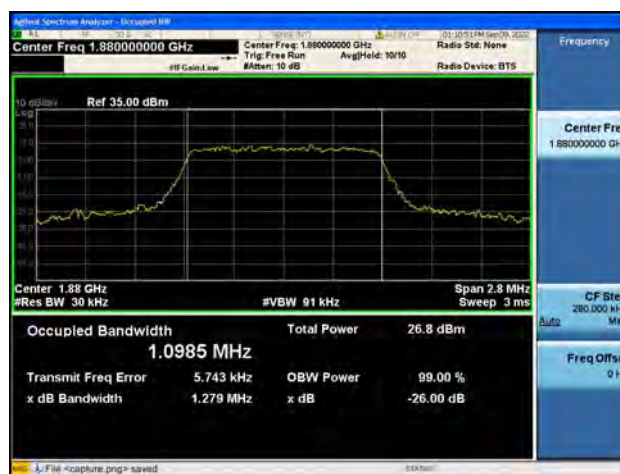
Band2 / 1.4MHz / 16QAM/ High CH
