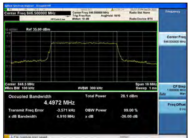
Band26Part22 / 5MHz / 16QAM/ High CH
