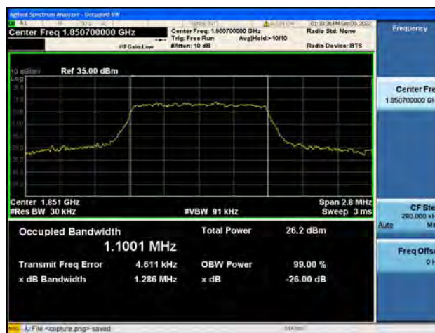
Band2 / 1.4MHz / 16QAM/ Mid CH
