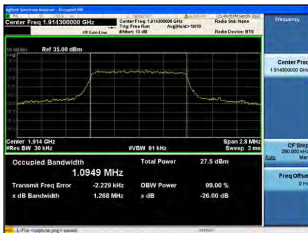
Band25 / 1.4MHz / QPSK/ High CH
