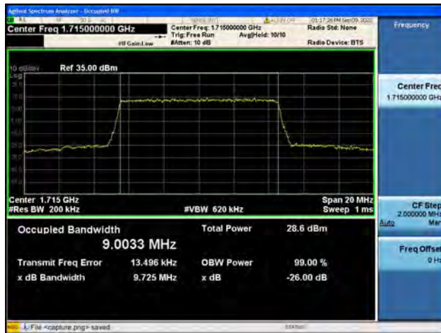
Band4 / 10MHz / QPSK/ Mid CH
