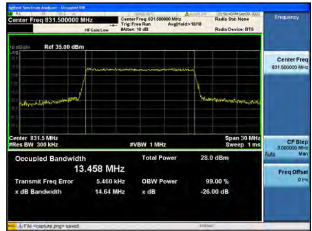
Band26Part22 / 15MHz / 16QAM/ Mid CH
