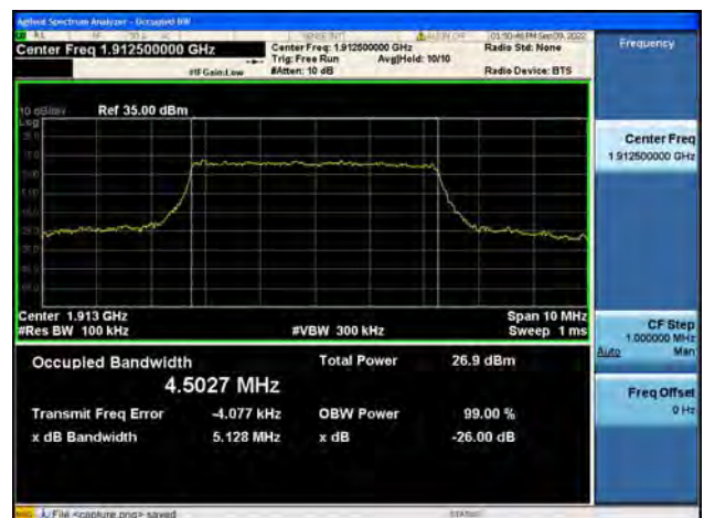
Band25 / 5MHz / 16QAM/ High CH
