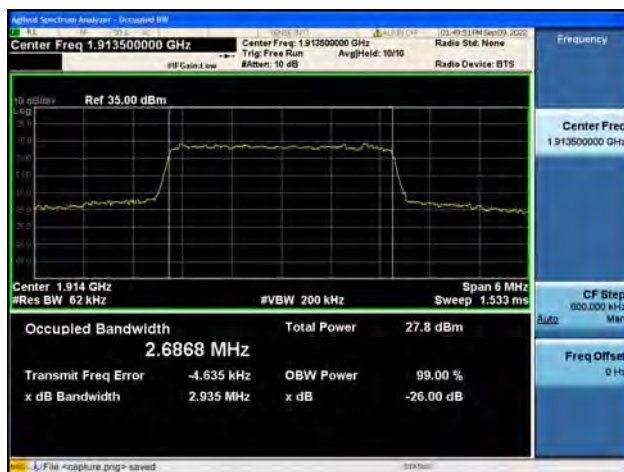
Band25 / 3MHz / QPSK/ High CH
