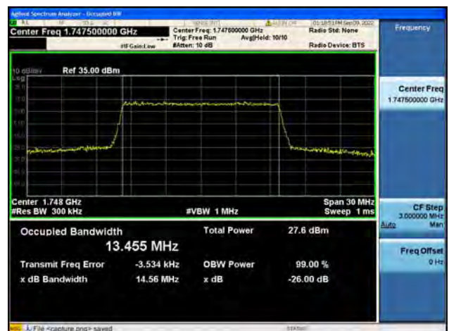
Band4 / 15MHz / 16QAM/ High CH
