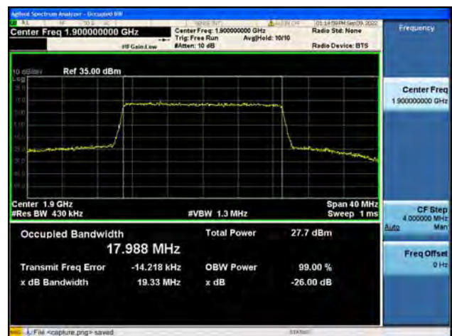
Band2 / 20MHz / 16QAM/ High CH
