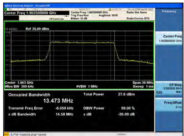
Band2 / 15MHz / 16QAM/ High CH
