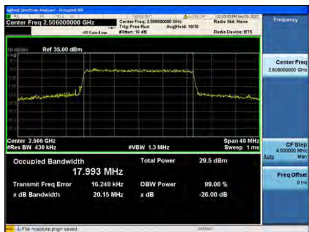
Band41 / 20MHz / QPSK/ Mid CH
