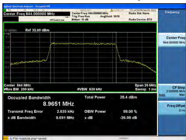
Band5 / 10MHz / 16QAM/ High CH
