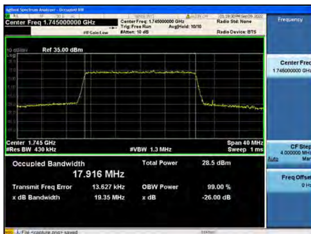
Band4 / 20MHz / QPSK/ High CH
