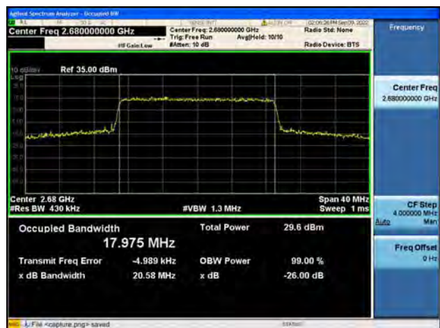
Band41 / 20MHz / QPSK/ High CH
