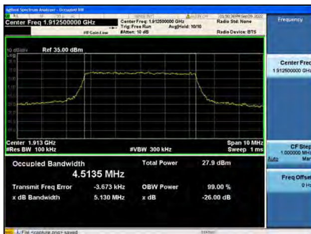
Band25 / 5MHz / QPSK/ High CH
