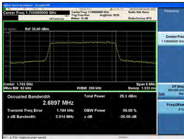
Band66 / 3MHz / QPSK/ High CH
