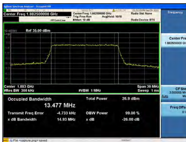
Band25 / 15MHz / 16QAM/ High CH
