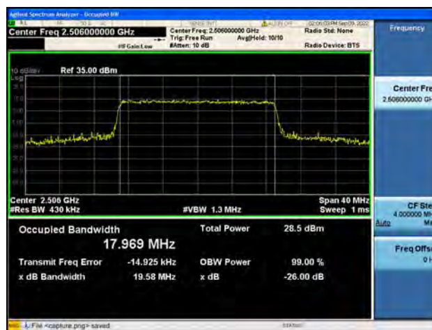
Band41 / 20MHz / 16QAM/ Mid CH
