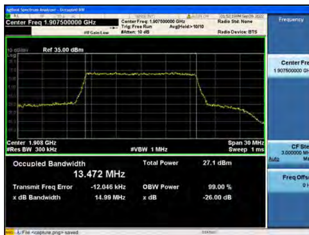
Band25 / 15MHz / 16QAM/ High CH
