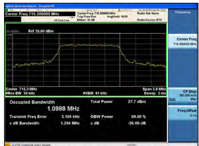
Band12 / 1.4MHz / 16QAM/ High CH
