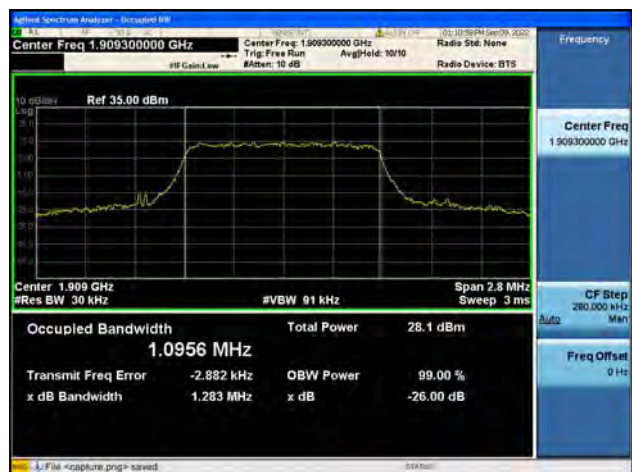
Band2 / 1.4MHz / QPSK/ High CH
