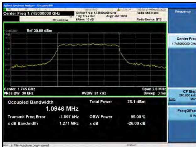
Band66 / 1.4MHz / QPSK/ High CH
