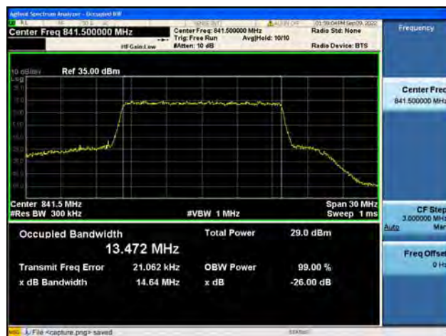
Band26Part22 / 15MHz / QPSK/ High CH
