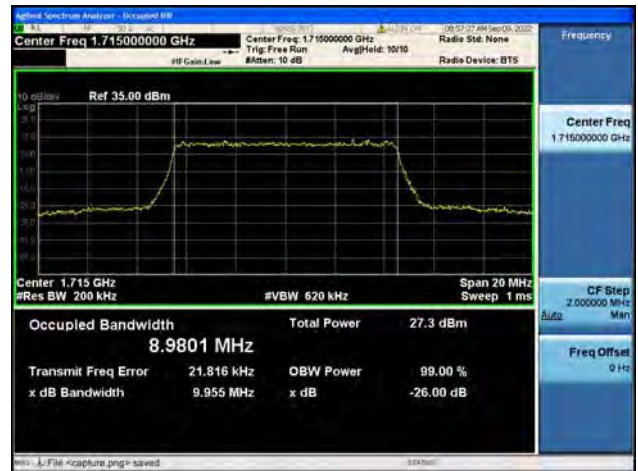
Band66 / 10MHz / 16QAM/ Mid CH
