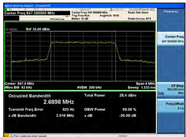
Band5 / 3MHz / 16QAM/ High CH
