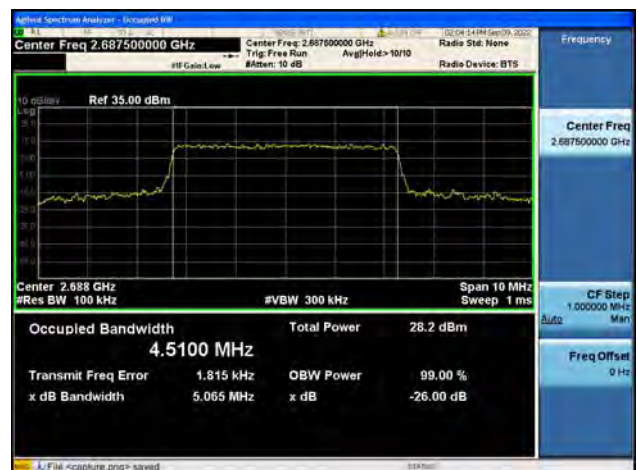
Band41 / 5MHz / 16QAM/ High CH
