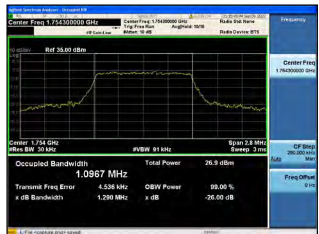
Band4 / 1.4MHz / 16QAM/ High CH
