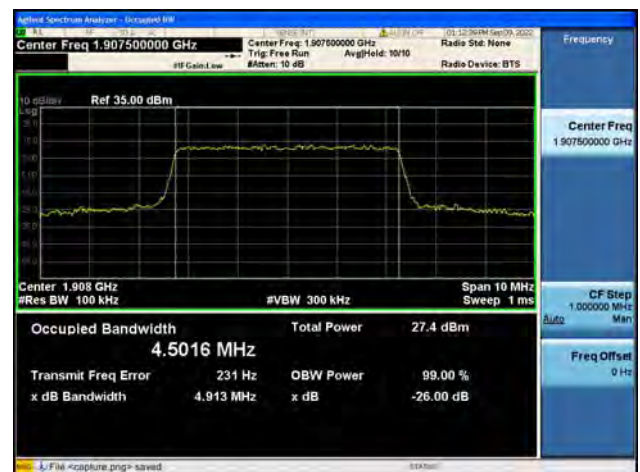
Band2 / 5MHz / 16QAM/ High CH
