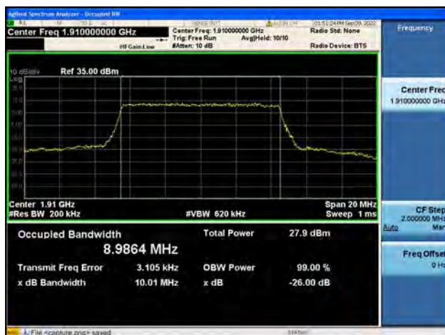
Band25 / 10MHz / QPSK/ High CH
