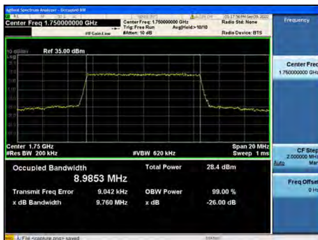
Band4 / 10MHz / QPSK/ High CH
