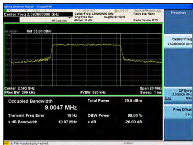
Band41 / 10MHz / QPSK/ High CH
