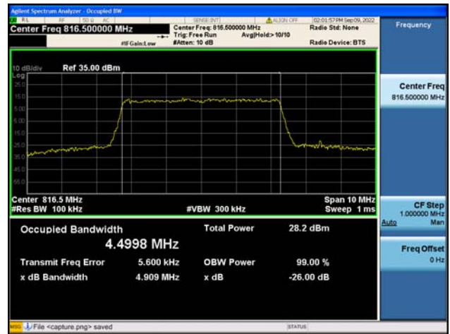
Band26Part90 / 5MHz / Mid CH / 16QAM
