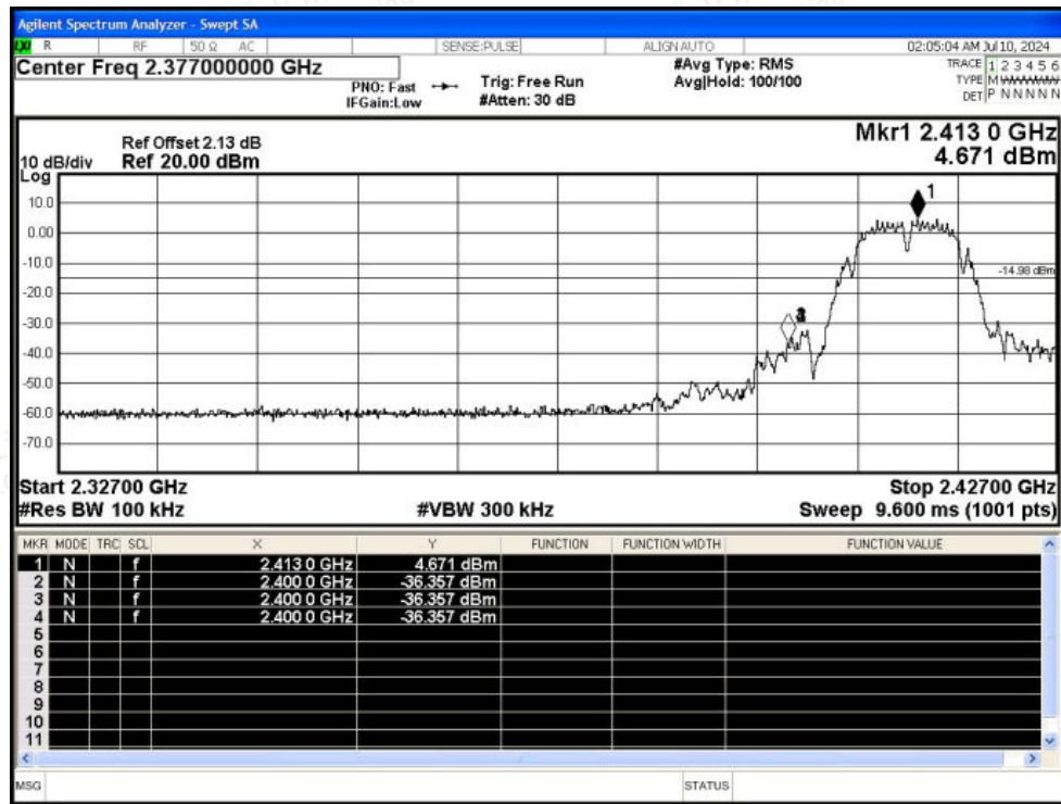
Band Edge NVNT b 2412MHz Ant1 Emission
