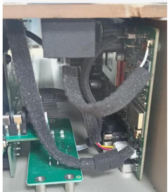
WiFi同轴线摆放。如图 WiFi coaxial cable placement. As shown in the figure.
