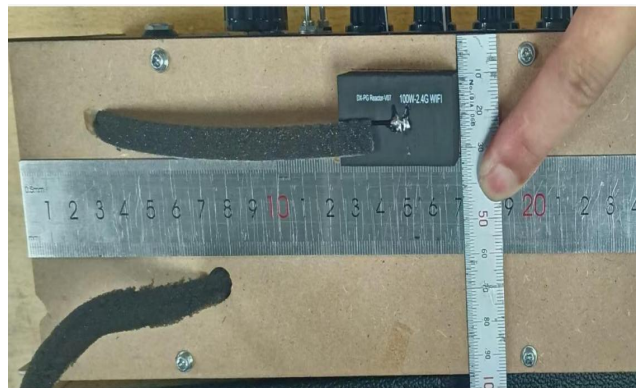
天线贴在木板外面，如图 The antenna is attached to the outside of the wooden board. As shown in the figure.
