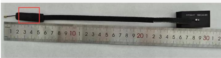
红色方框位置为磁环位置。如图 The red box indicates the position of the magnetic ring. As shown in the figure.
