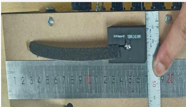
天线贴在木板外面，距边缘约 10MM.如图 The antenna is attached to the outside of the board, about 10mm from the edge, as shown in the figure
