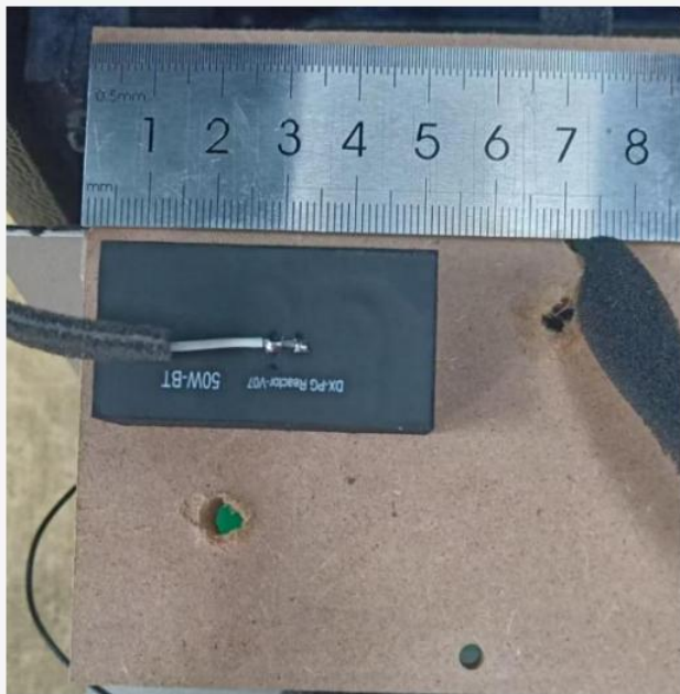
天线贴在木板内面，距边缘约 5MM.如图 The antenna is attached to the inner side of the board, about 5MM from the edge, as shown in the figure
