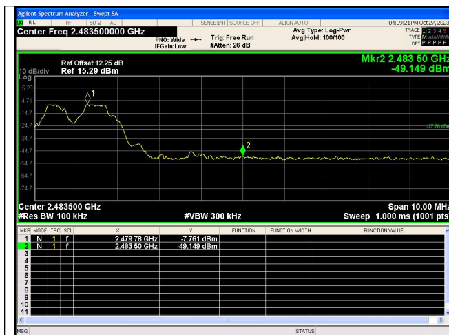
Out Of Band Emission(Right) GFSK_DH5_Channel Hopping
