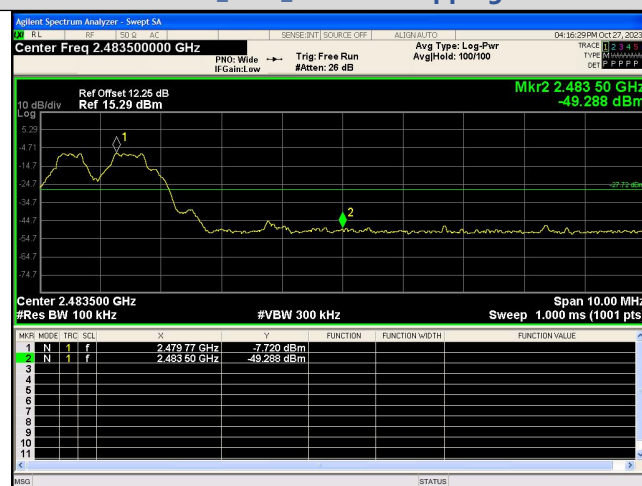
Out Of Band Emission(Right) GFSK_DH5_Channel Hopping
