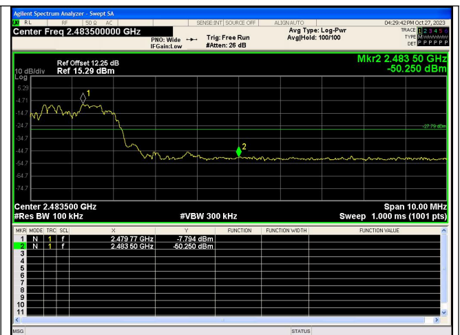
Out Of Band Emission(Right) \pi/4 DQPSK_2-DH5_Channel Hopping
