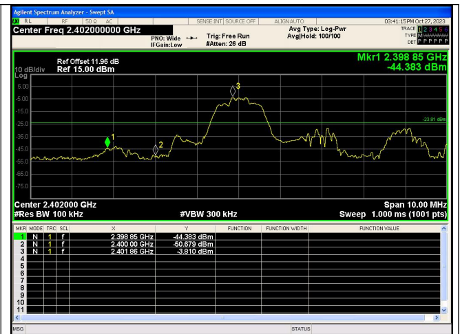
Out Of Band Emission \pi/4 DQPSK_2-DH5_Channel 0
