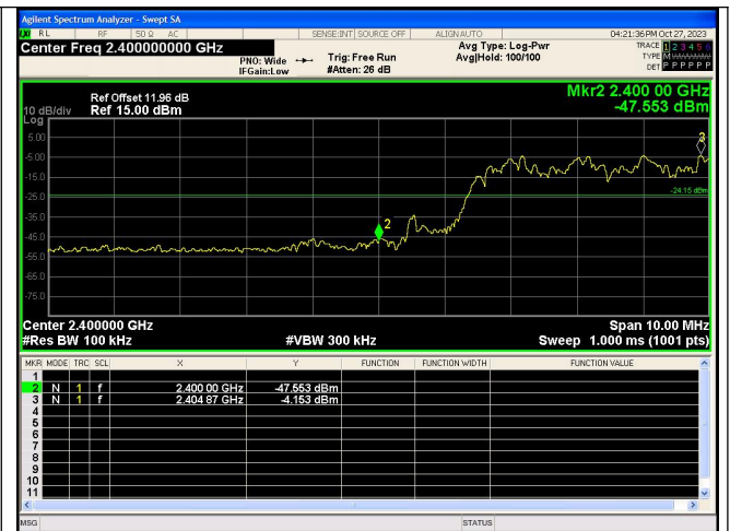
Out Of Band Emission(Left) \pi/4 DQPSK_2-DH5_Channel Hopping
