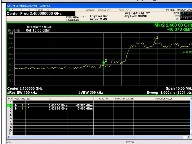
Out Of Band Emission(Left) 8DPSK_3-DH5_Channel Hopping
