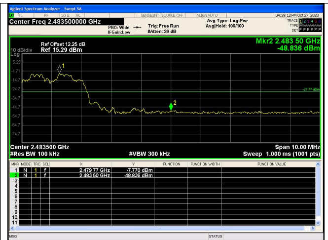
Out Of Band Emission(Right) 8DPSK_3-DH5_Channel Hopping
