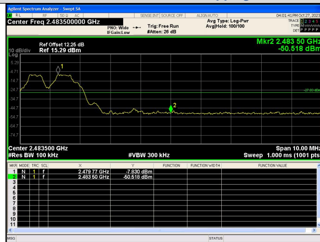
Out Of Band Emission(Right) GFSK_DH5_Channel Hopping
