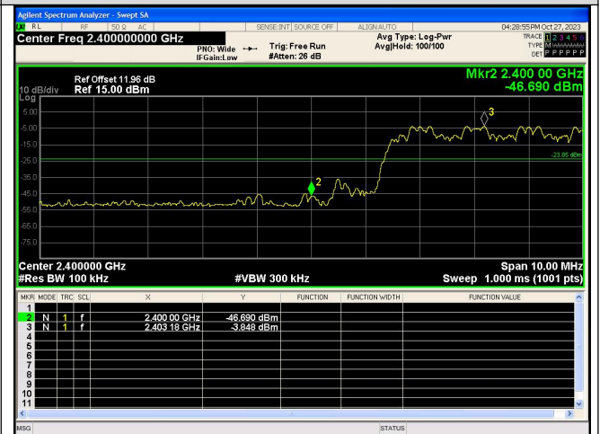
Out Of Band Emission(Left) \pi/4 DQPSK_2-DH5_Channel Hopping
