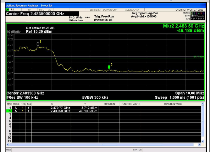
Out Of Band Emission(Right) \pi/4 DQPSK_2-DH5_Channel Hopping
