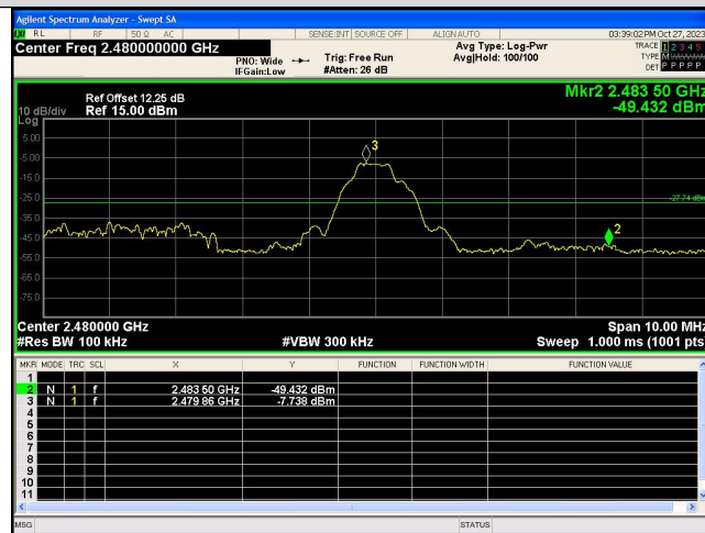
Out Of Band Emission GFSK_DH5_Channel 78
