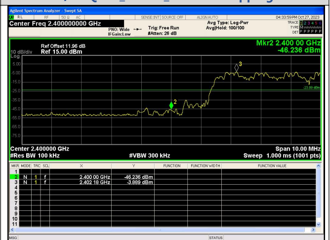
Out Of Band Emission(Left) \pi/4 DQPSK_2-DH5_Channel Hopping
