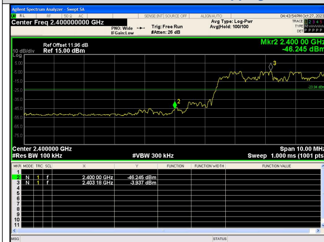
Out Of Band Emission(Left) 8DPSK_3-DH5_Channel Hopping
