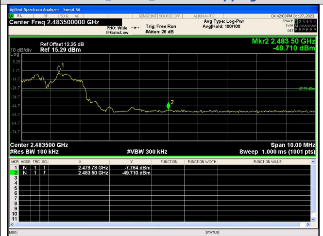
Out Of Band Emission(Right) 8DPSK_3-DH5_Channel Hopping
