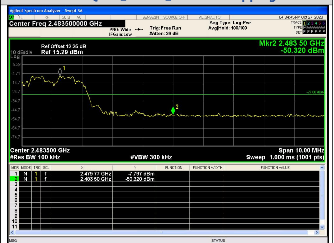
Out Of Band Emission(Right) \pi/4 DQPSK_2-DH5_Channel Hopping
